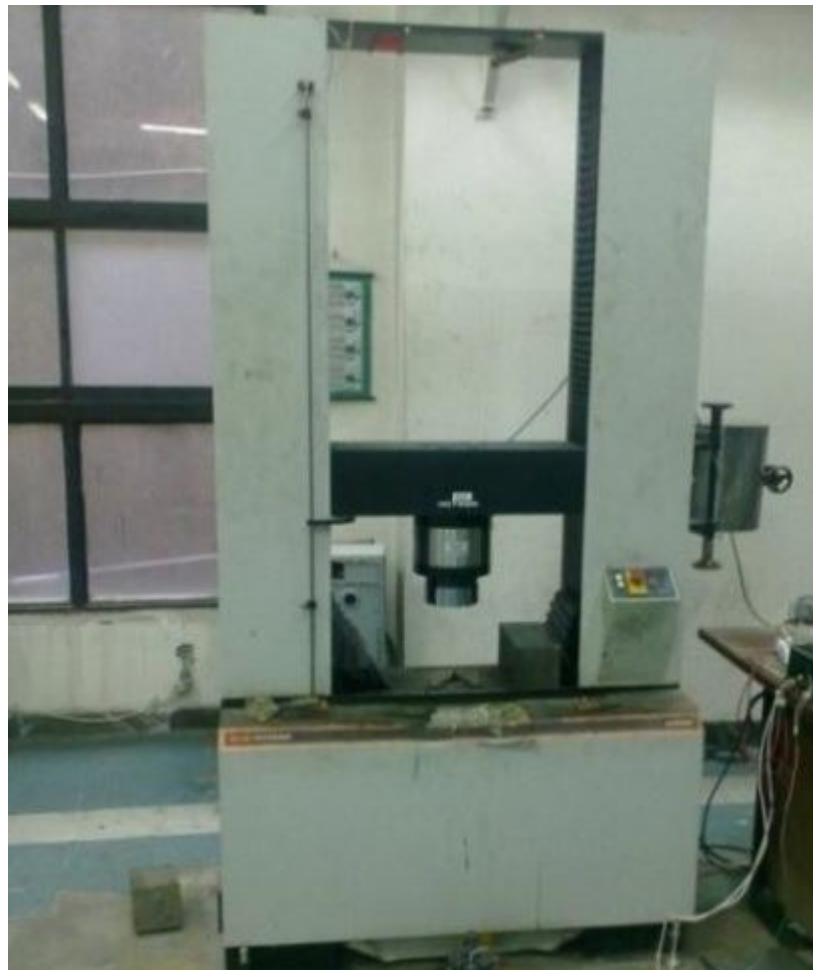
Figure 3.3 schematic of instron a tensile testing machine, Model 4208
