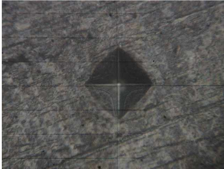
Figure 3.11 micro-hardness test of 1 pass sample
