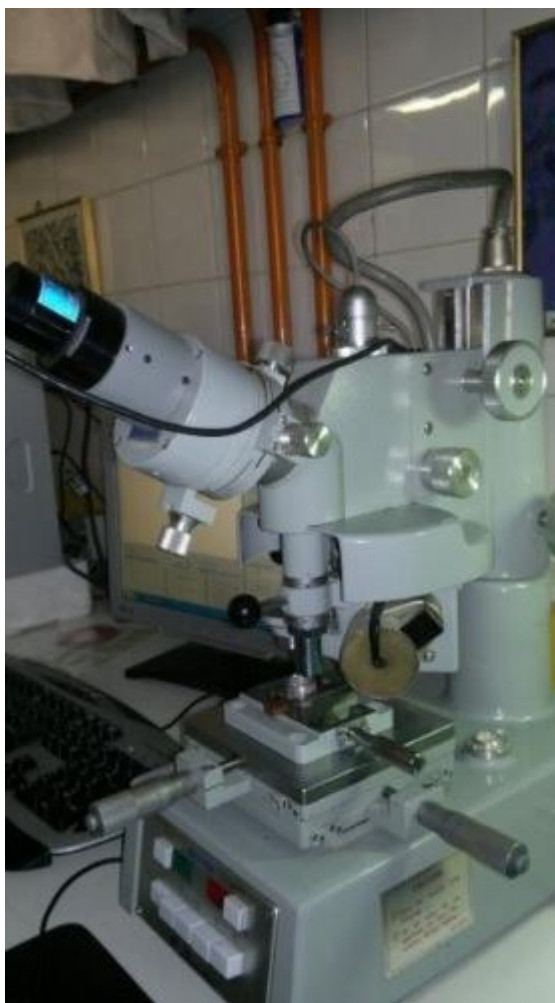
Figure 3.10 Shimadzu Micro-hardness test machine
