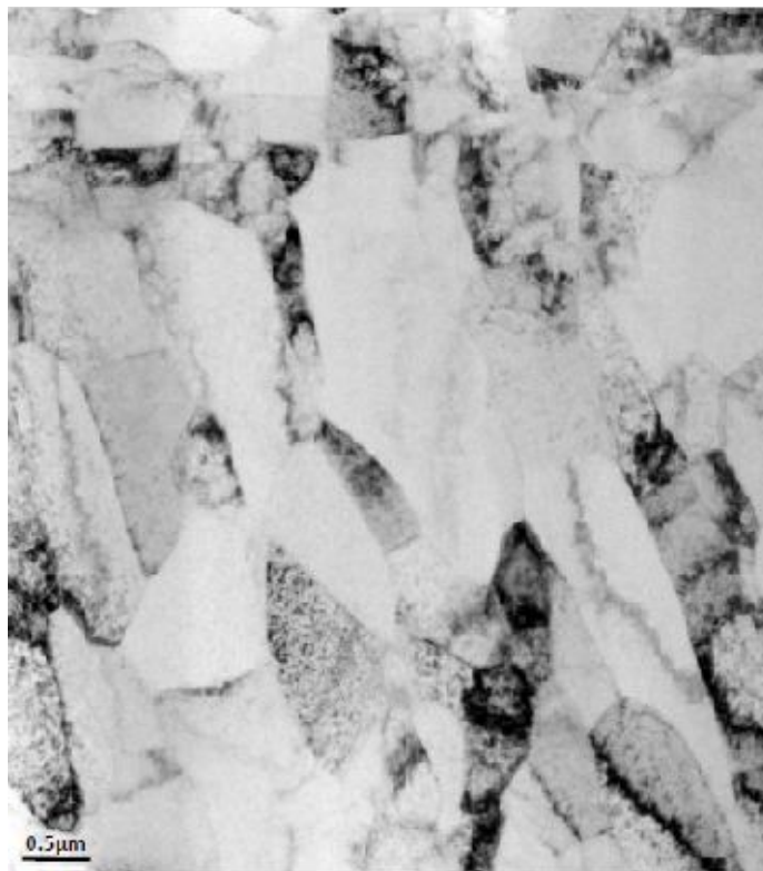
Figure 4.11 Bright field TEM micrographs of the cross-sectional microstructure of the TCAP processed tube after (a) one, (b) two and (c) three passes.
