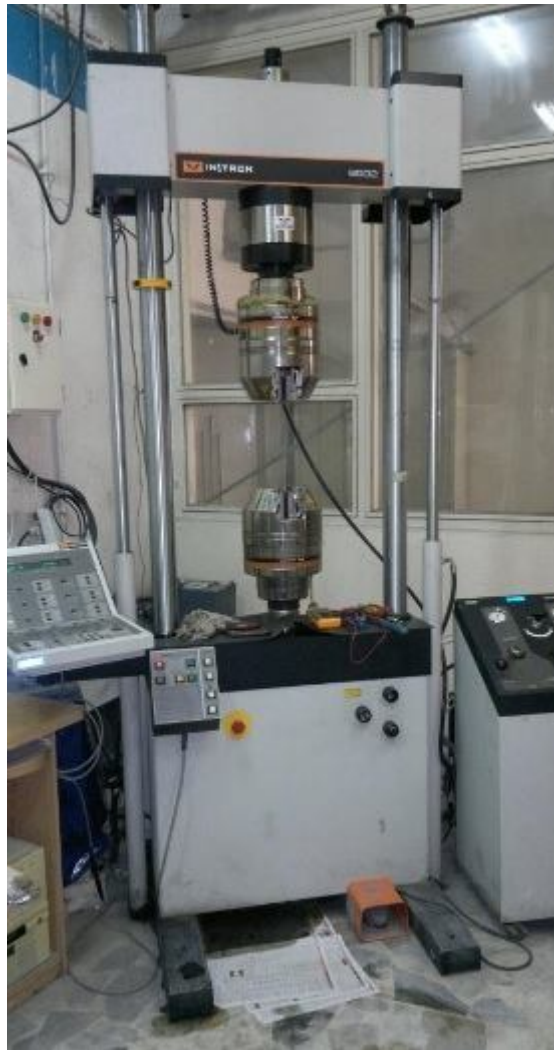
Figure 3.13 Tension Testing Machine model 8502
