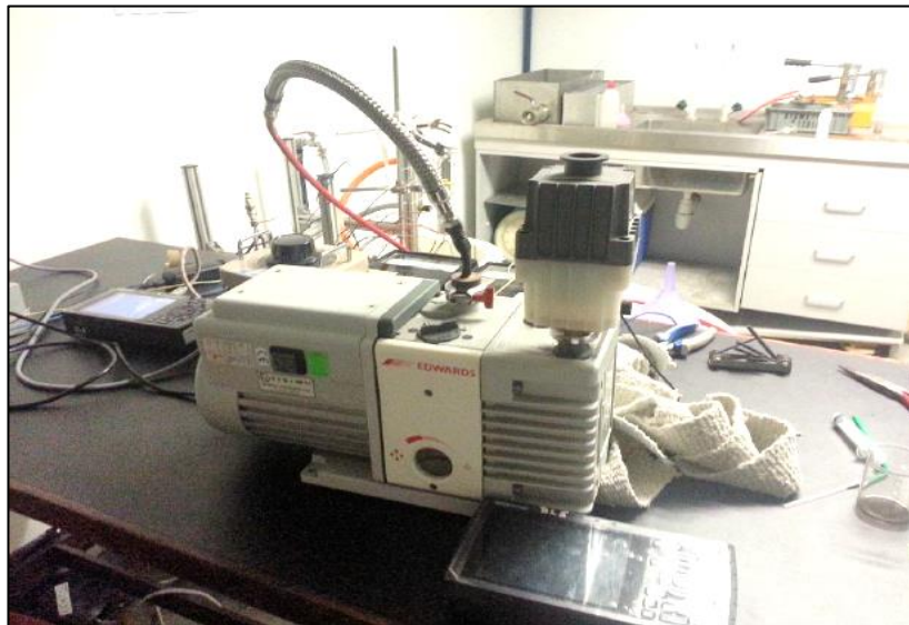
Figure 3.13: Vacuum pump used to achieve the negative pressure inside the pump
