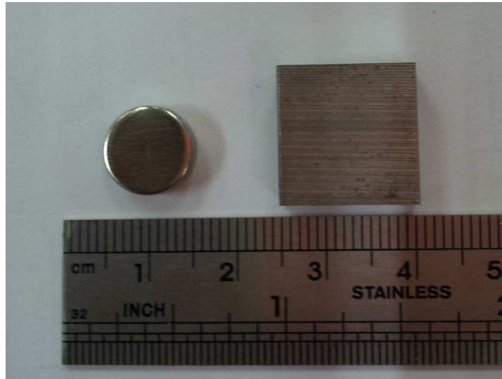
Figure 3.2: Substrates used in the analysis (a) On the left SS and; (b) On the right HSS.
