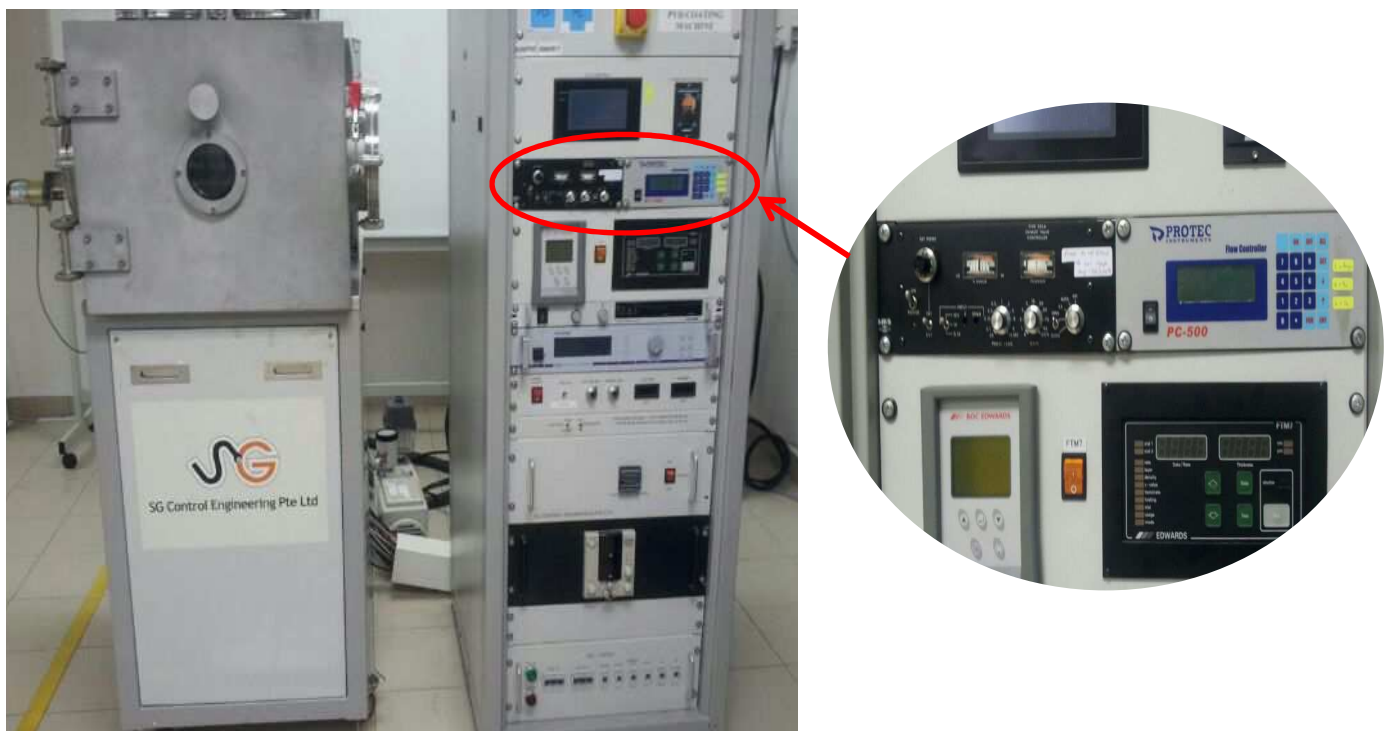
Figure 3.5: TF450 PVD magnetron sputtering system (SG Control Engineering PTE LTD, Singapore) equipped with Protec Instruments PC-500 Flow Controller (enlarge picture).
