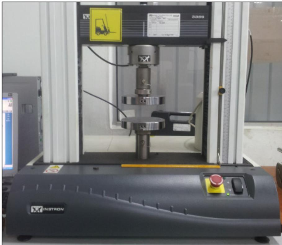
Figure 3.10: INSTRON 3369 Testing Machine
