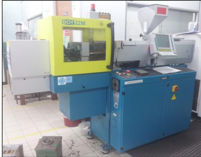
Figure 3.8: Plastic Injection Molding Machine
