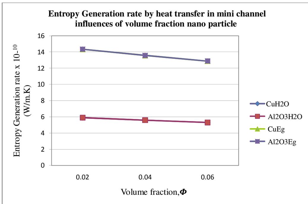
Figure 4.8 - Entropy generation rate by heat transfer in mini channel influences of volume fraction nano particle
