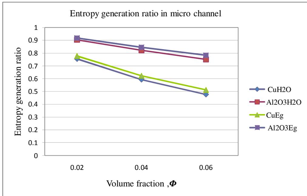
Figure 4.5- Graph of entropy generation ratio in micro channel.
