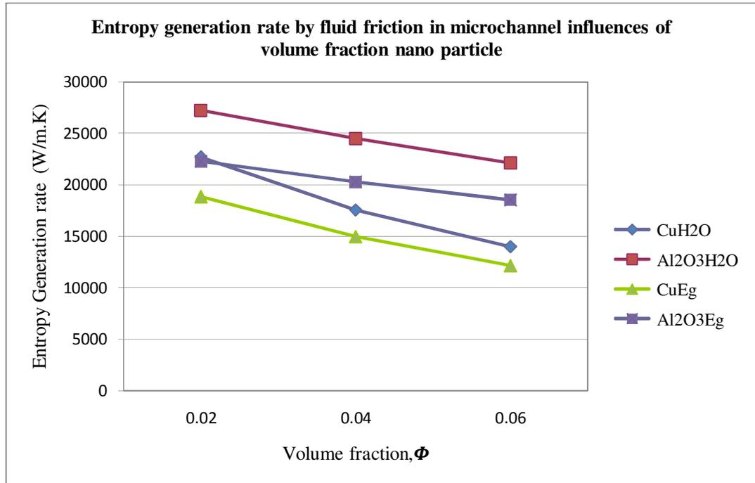
Figure 4.11 - Entropy generation rate by fluid friction in micro channel influences of volume fraction nano particle
