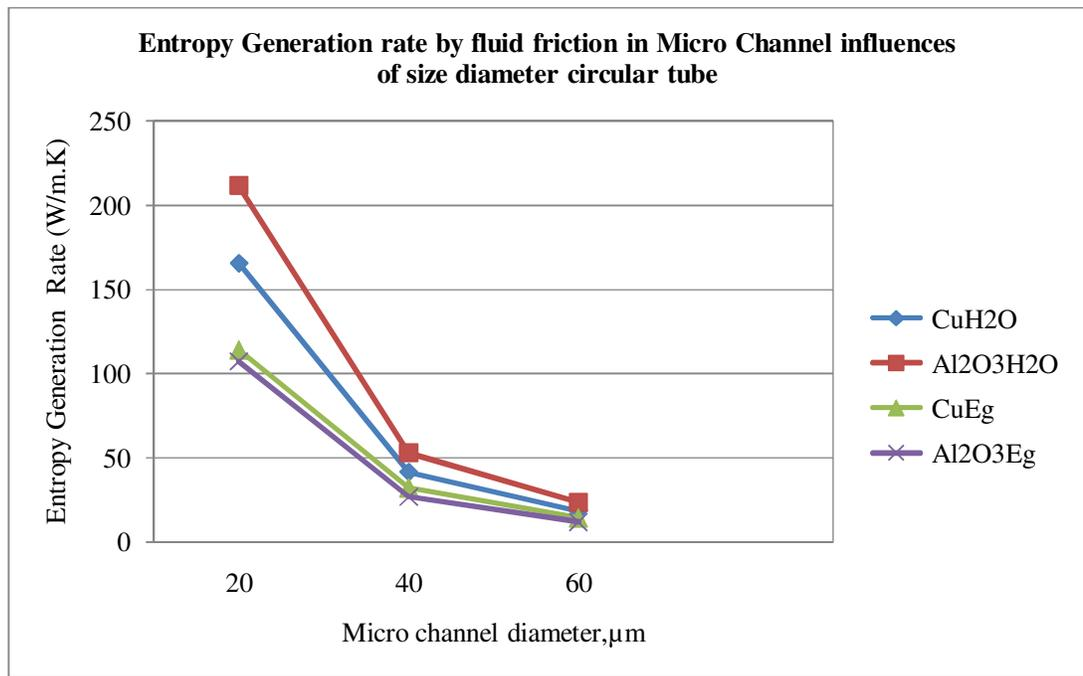
Figure 4.13- Entropy generation rate by fluid friction in micro channel influences of size diameter circular tube
