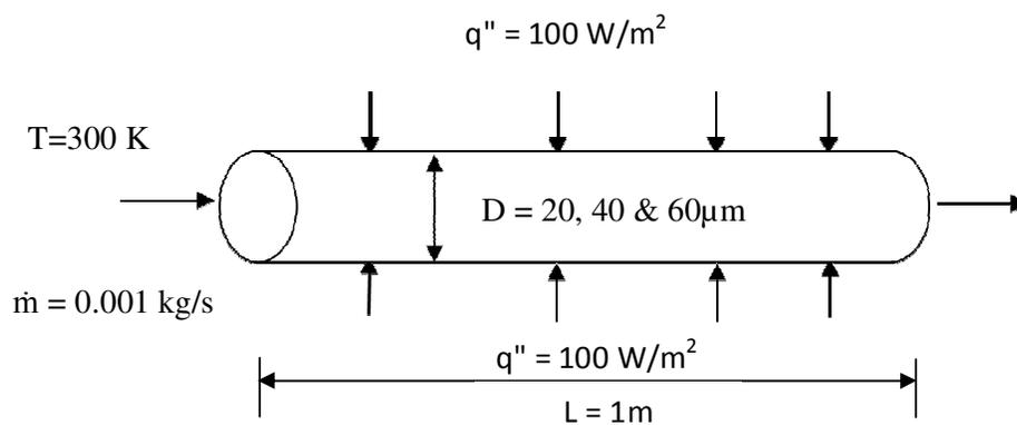
Figure 3.1 - Circular micro channel of constant cross section
