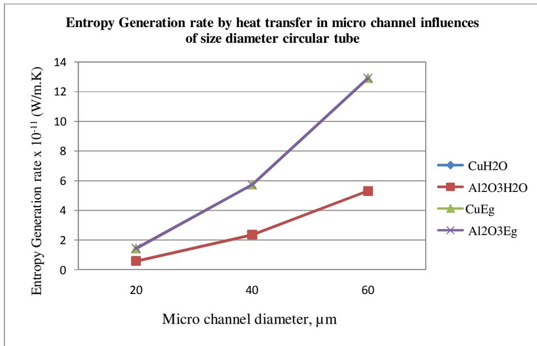
Figure 4.9 - Entropy generation rate by heat transfer in micro channel influences of size diameter circular tube
