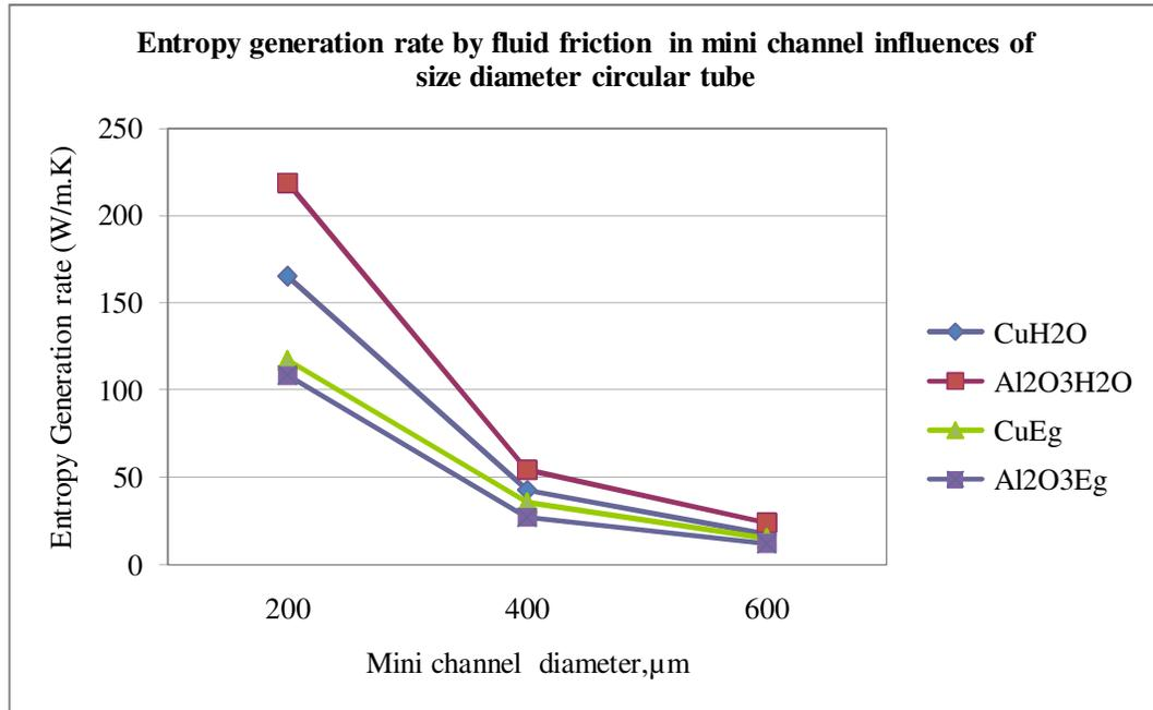
Figure 4.14 - Entropy generation rate by fluid friction in mini channel influences of size diameter circular tube
