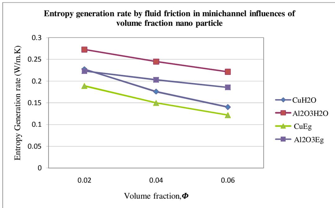
Figure 4.12 - Entropy generation rate by fluid friction in mini channel influences of volume fraction nano particle
