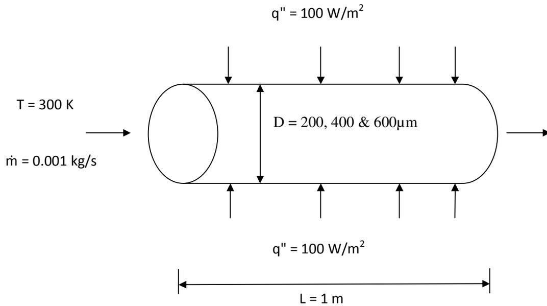
Figure 3.2 - Circular mini channel of constant cross section
