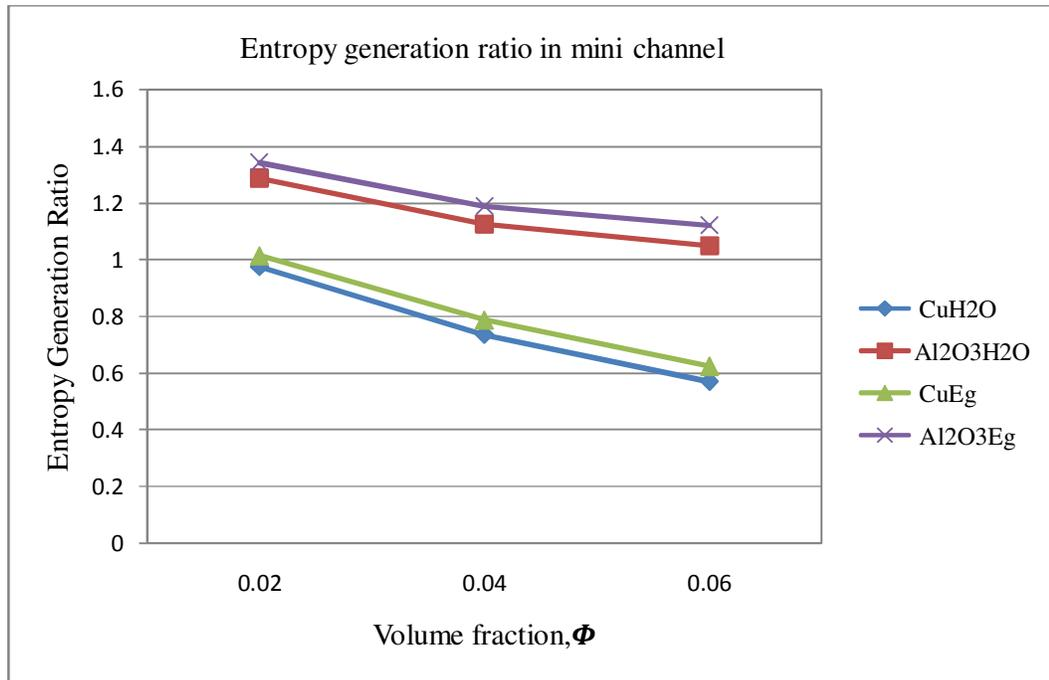
Figure 4.6- Graph of entropy generation ratio in mini channel
