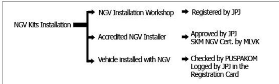
Figure 6: Natural Gas Installation Procedure Flowchart
