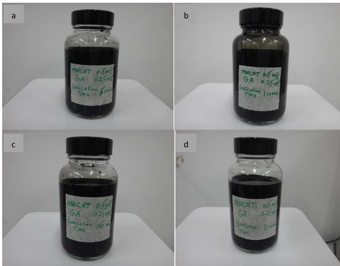
Figure 3.6 Vials including 0.5 wt % of MWCNT` s disspered in distilled water after 2 weeks and different ultrasonication times: (a) 50 minutes; (b) 100 minutes; (c) 150 minutes; (d) 200 minutes.
