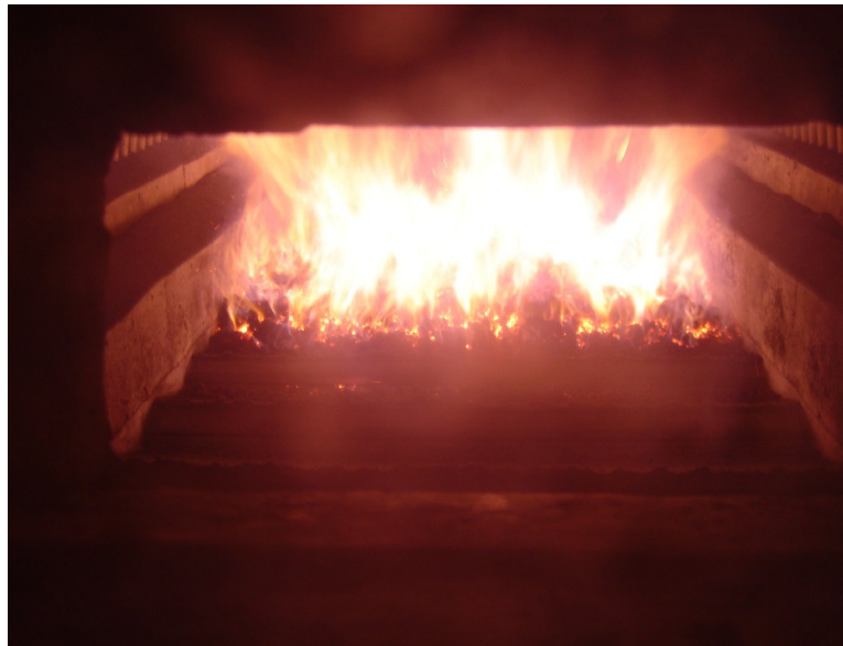
Figure 5.3: Reciprocating grate during Combustion
