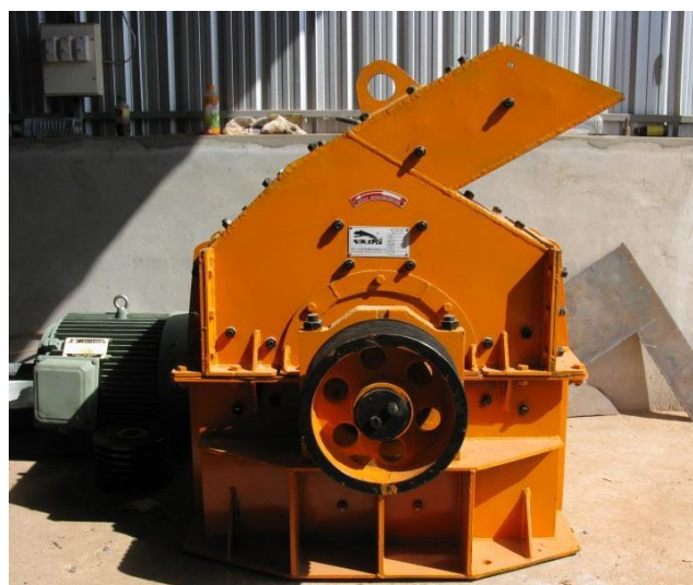
Figure 3.9 Horizontal hammer crushing machine
