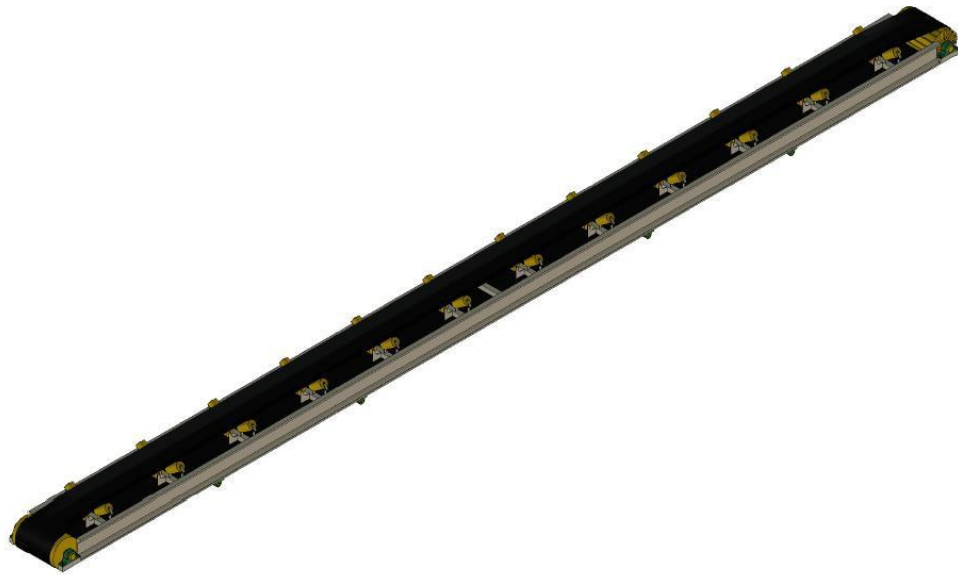
Figure 4.7 Troughed conveyor belt design.
