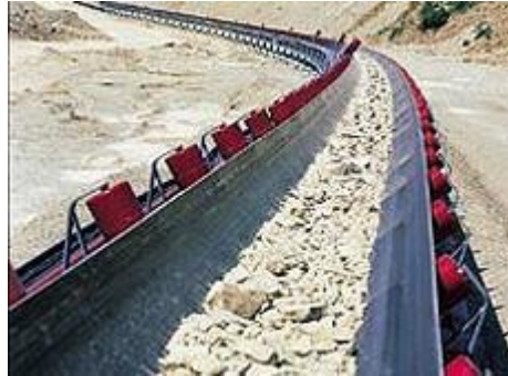
Figure 2.1 Troughed conveyor belt
