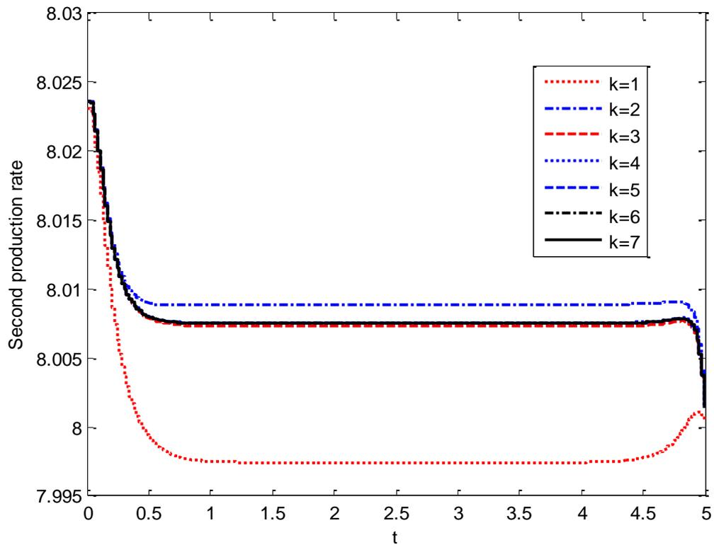
**Figure 6.12: Second production rate against time  $t_f = 5$  and  $m = 256$  of the application of the direct method using logistic demand rates for  $k = 1, 2, 3, 4, 5, 6, 7$  quasilinearization iterations**
