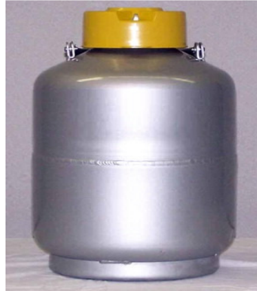
Figure 8.1 Typical cryogenic storage tanks for liquefied nitrogen gas (Jahan et al. , 2012).
