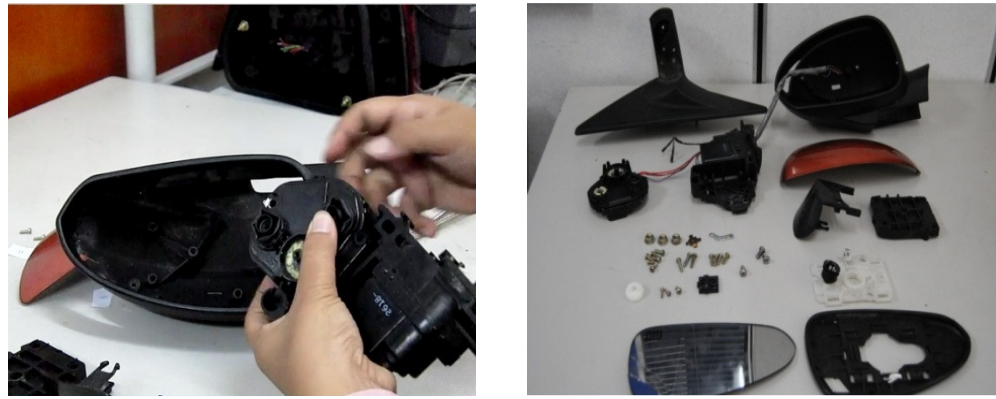
Figure 5.11 Manual disassembly of a car's side mirror.
