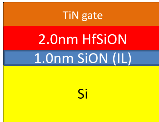
Fig. 4.14 Schematic illustration of the 2.0nm TiN/ HfO 2 / SiO 2 gate stack
