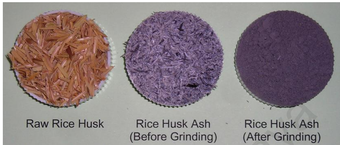
Figure 2.7: (a) Raw rice husk from Selangor, Malaysia (b) RHA before grinding (c) RHA after grinding (Raman et al., 2011)
