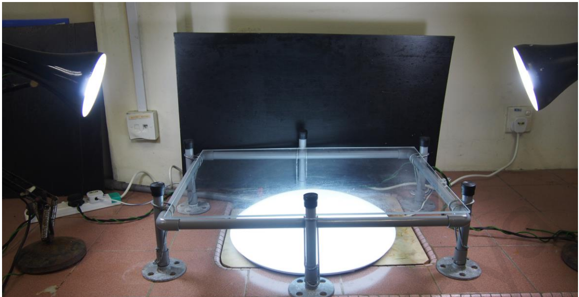
Figure 2.3: Dry photography setup showing the acrylic stage, with light source below and additional light sources at the sides.
