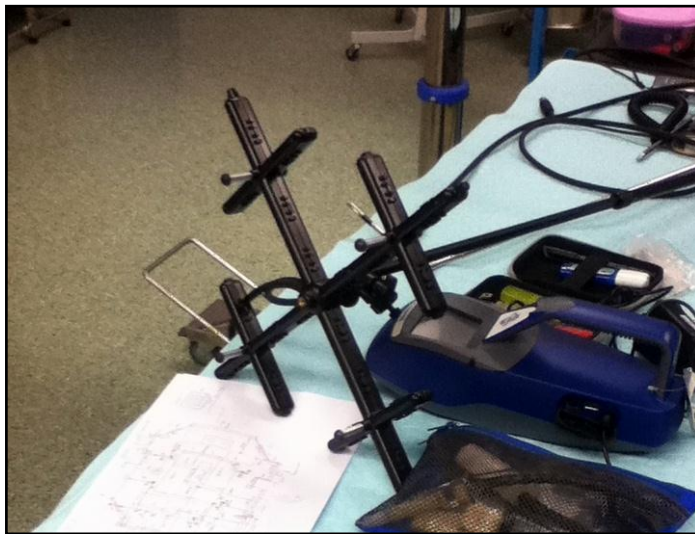
Figure 4.5: Velocity matrix available in Alnor EBT721 balometer.
