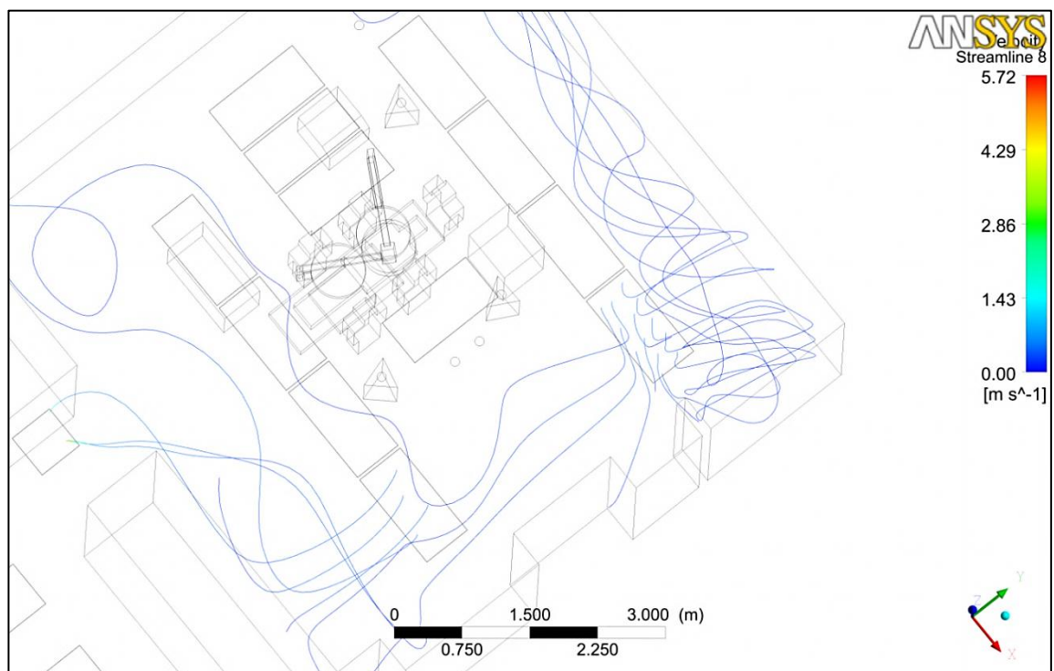
Figure 5.23: Streamlines for air discharged from inlet 4 and inlet 8.
