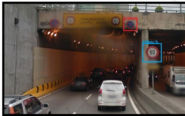
Figure 4.19: Successful detection 60km/h speed limit sign and no stopping sign
