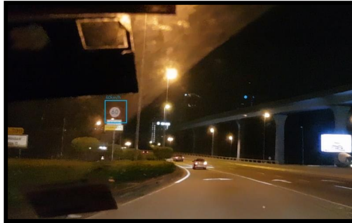
Figure 4.6: Successful detection of 60km/h speed limit sign at night
