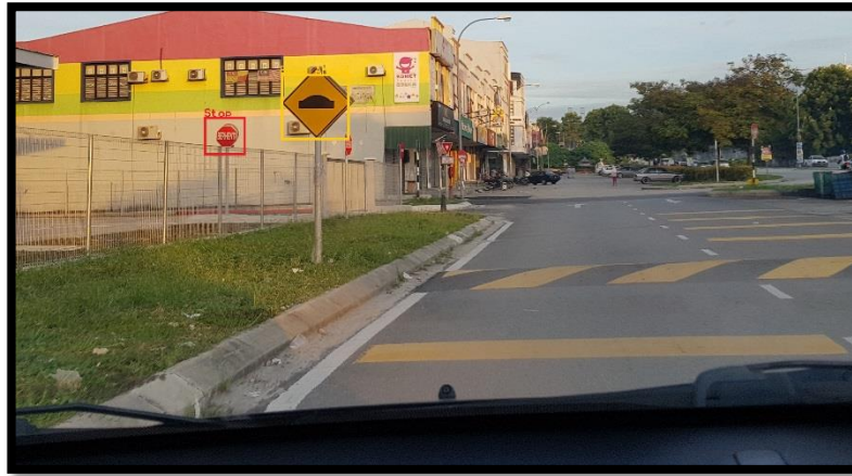
Figure 4.15: Successful detection of Bump Ahead and Stop sign
