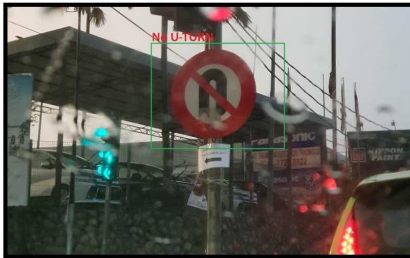
Figure 4.12: Successful detection of No U-turn sign in rainy day
