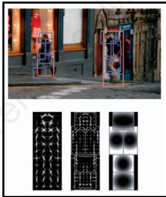
Figure 2.2: Detection of a single person and representation of single person in parts based models [18]
