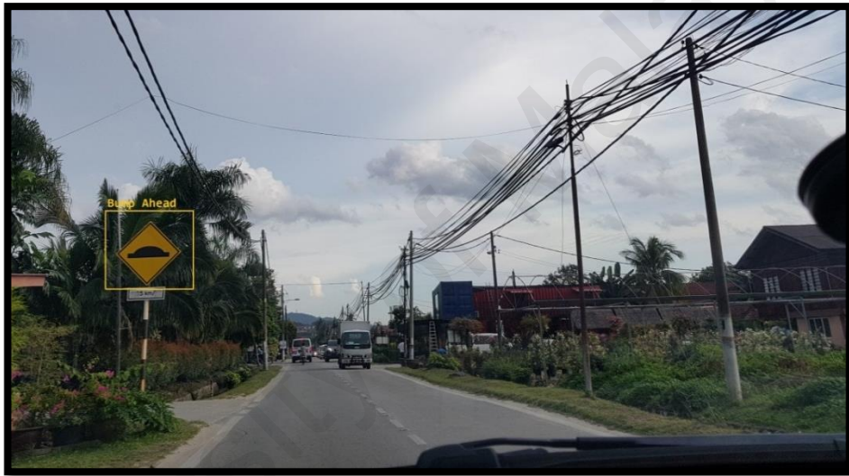
Figure 4.10: Successful detection of bump sign in day time
