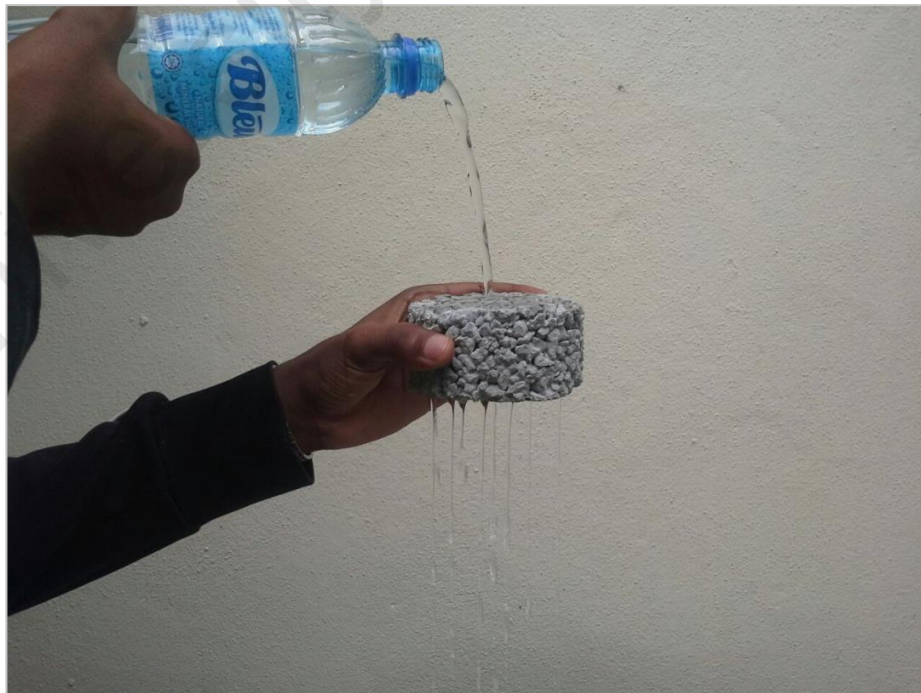
Figure 2.2: Water penetrating through the voids of a pervious concrete
