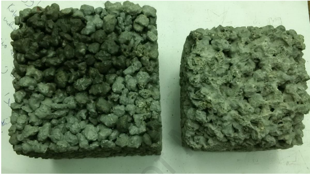
Figure 4.25: A typical POC pervious concrete specimen before (LHS) and after (RHS) abrasion resistance test
