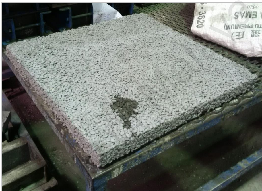
Figure 2.1: Pervious concrete slab
