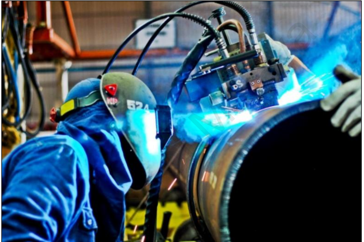
Figure 5.1 Welding fumes generated by automatic welding
