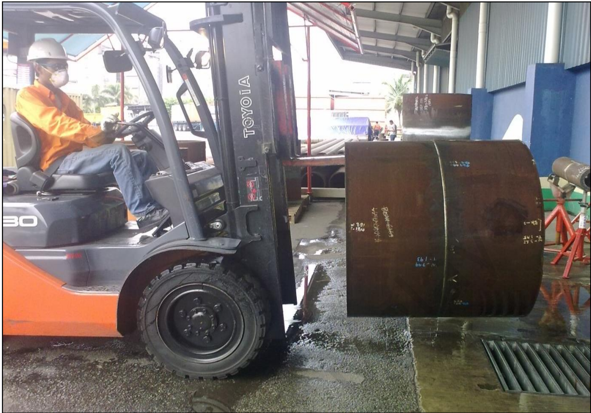
Figure 5.4 Competent forklift operator transferring a pipe joint
