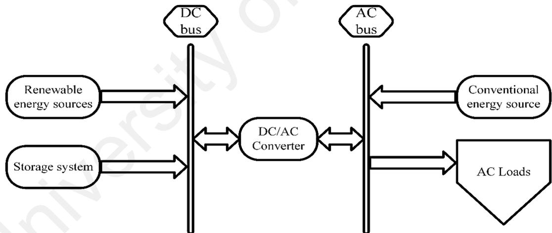
**Figure 1.1:** Simplified hybrid system block diagram
