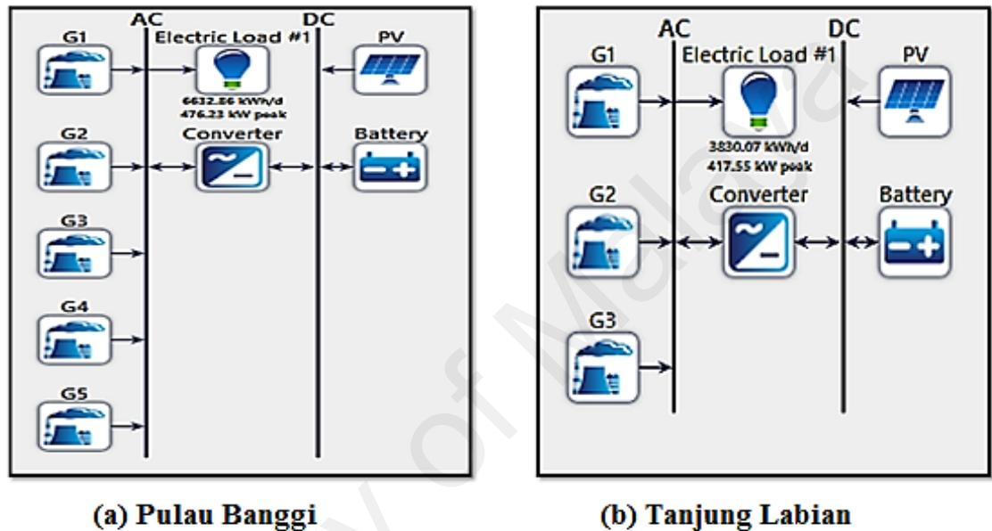
**Figure 4.1:** Existing hybrid system in both location implemented in HOMER (a) Pulau Banggi (b) Tanjung Labian
