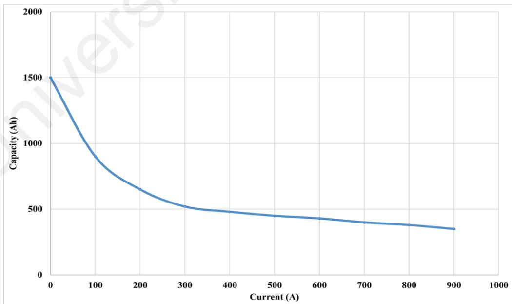
**Figure 3.7:** Batteries' capacity curve Capacity (Ah) VS discharge current (A)
