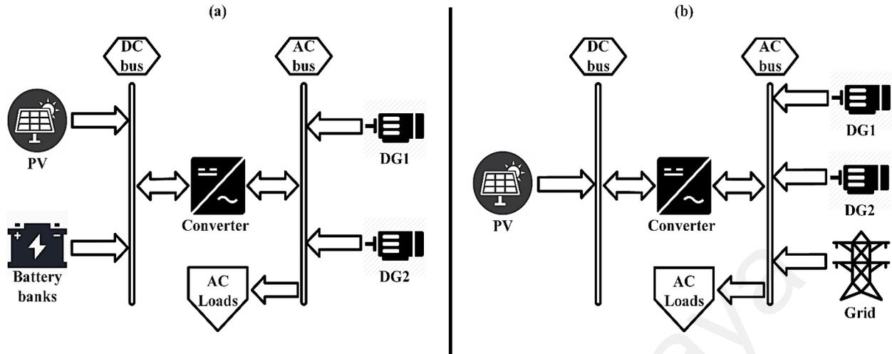
**Figure 4.14:** System components including all parts (a) Off-grid system (b) On-grid system
