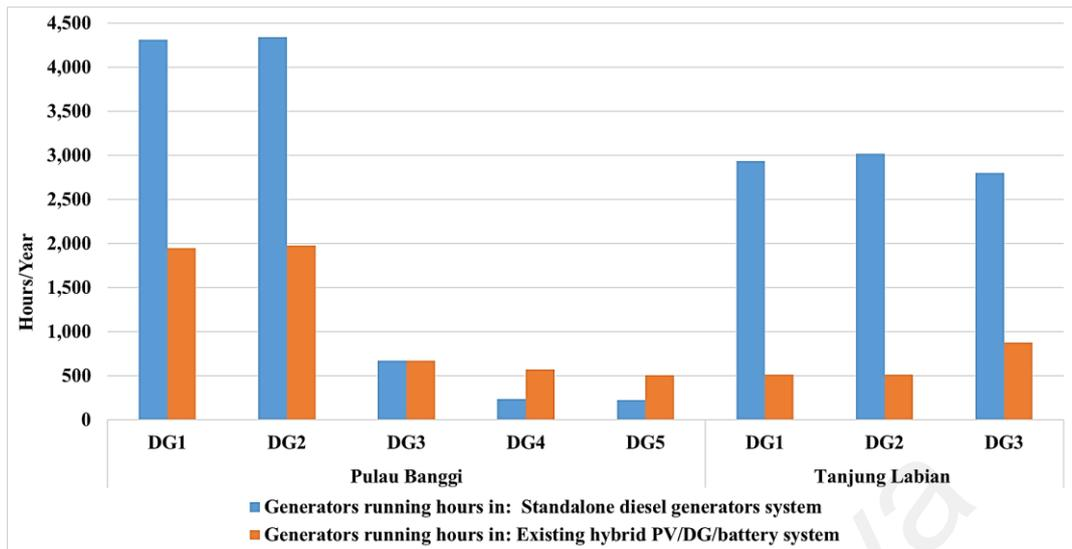
**Figure 4.8:** Pulau Banggi and Tanjung Labian generators running hours before and after adding PV/batteries
