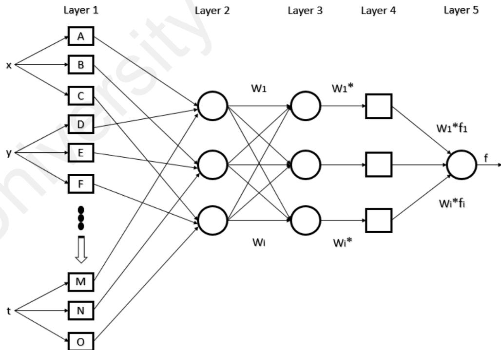
**Figure 3.11:** Five inputs, multiple rules and one output ANFIS structure
