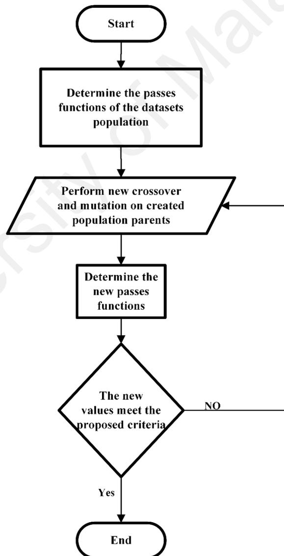
**Figure 3.13:** General description of GA work procedure flowchart
