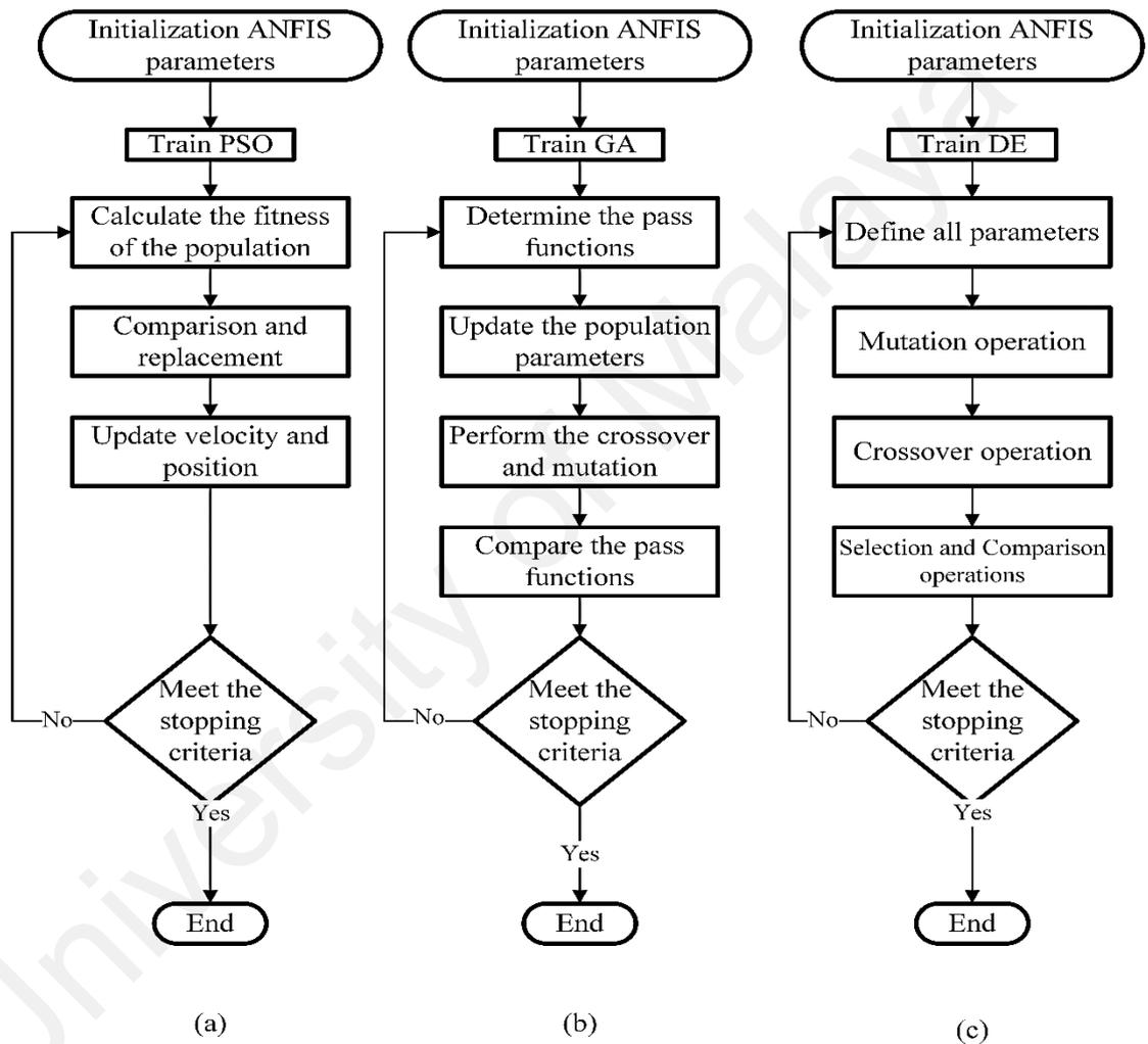
**Figure 3.10:** General simulation setup of all proposed models (a) ANFIS-PSO, (b) ANFIS-GA, and (c) ANFIS-DE
