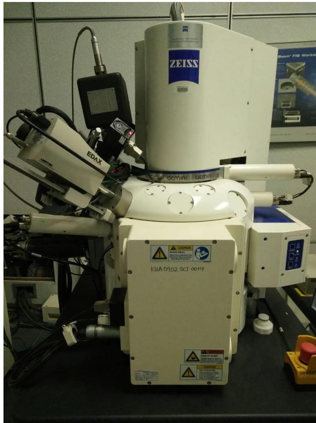
Figure 3.8: Field emission scanning electron microscope (FESEM)
