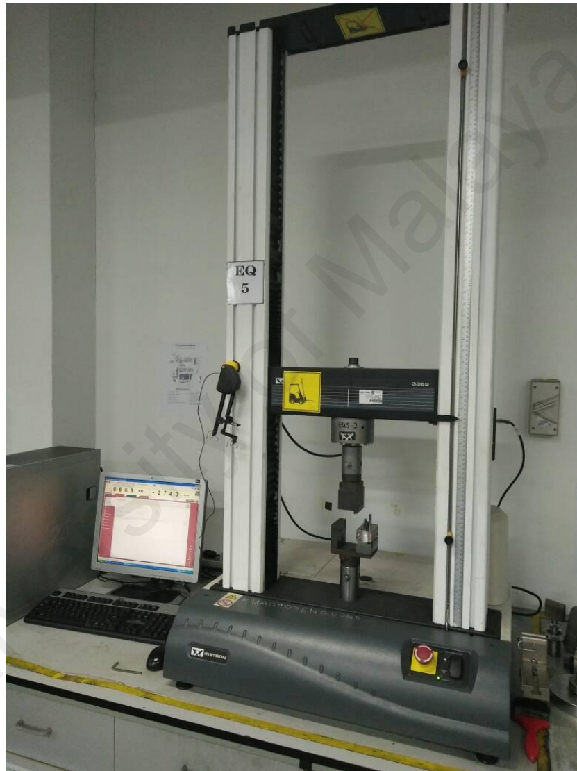
Figure 3.6: INSTRON universal testing machine
