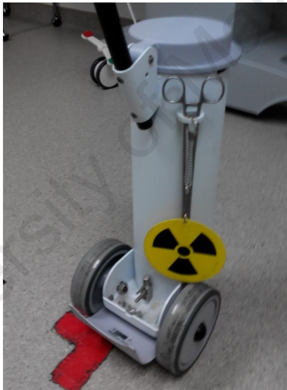
Figure 7: Emergency container with long pair of forceps
