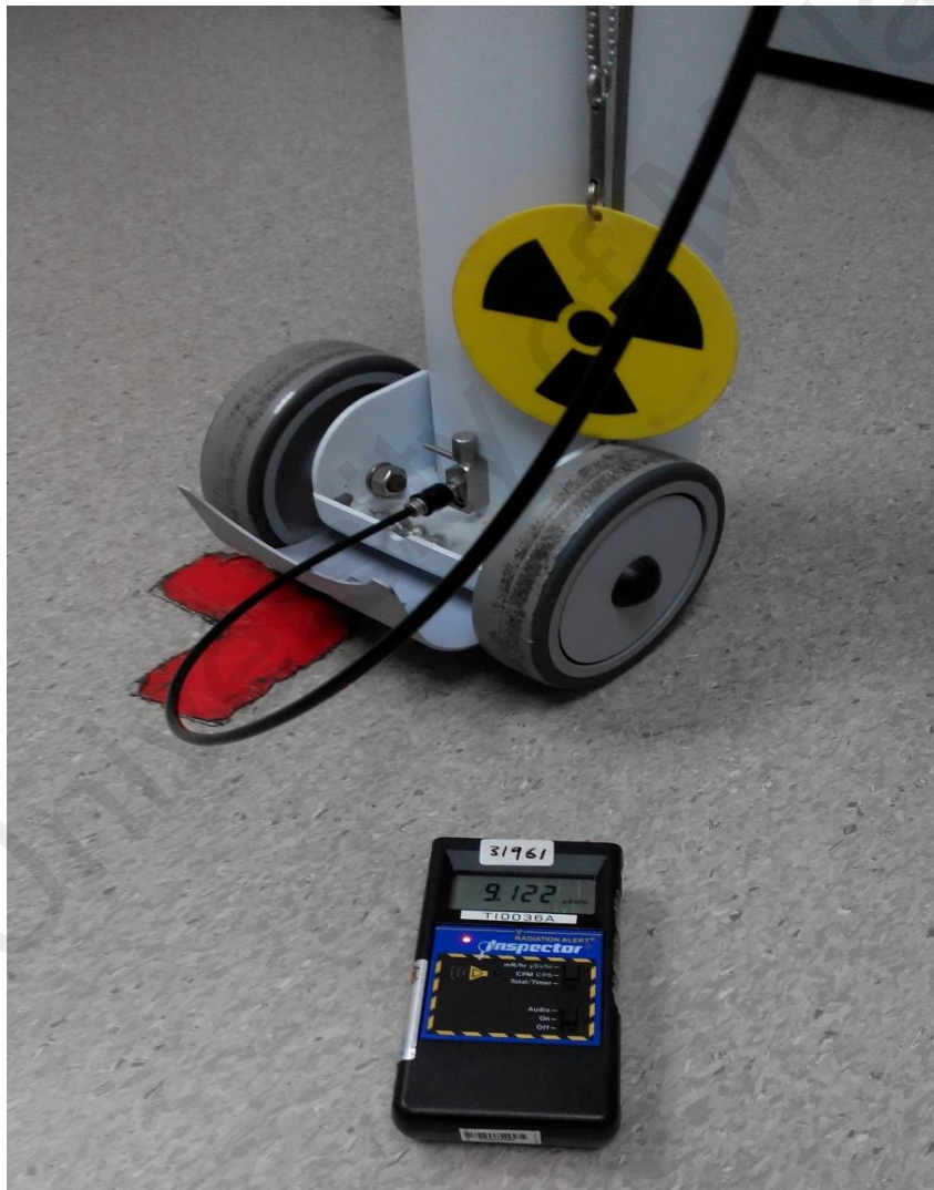
Figure 10: Source inside an emergency container.
