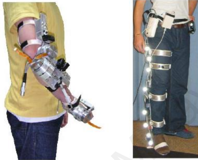
Figure 1.1 Upper and lower limb exoskeleton for rehabilitation robotics (Rocon et al., 2007)
