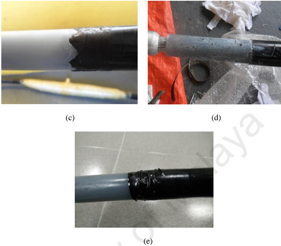
Figure 3.2: Defects created; (a) Defect of incision on insulation, (b) Defect of shift on axial direction, (c) Defect of tip on semiconductor layer, (d) Defect of XLPE metal particle and (e) Defect of air gap in semiconductor layer
