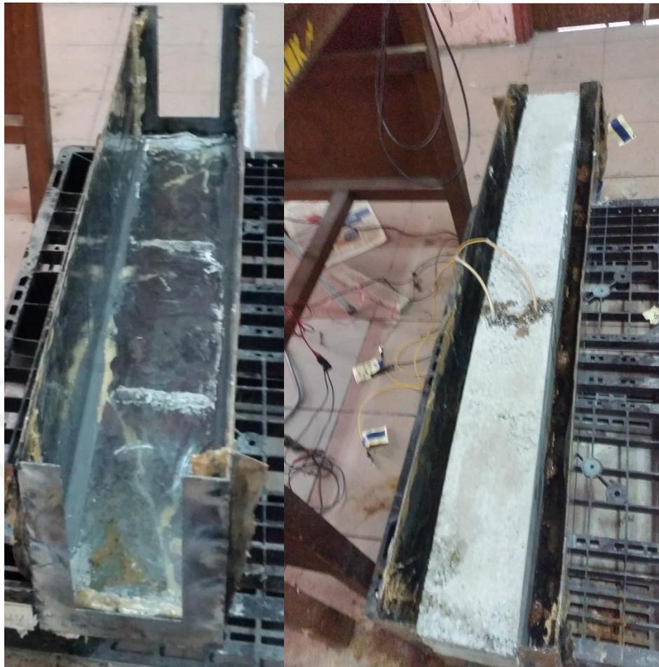
Figure 3.14: Steel container used for accelerated corrosion of beam specimens.
