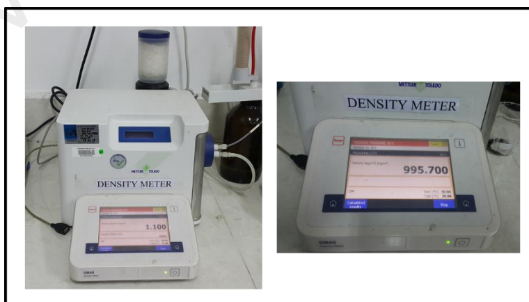
Figure 3. 15: DE-40 density meter, Mettler Toledo
