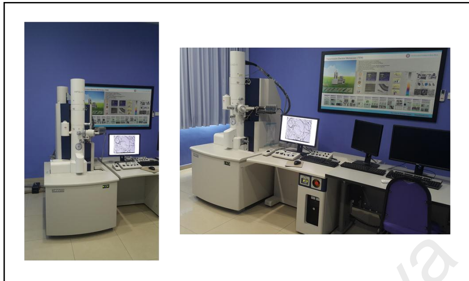
Figure 3. 10: Hitachi HT7700 transmission electron microscope
