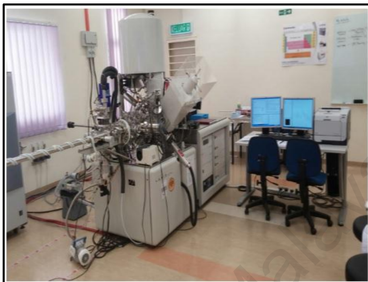
Figure 3. 9: Axis Ultra-DLD system, Kratos Analytical X-ray photoemission spectrometer (XPS)
