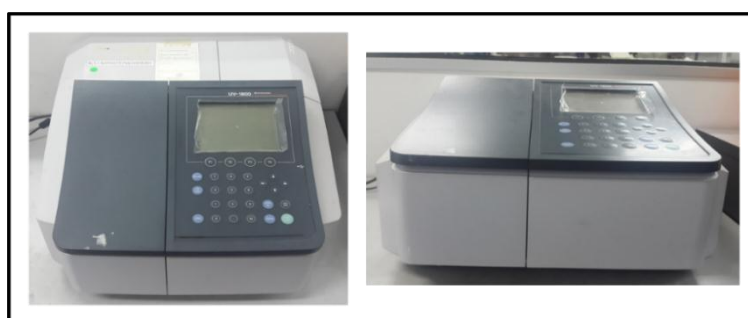
Figure 3. 12: Shimadzu UV-1800 spectrophotometer
