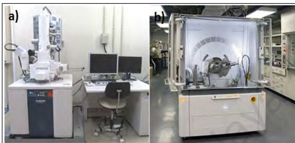
Figure 3.5: Instruments used for FESEM (a), and XRD analysis (b).
