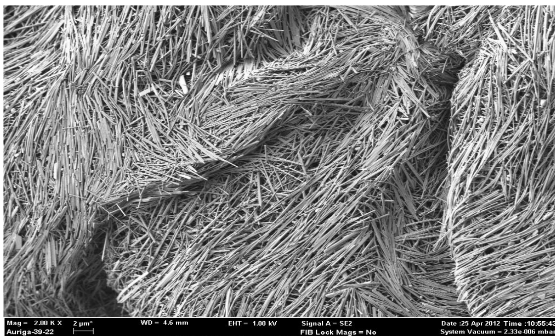
Figure 4.16: FESEM image of as-synthesized sample with \text{CuCl}_2 mediated agent at 2000X magnification.
