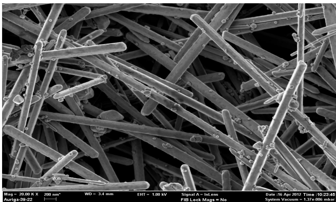
Figure 4.4: FESEM image of as-synthesized sample which has PVP: AgNO 3 molar ratio of 7.5:1 and 10 minutes of injection time.
