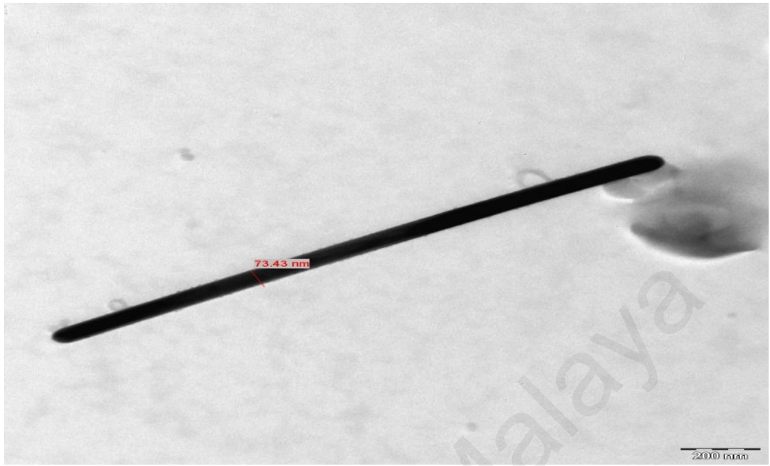
Figure 4.41: TEM image for as-synthesized sample with control agents of KCl.
