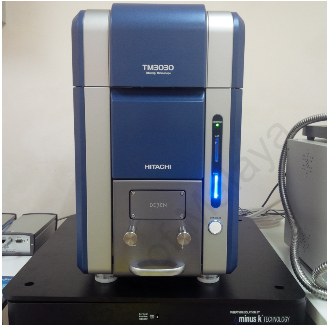
Figure C.14. The table-top scanning electron microscope machine used to evaluate the surface topology and phase composition.
