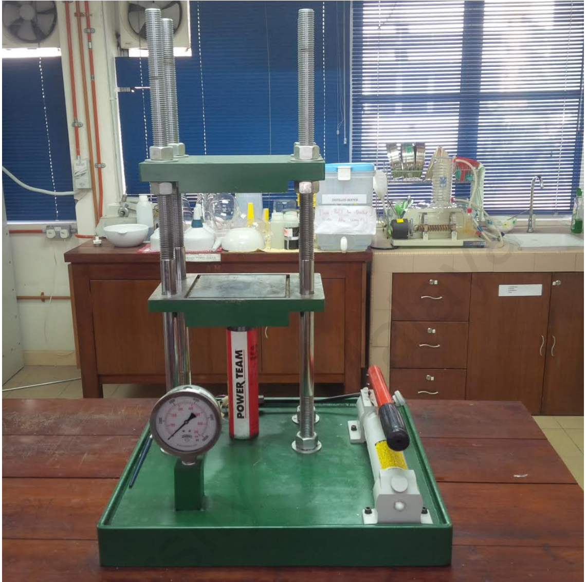
Figure C.8. The apparatus is used to exert a fixed amount of force onto the dies.
