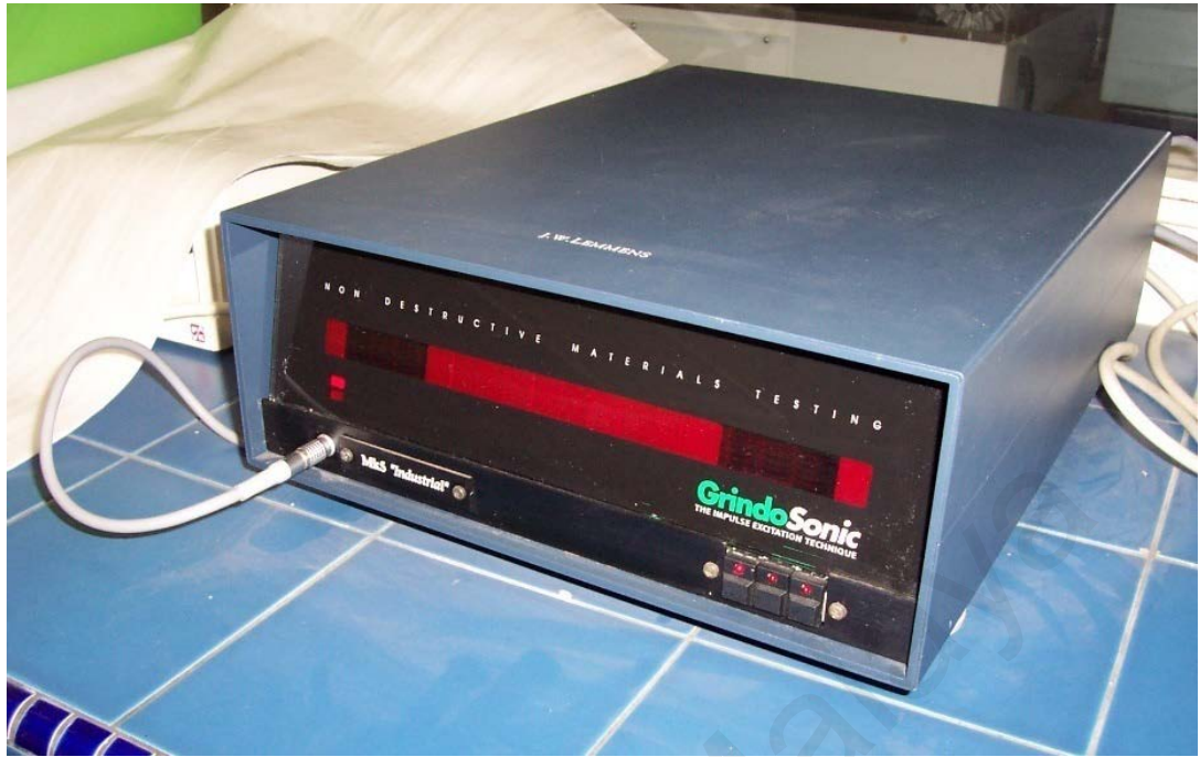
Figure C.17. The image above shows GrindoSonic: MK 5 "Industrial", Belgium; used to measure the Young's modulus of the bar samples.
