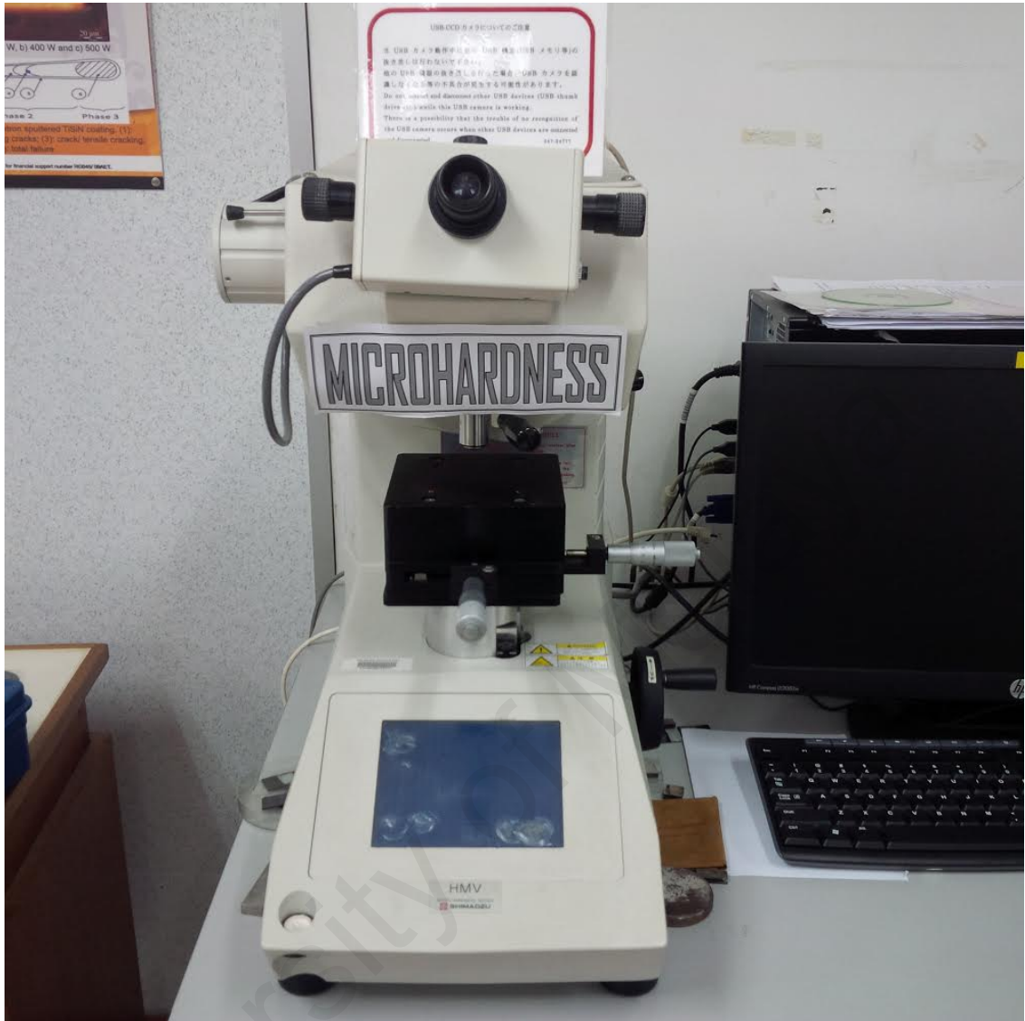
Figure C.15. The micro hardness machine used to evaluate the Vickers hardness and the fracture toughens of the samples.
