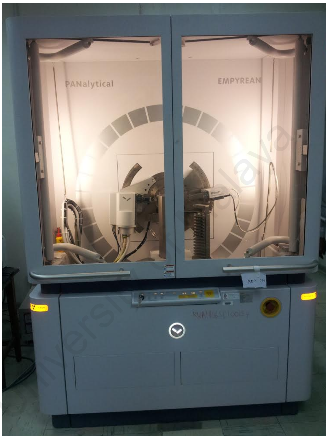
Figure C.13. The XRD machine used to check the phase composition of the forsterite.
