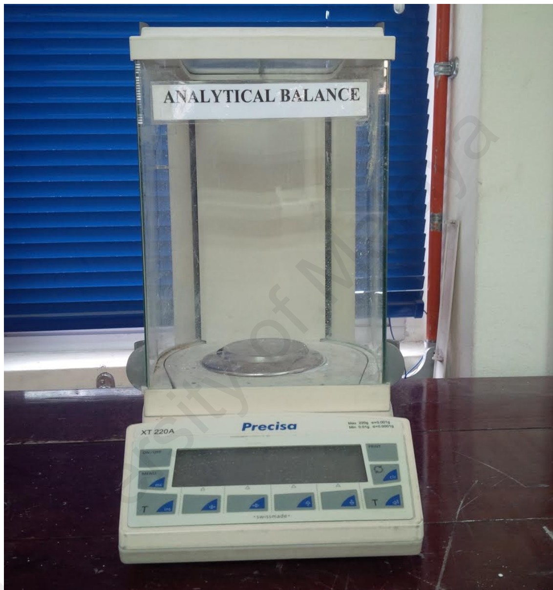
Figure C.1. The analytical balance used to measure the weight of the precursors.
