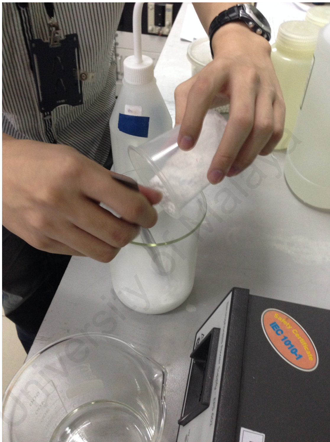
Figure C.2. The mixing process of the precursors into ethanol.
