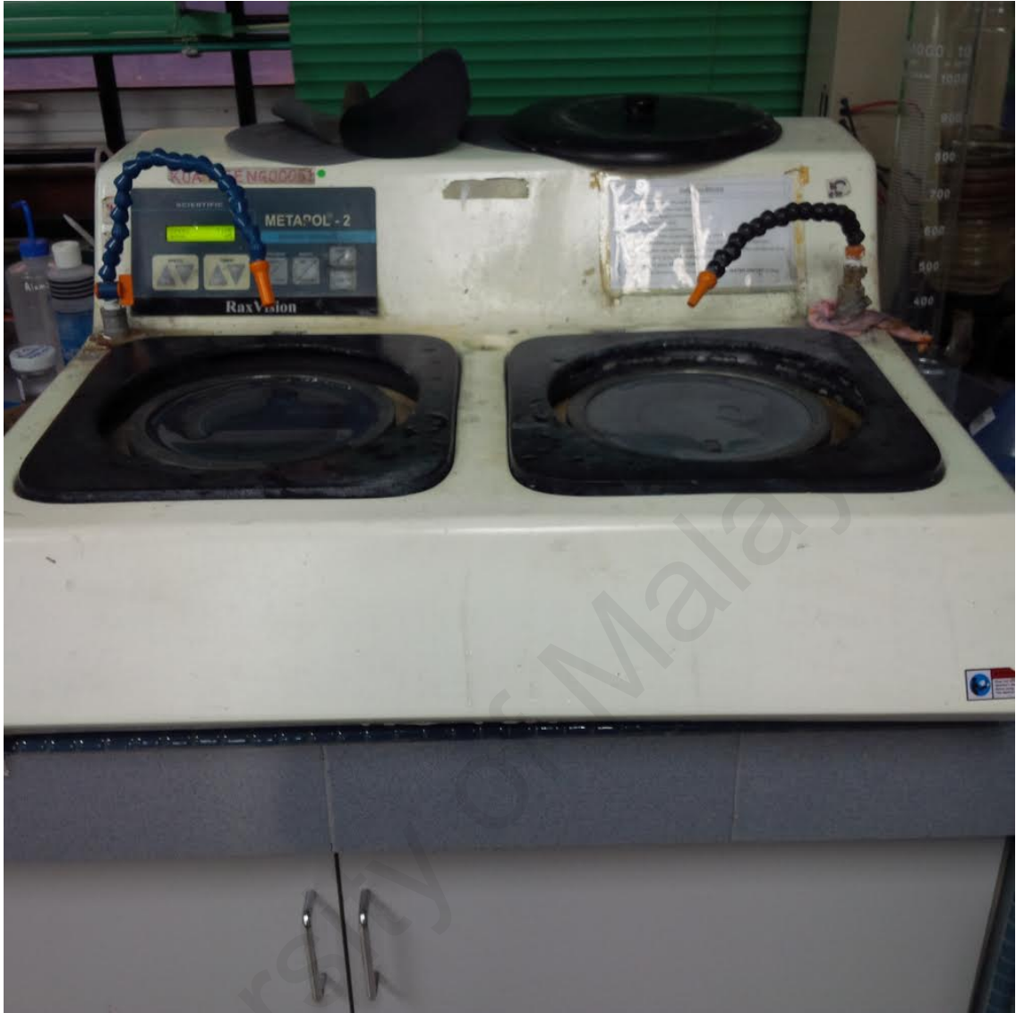
Figure C.11. the machine used to grind and polish the sintered forsterite compacts.
