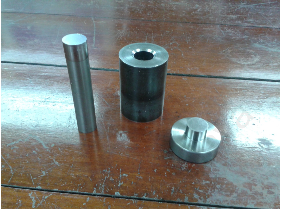
Figure C.7. The die used to compact the powders into disc or bar shape.
