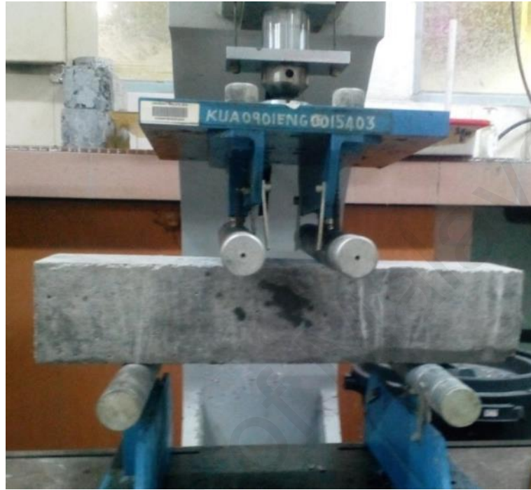
Figure 3.8: Flexural strength test
