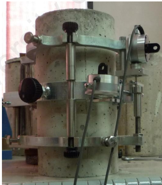
Figure 3.9: Static modulus of elasticity test
