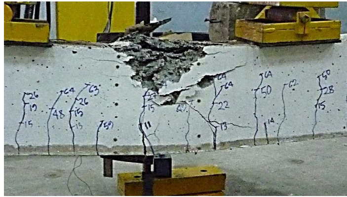
Figure 4.10: Concrete crushing and Cracks of Beam specimens at constant moment zone
