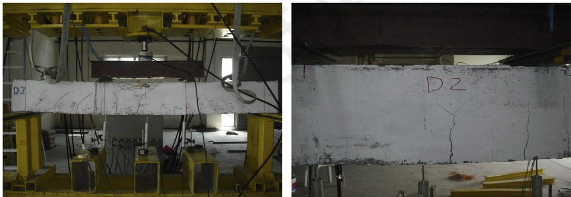
Figure 2.6: Crack patterns and failure mode of POC concrete beam (Mohammed et al., 2014)
