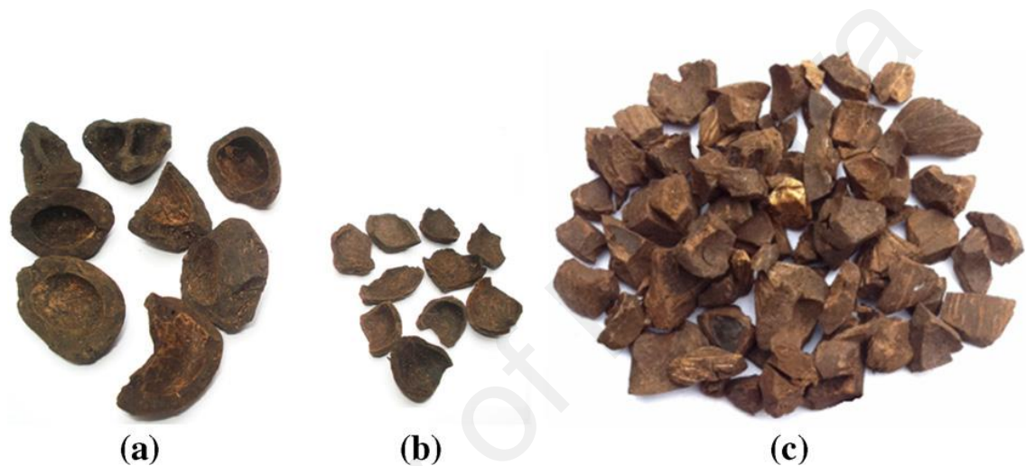
Figure 2.3: OPS aggregates: (a) original size, (b) original small size and (c) crushed from original size (Shafiq et al., 2011a)
