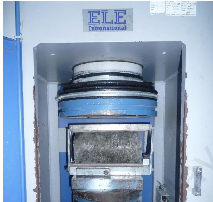
Figure 3.7: Splitting tensile strength test
