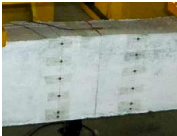
Figure 3.16: Demec points on a concrete beam
