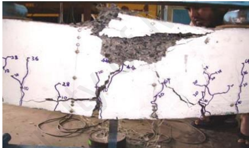
Figure 2.5: Failure modes of OPS concrete beam (Alengaram et al., 2008)
