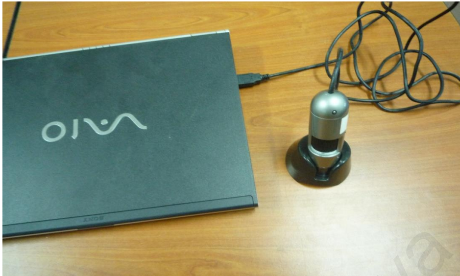
Figure 3.15: Dino-lite digital microscope for crack width measurement
