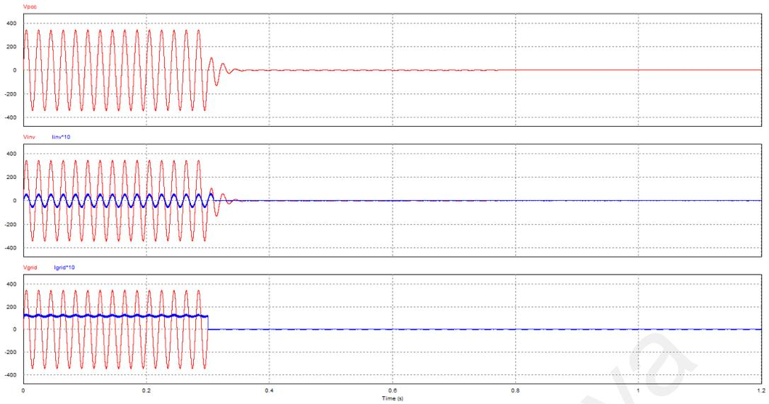
Figure 5.10: Simulation result under islanding detection at  $Q=2$
