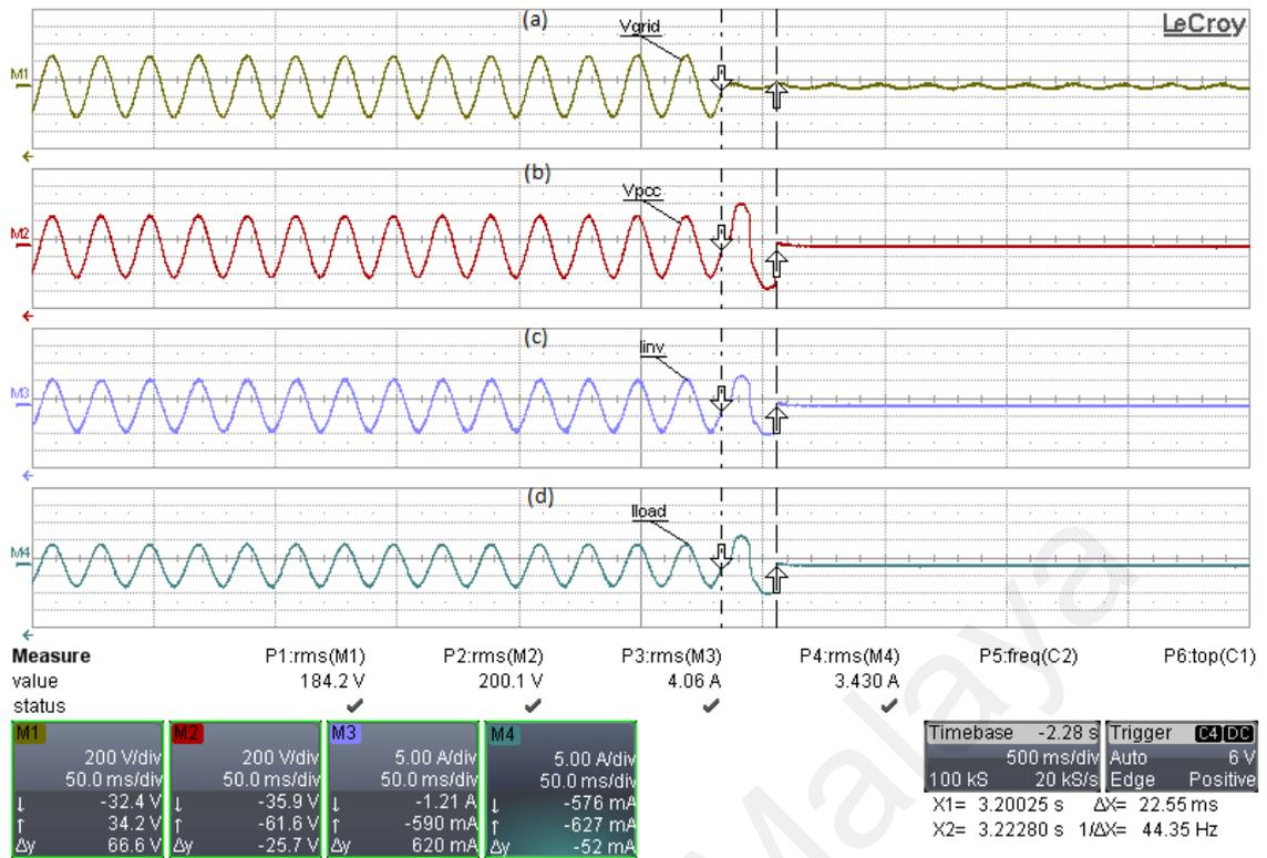
Figure 5.15: Experiment result for resistive R load under islanding operation for 75% (1.5kW) inverter output with (a):(M1)  $V_{grid}$ , (b):(M2)  $V_{PCC}$ , (c):(M3) the inverter output current and (d):(M4) load current
