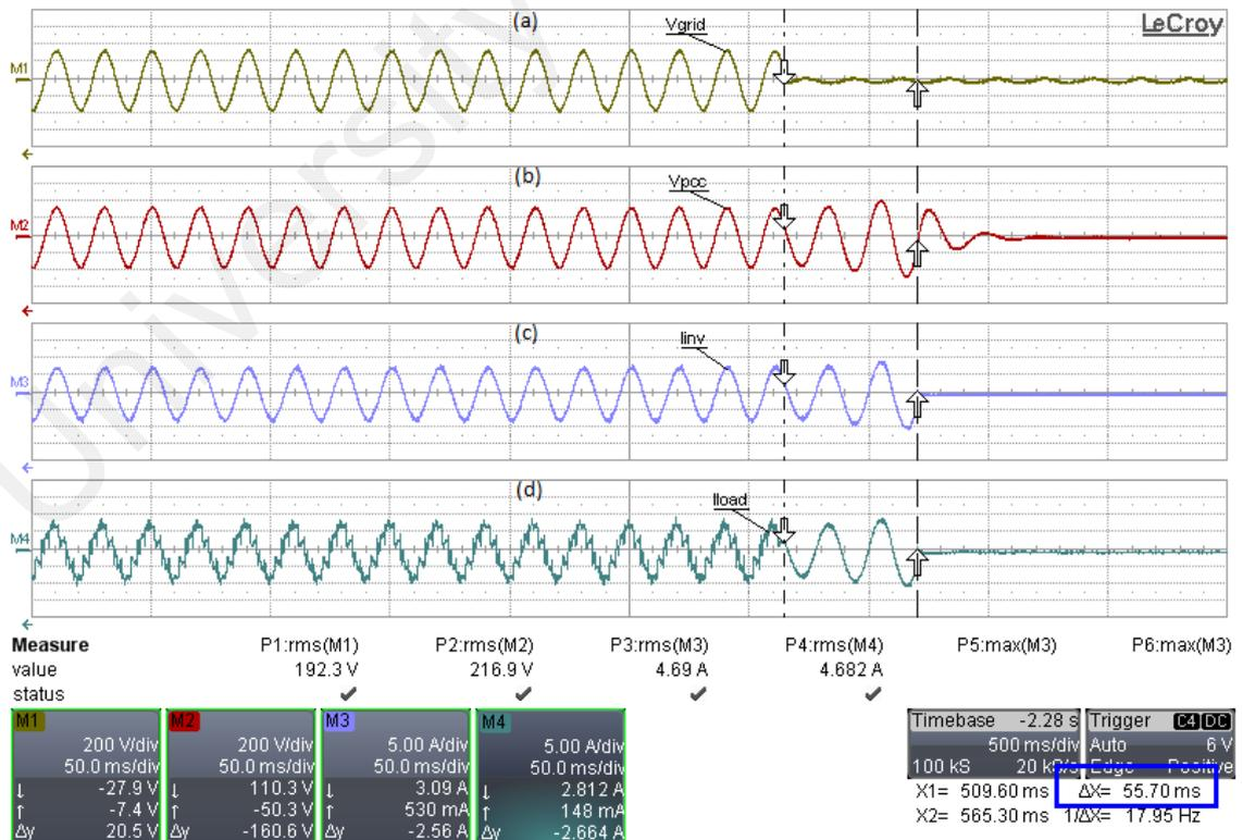
Figure 5.21: Experimental result for R-L-C load under islanding operation at  $Q=2.5$  with (a):(M1)  $V_{grid}$ , (b):(M2)  $V_{PCC}$ , (c): (M3) the inverter output current and (d):(M4) load current
