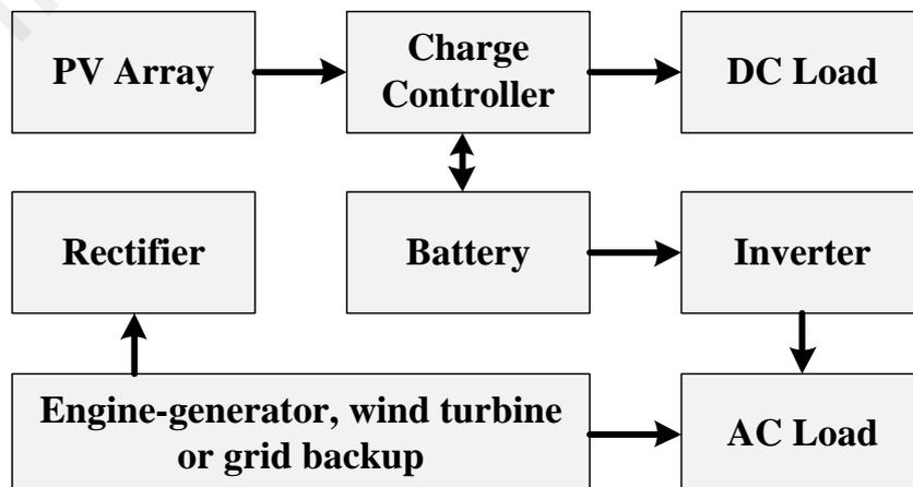
Figure 2.5: Schematic diagram of a hybrid PV system incorporating a PV array and additional power supply backup (www.fsec.ucf.edu)
