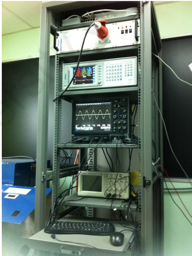
Figure B.6: PM6000 Power Analyzer and Lecroy Wave Runner 64Xi-A Oscilloscope.
