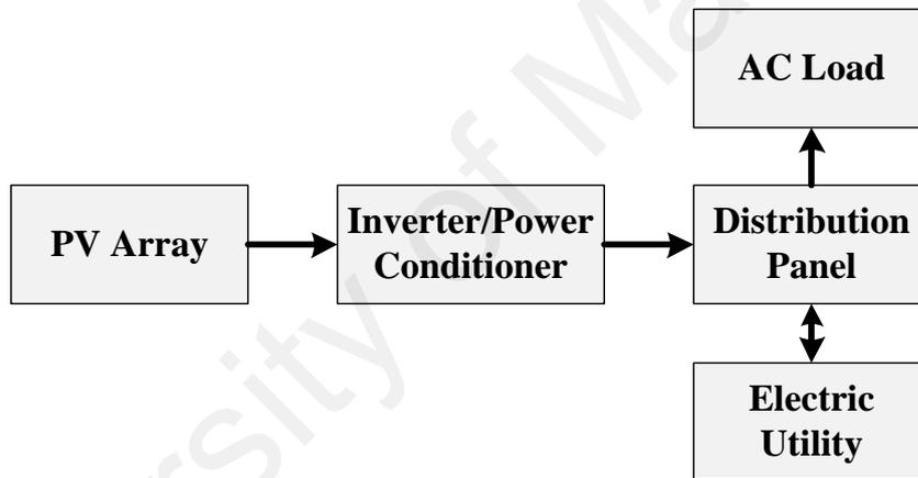
Figure 2.4: Diagram of grid-connected photovoltaic system (www.fsec.ucf.edu)
