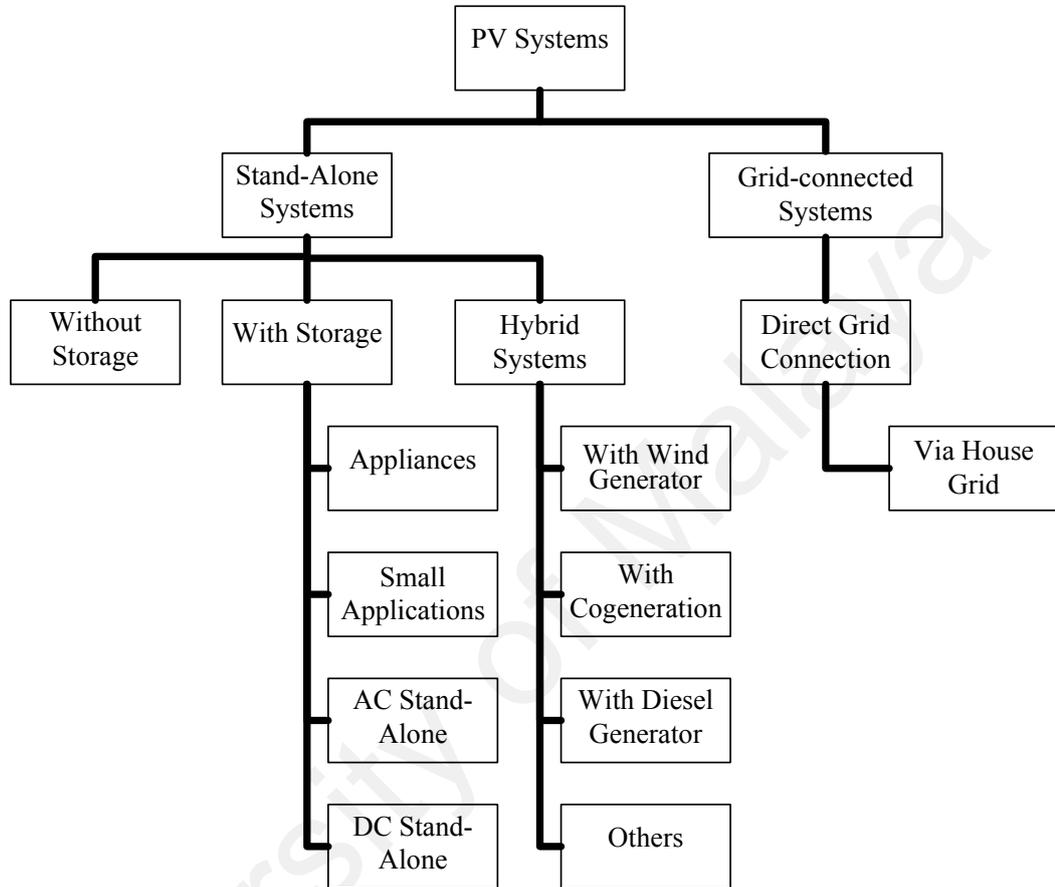
Figure 2.1: PV system configurations
