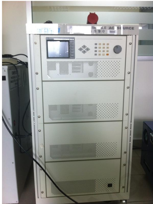
Figure B.9: Programmable AC source Model 6560
