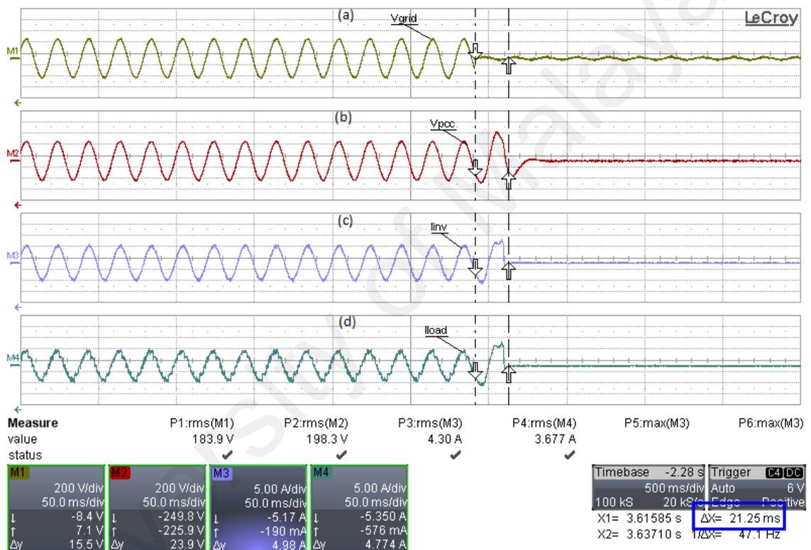
Figure 5.19: Experimental result for R-L-C load under islanding operation at  $Q=1$  with (a):(M1)  $V_{grid}$ , (b):(M2)  $V_{PCC}$ , (c):(M3) the inverter output current and (d):(M4) load current
