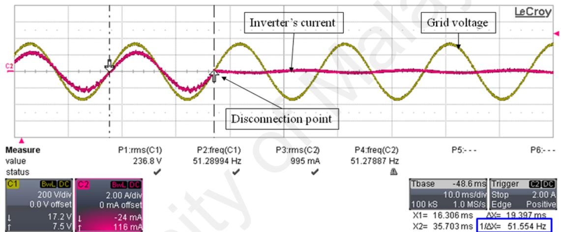
Figure 4.11: Over frequency islanding: (C1) Grid voltage and (C2) Inverter's current
