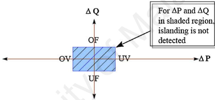
Figure 3.4: NDZ mapping in  $\Delta P$  versus  $\Delta Q$  space for OUV and OUF (Eltawil & Zhao, 2010; Ropp, et al., 2000; T5-09, 2002)
