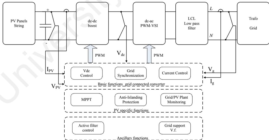
Figure 2.12: Block diagram of a single-phase grid connected PV inverter
