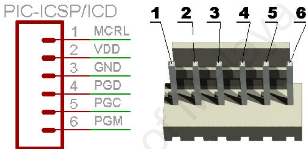
Figure C.2: Connector ICSP pin locations for PIC18F4550
