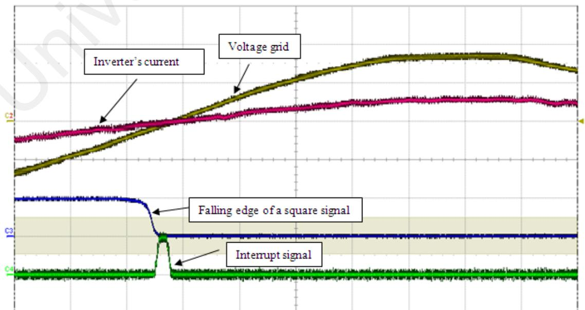
Figure 4.9: Falling edge of a square wave signal with the triggered interrupt
