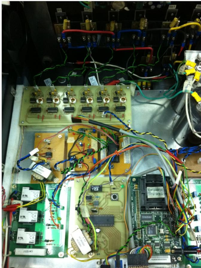
Figure B.3: Proposed circuits with PIC18F4550, gate drive circuits, sensor circuits and eZdsp™ F2812 board.
