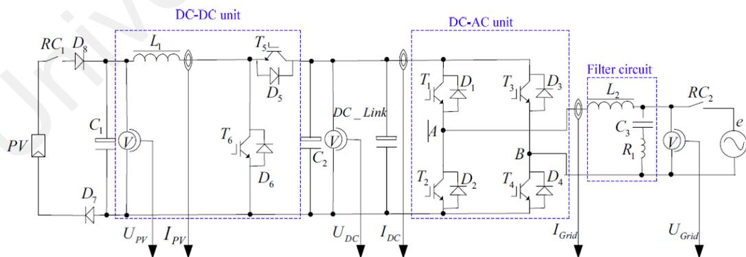
Figure 2.11: General main circuit block diagram (Zhou, et al., 2010)
