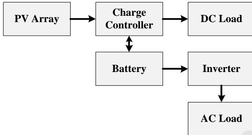
Figure 2.3: Diagram of stand-alone PV system with battery storage powering DC and AC loads (www.fsec.ucf.edu)
