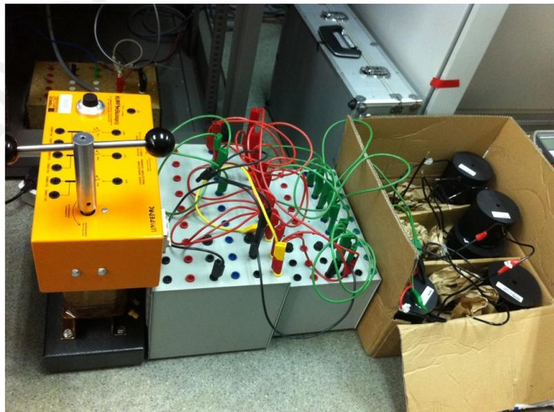
Figure B.2: Variable Inductor and Capacitor loads
