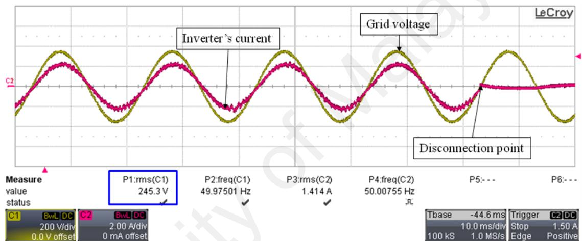
Figure 4.7: Over voltage islanding: (C1) Grid voltage and (C2) Inverter's current
