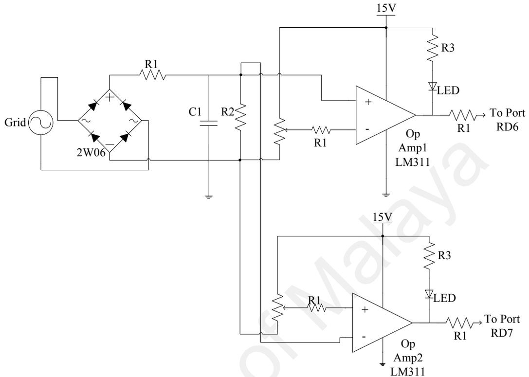
Figure 4.4: Under and over voltage circuit
