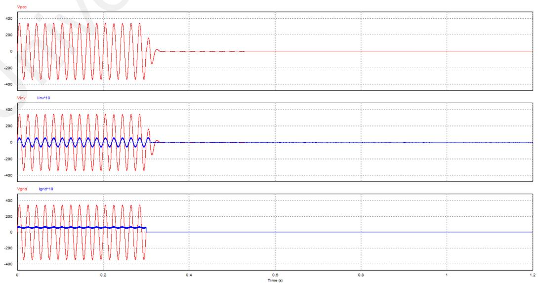
Figure 5.9: Simulation result under islanding detection at  $Q=1$
