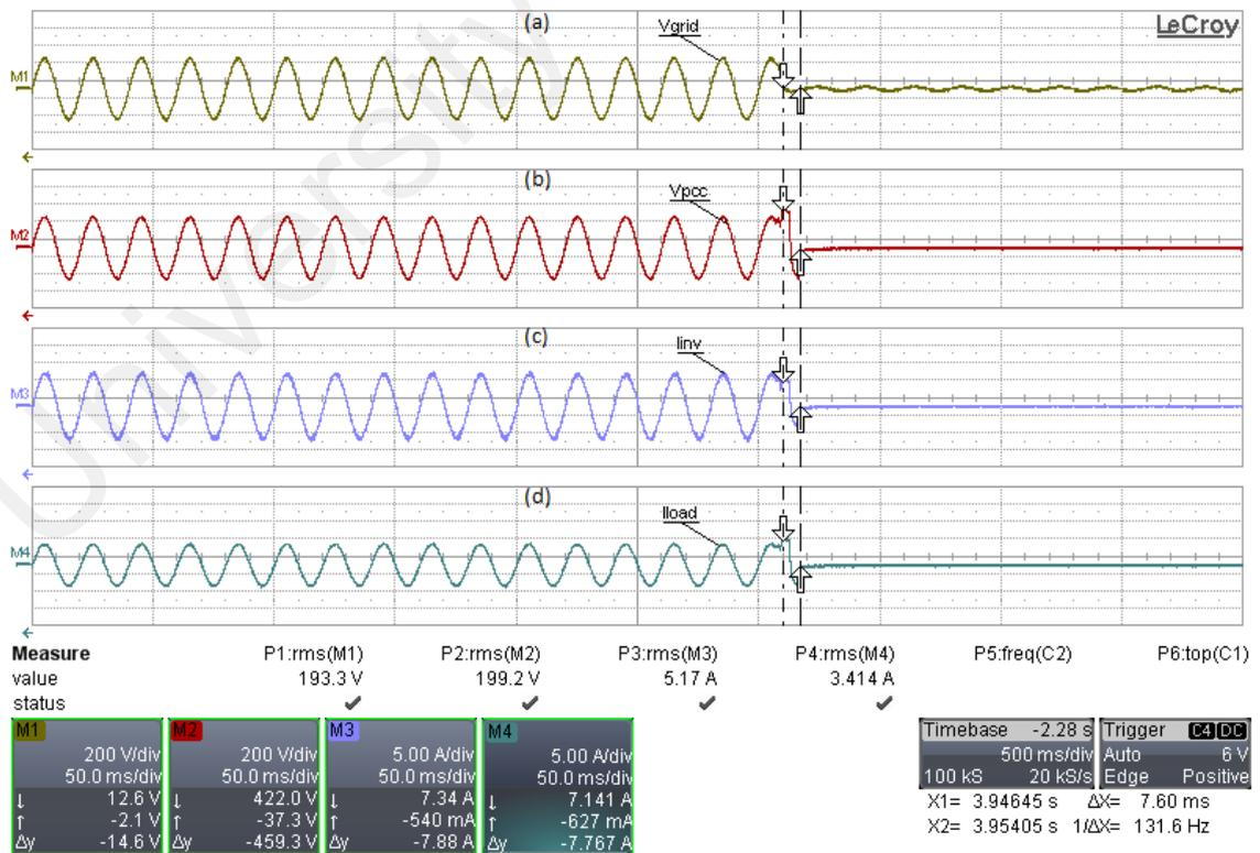
Figure 5.16: Experiment result for resistive R load under islanding operation for 100% (2kW) inverter output with (a):(M1)  $V_{grid}$ , (b):(M2)  $V_{PCC}$ , (c):(M3) the inverter output current and (d):(M4) load current
