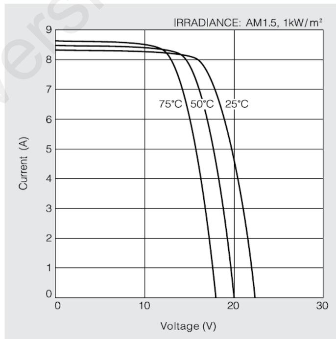
Figure 2.10: I-V characteristics of a PV Cell array for various values of temperature  $T$  at  $1000W/m^2$  irradiance, for KD135GX-LPU (Kyocera, 2008)
