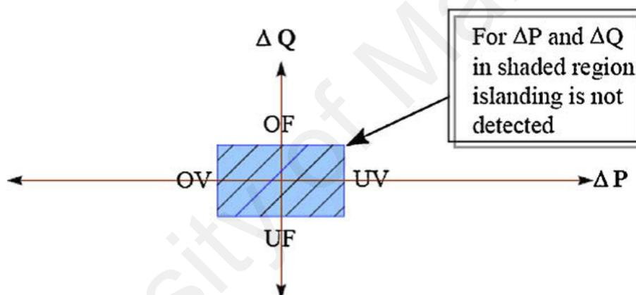
Figure 5.1: NDZ mapping in  $\Delta P$  versus  $\Delta Q$  space for the proposed method
