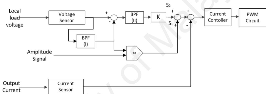
Figure 3.5: Control of the grid-connected inverter as virtual resistor or virtual capacitor (Chiang, et al., 2012; Chiang, et al., 2010)
