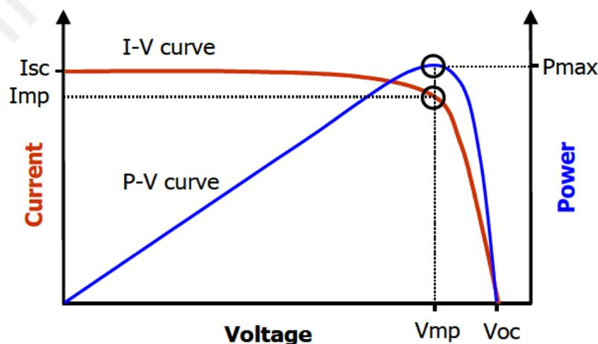
Figure 2.8: The I-V and P-V curves of a photovoltaic device. The P-V curve is calculated from the measured I-V curve
