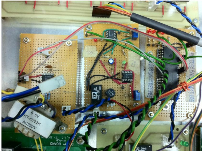
Figure B.1: The proposed under/over voltage and under/over frequency circuits
