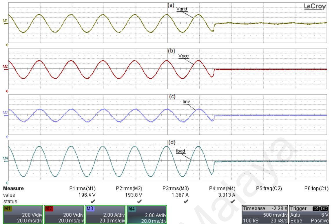
Figure 5.13: Experiment result for resistive R load under islanding operation for 25% (500W) inverter output with (a):(M1)  $V_{grid}$ , (b):(M2)  $V_{PCC}$ , (c):(M3) the inverter output current and (d):(M4) load current
