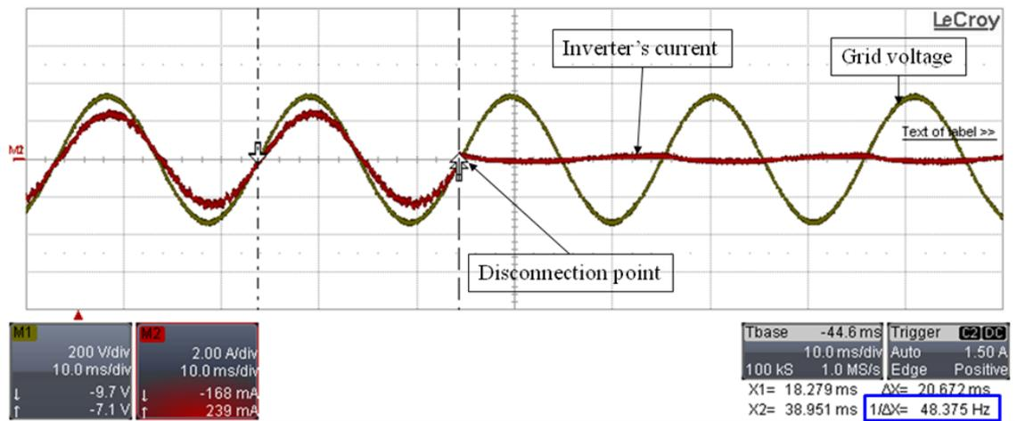
Figure 4.10: Under frequency islanding: (C1) Grid voltage and (C2) Inverter's current
