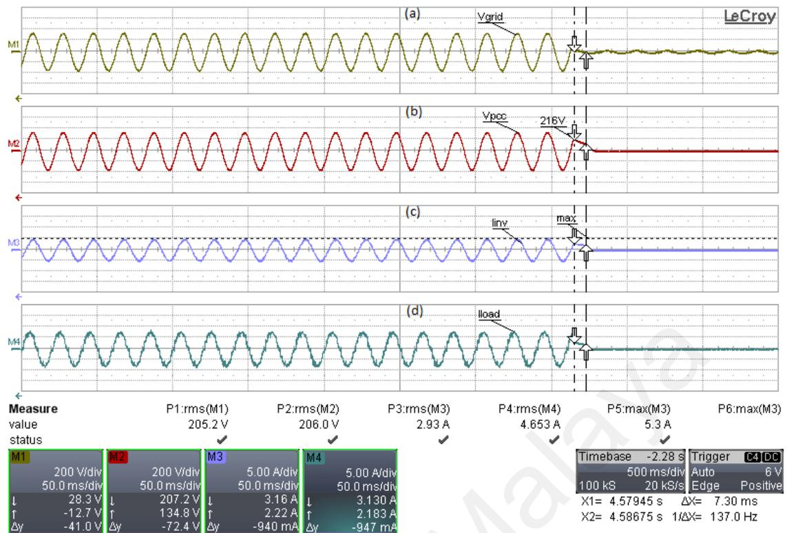
Figure 5.18: Experimental result for R-C load under islanding operation with (a):(M1)  $V_{grid}$ , (b):(M2)  $V_{PCC}$ , (c):(M3) the inverter output current and (d):(M4) load current
