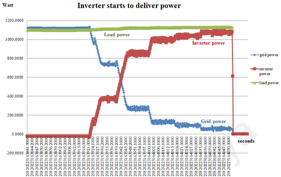
Figure 5.23: The inverter comes "on-line" and gradually increases its output to 1kW
