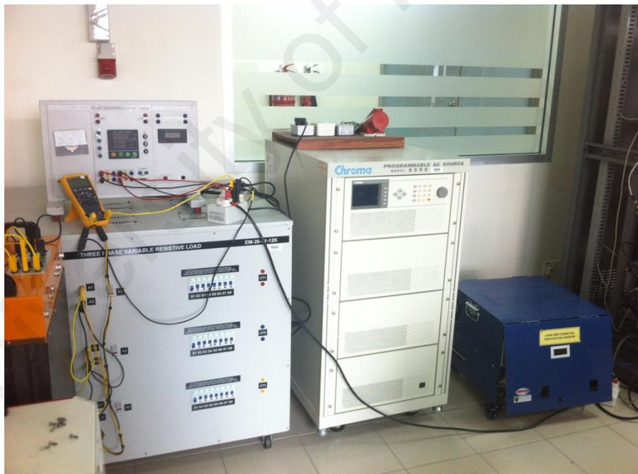
Figure B.12: Islanding Test with Resistive load, inverter and Programmable AC source Model 6560
