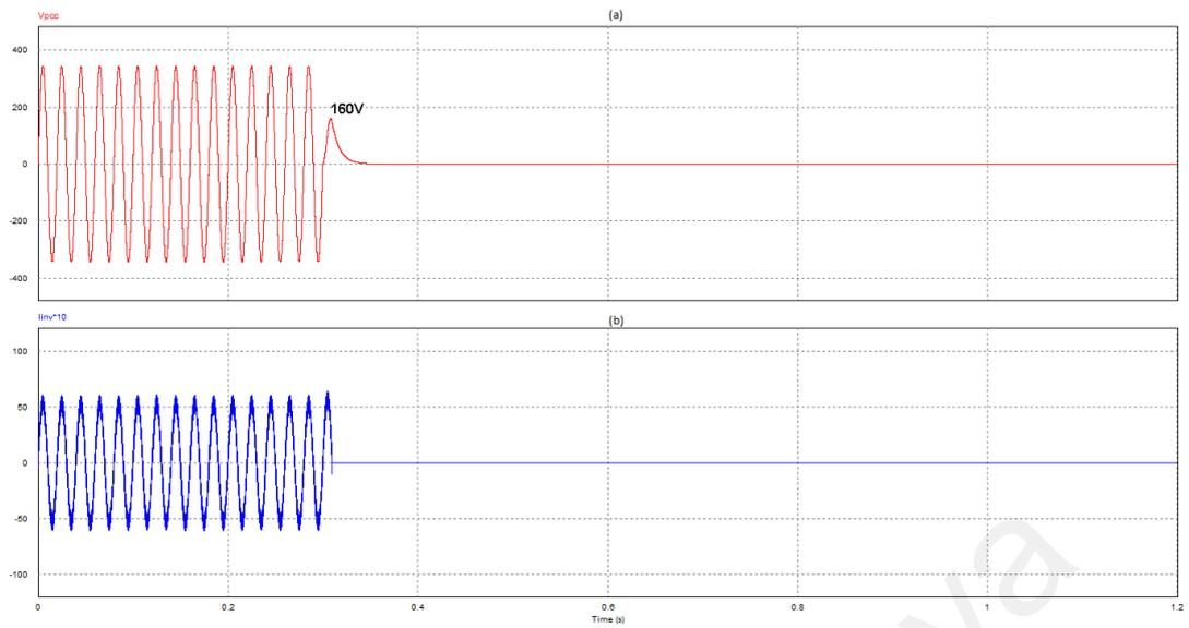
Figure 5.8: Simulation result for R-C load under islanding operation with  $Q=2.5$  and  $P=1\text{kW}$  with (a):  $V_{PCC}$ , and (b):  $I_{inv} * 10$
