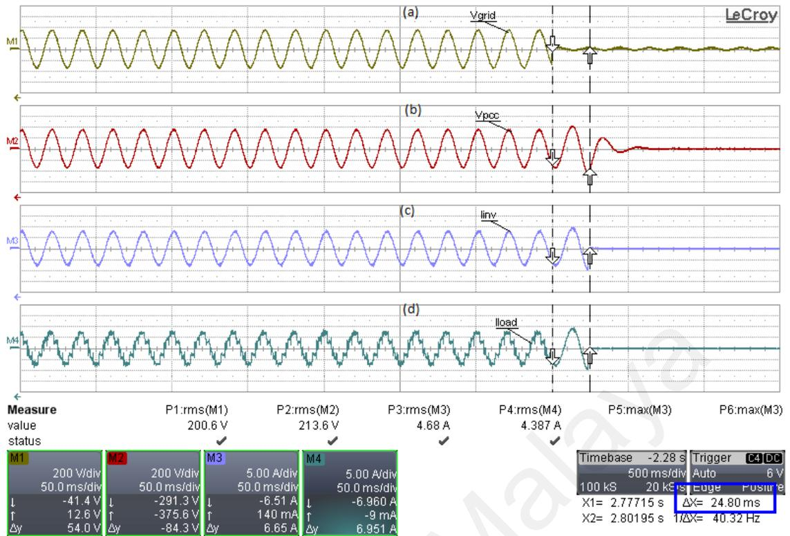
Figure 5.20: Experimental result for R-L-C load under islanding operation at  $Q=2$  with (a):(M1)  $V_{grid}$ , (b):(M2)  $V_{PCC}$ , (c): (M3) the inverter output current and (d):(M4) load current
