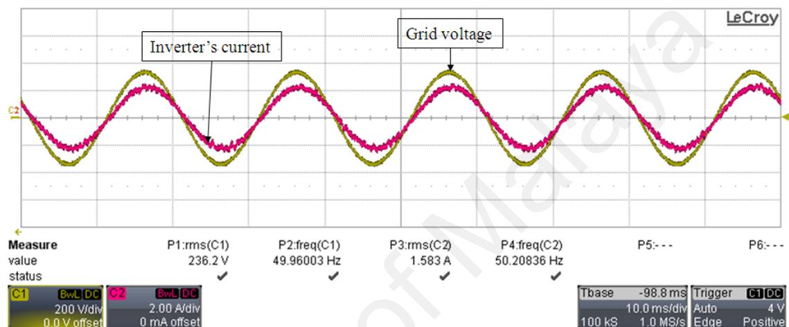
Figure 4.5: Normal condition at 240V and 50Hz: (C1) Grid voltage and (C2) Inverter's current
