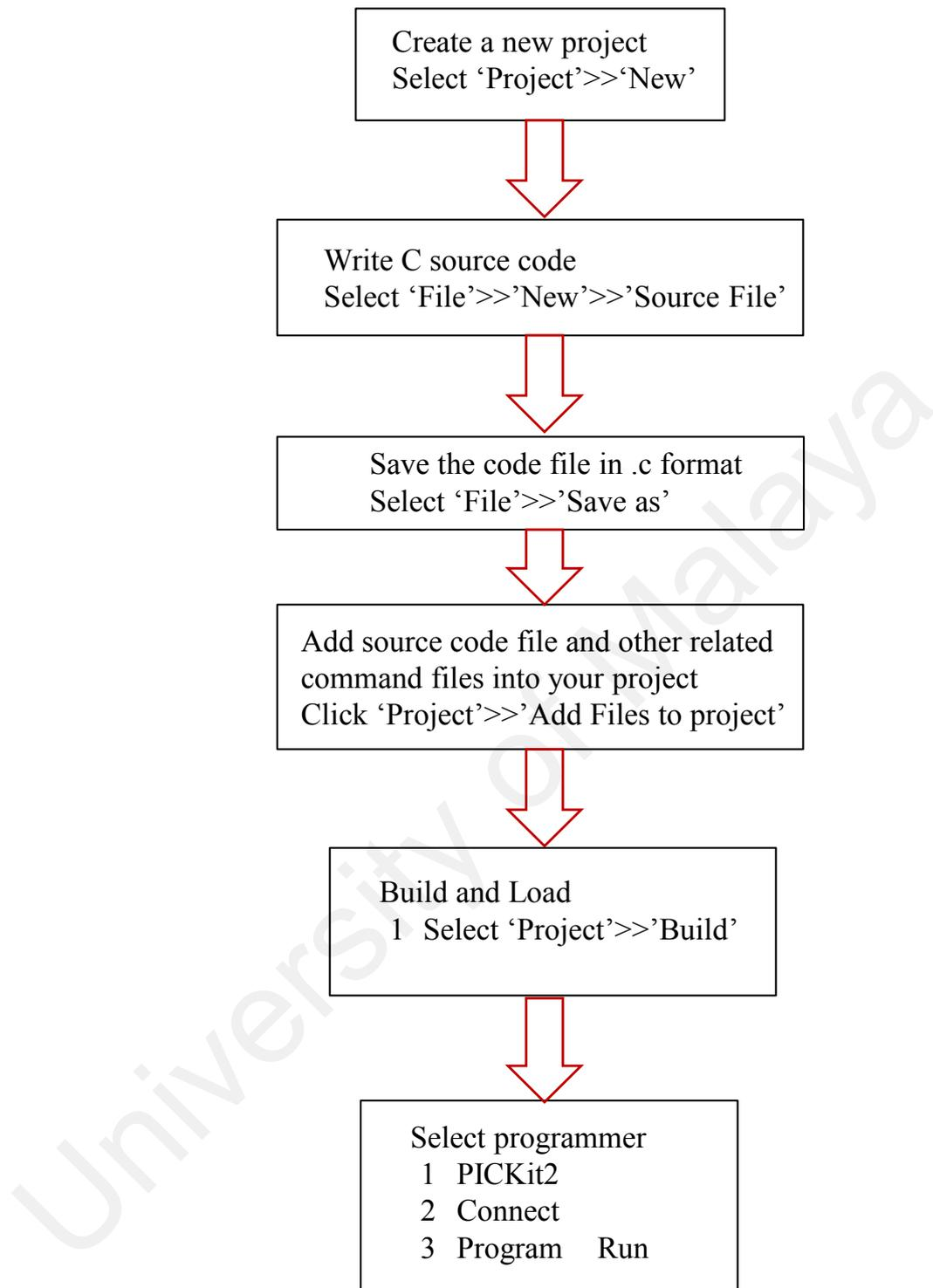
Figure 4.18: Develop, build and run a program code in MPLAB IDE
