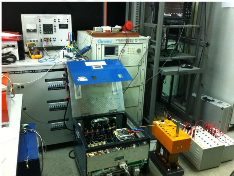
Figure B.4: Three Phase Variable Resistive Load and Single Phase Grid Connected PV Inverter.
