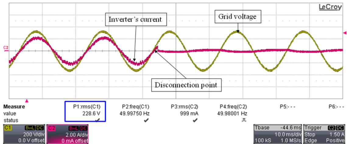
Figure 4.6: Under voltage islanding: (C1) Grid voltage and (C2) Inverter's current
