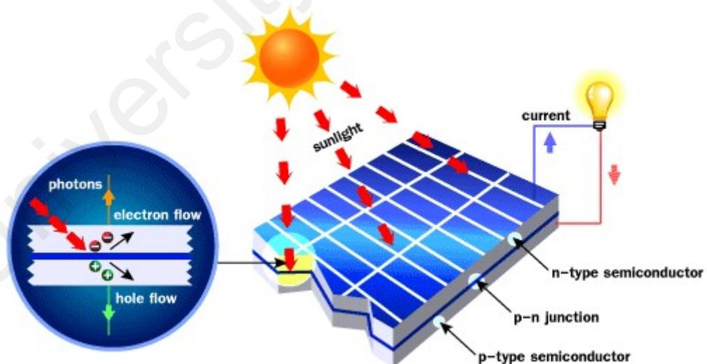
Figure 2.6: Work flow of a PV cell (www.pvsolarchina.com)
