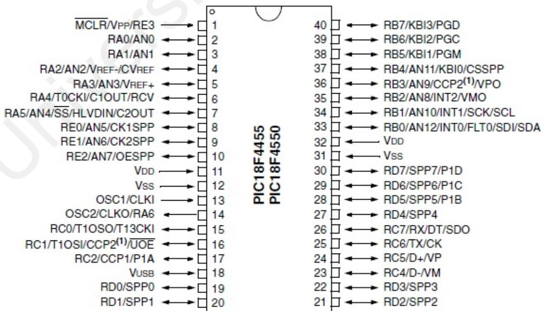
Figure C.1: 40 pin diagrams of PIC18F4550.
