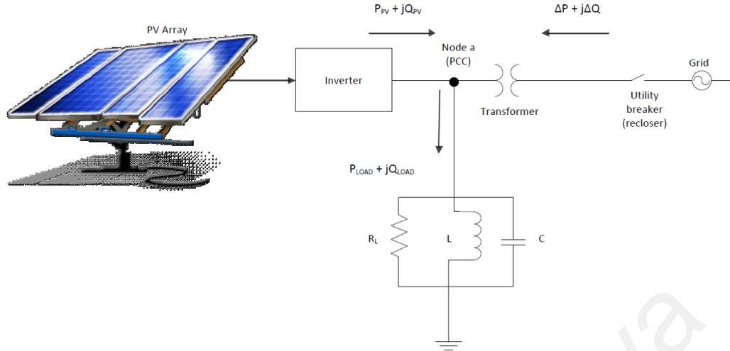
Figure 3.1: PV System/Utility Feeder Configuration, with definitions for power flow and terms (T5-09, 2002)
