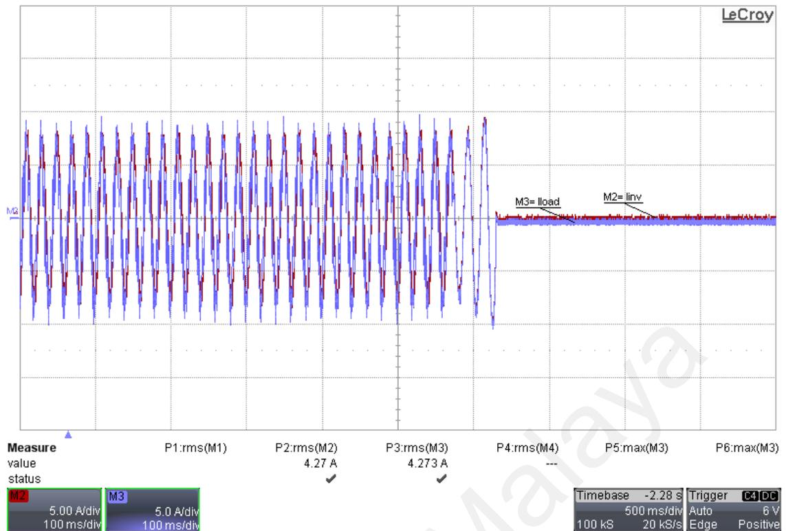
Figure 5.22: Experiment results for R-L-C load under islanding operation at  $Q=2.5$  with (M2) the inverter output current, (M3) load current
