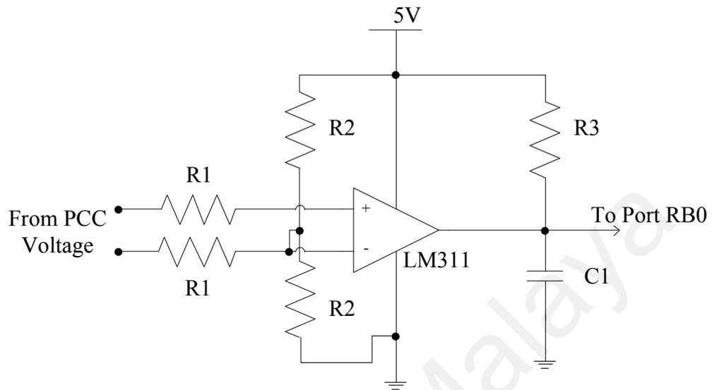
Figure 4.8: Zero crossing detector circuit for under and over frequency detection
