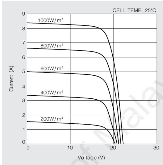
Figure 2.9: I-V characteristics of a PV cell array for various values of irradiance  $S$  at  $25^\circ C$ , for KD135GX-LPU (Kyocera, 2008)
