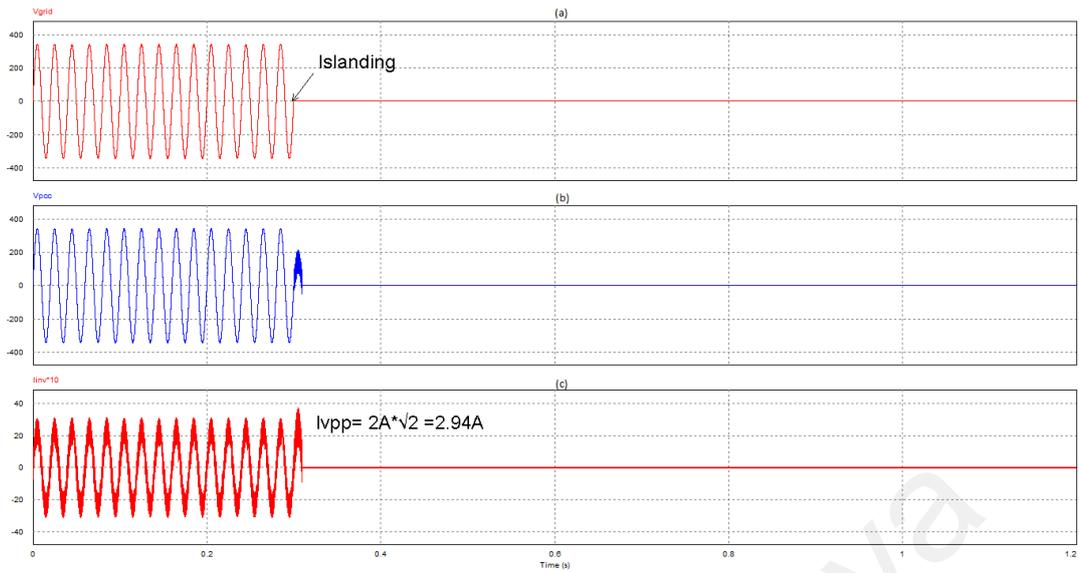
Figure 5.3: Simulation result for R load with 25% (500W) inverter output under islanding operation with (a):  $V_{grid}$ , (b):  $V_{PCC}$ , and (c):  $I_{inv} * 10$
