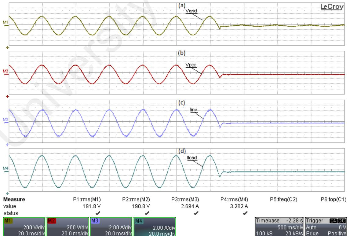
Figure 5.14: Experiment result for resistive R load under islanding operation for 50% (1kW) inverter output with (a):(M1)  $V_{grid}$ , (b):(M2)  $V_{PCC}$ , (c):(M3) the inverter output current and (d):(M4) load current
