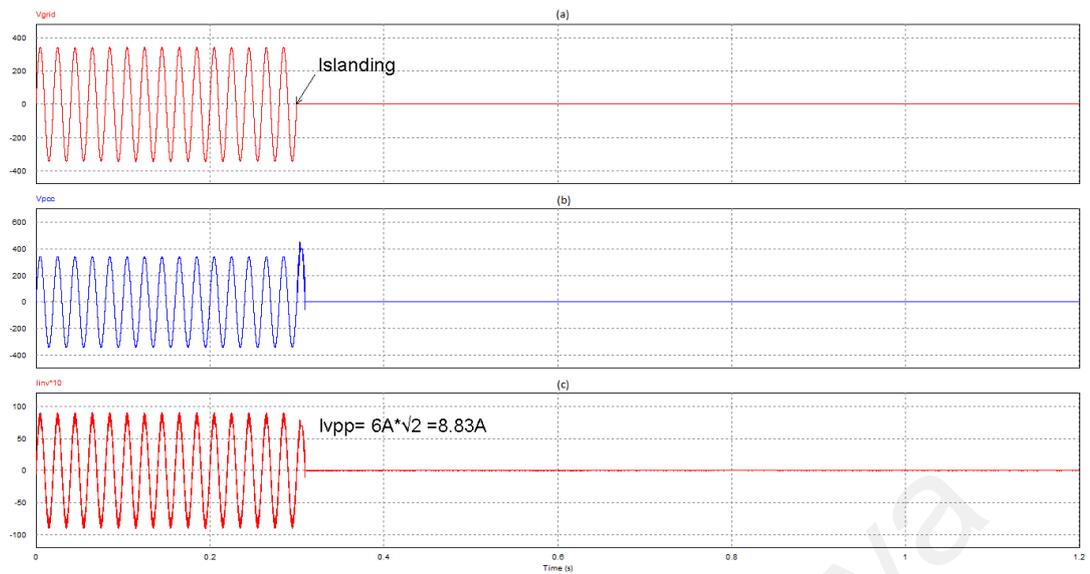
Figure 5.5: Simulation result for R load with 75% (1.5kW) inverter output under islanding operation with (a):  $V_{grid}$ , (b):  $V_{PCC}$ , and (c):  $I_{inv} * 10$
