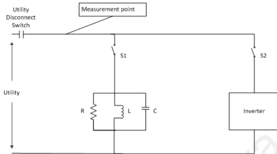
Figure 3.3: Anti-islanding test circuit ("IEEE Recommended Practice for Utility Interface of Photovoltaic (PV) Systems," 2000)
