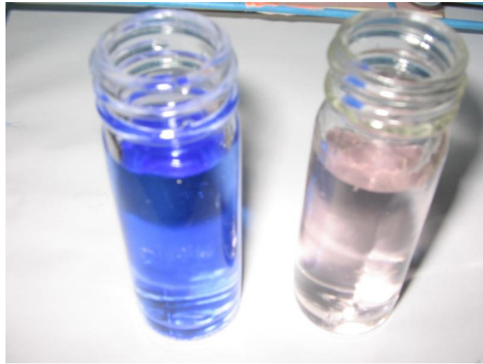
Figure 3. Comparison of initial dye concentration and result after 12 hr with 0.6 \text{ l min}^{-1} of air flow rate
