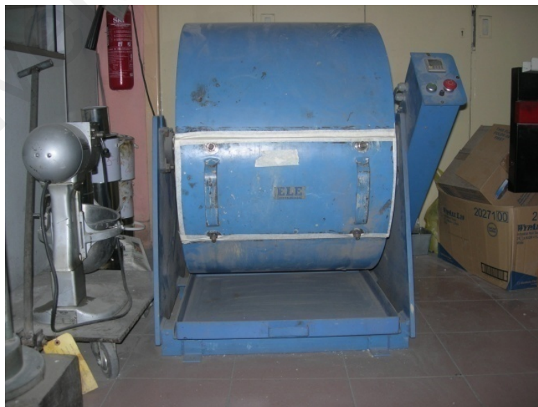
Figure 3.4: Los Angeles grinding machine
