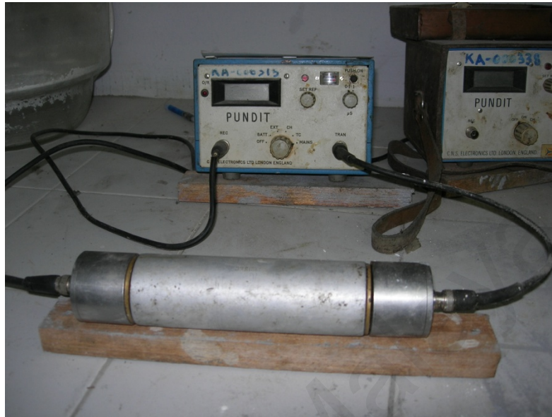
Figure 3.16: Apparatus for ultrasonic pulse velocity (UPV)
