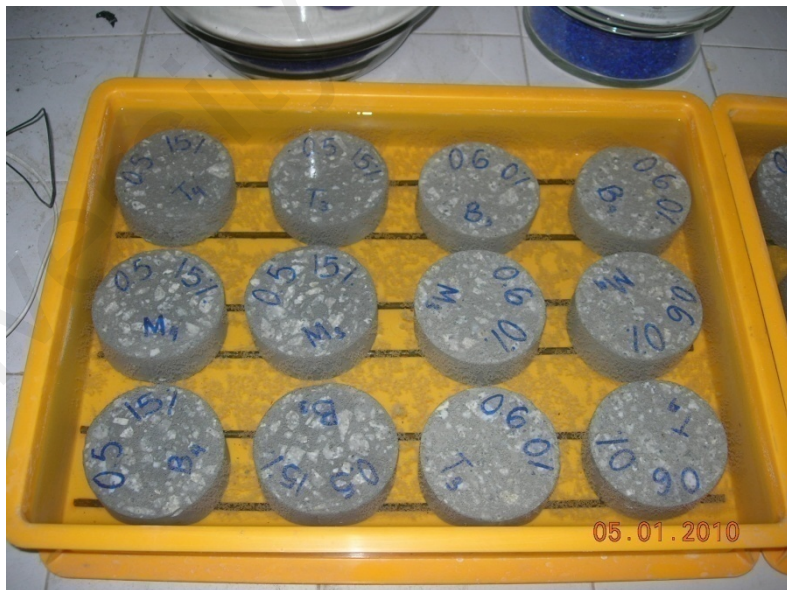
Figure 3.20: Specimens immersion in cool water
