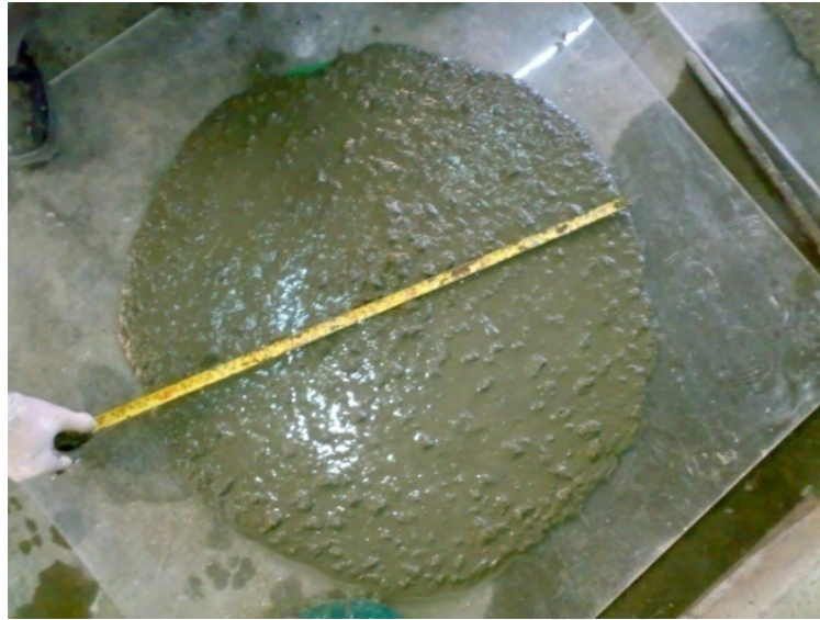
Figure 3.8: Measurement of slump flow
