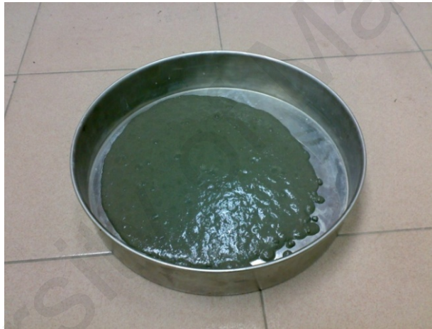
Mortar passed through sieve
