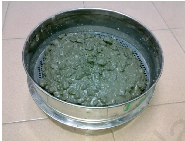
Initial stage of sieve segregation test
