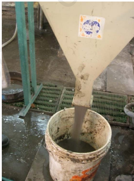
Figure 3.10: Testing of V-funnel flow
