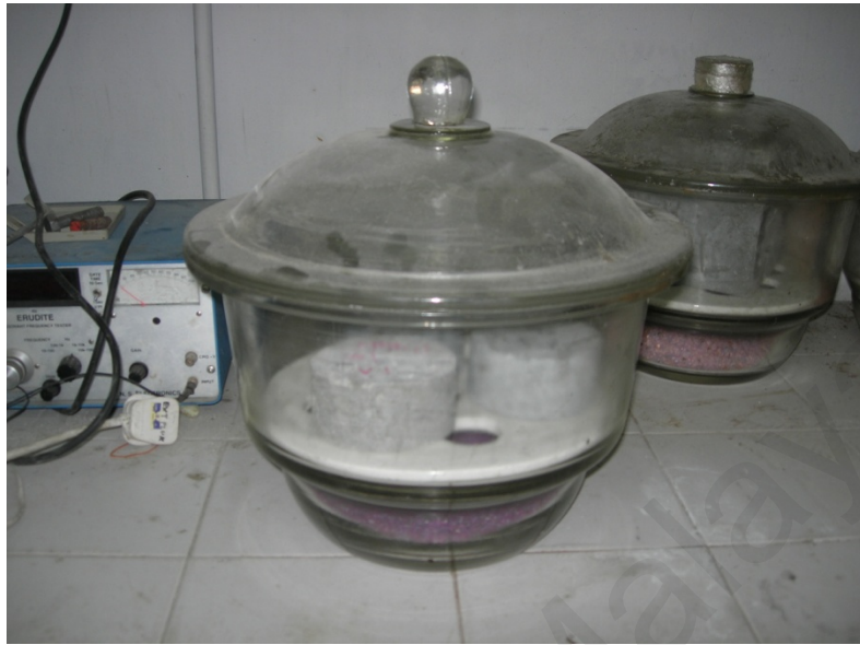
Figure 3.19: Specimens cooling in desiccators
