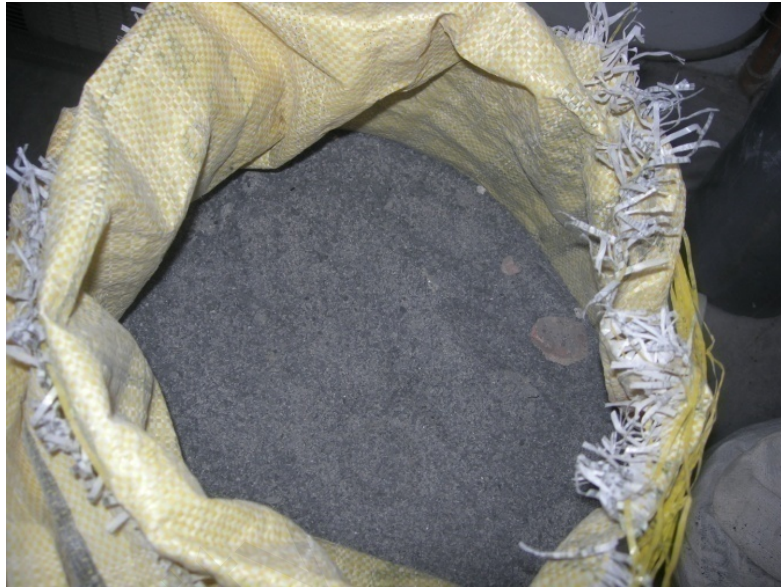
Figure 3.3: Raw palm oil fuel ash
