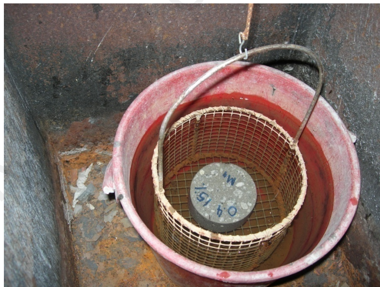
Figure 3.22: Buoyant mass measurement of specimen
