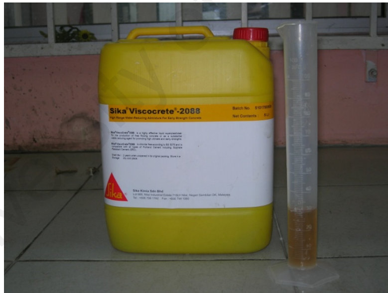
Figure 4.6: High-range water reducer (Sika viscocrete-2088)
