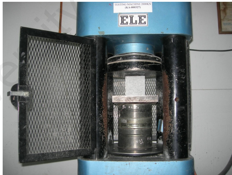
Figure 3.15: Compression testing machine for compressive strength test
