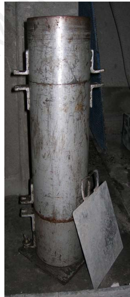
Figure 3.13: Details of the simplified segregation column apparatus
