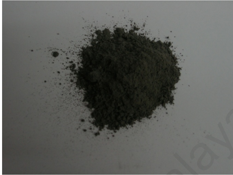
Figure 3.5: Ground palm oil fuel ash
