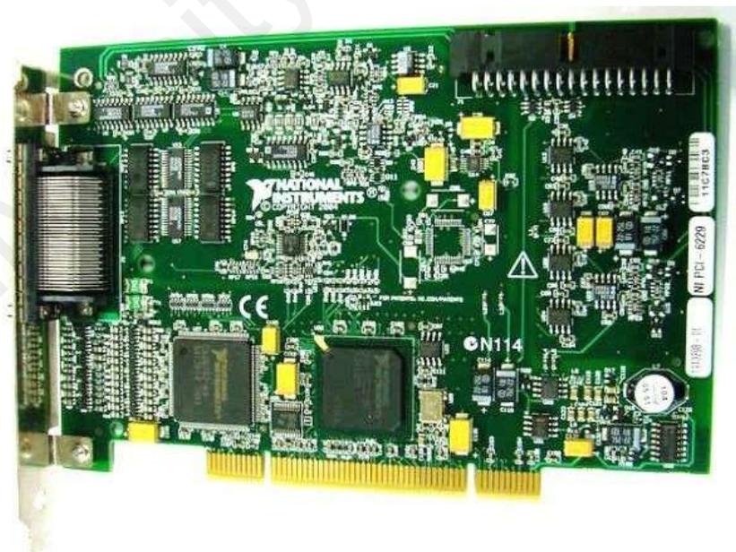
Figure 3.19 NI PCI-6229 DAQ card from National Instruments.
