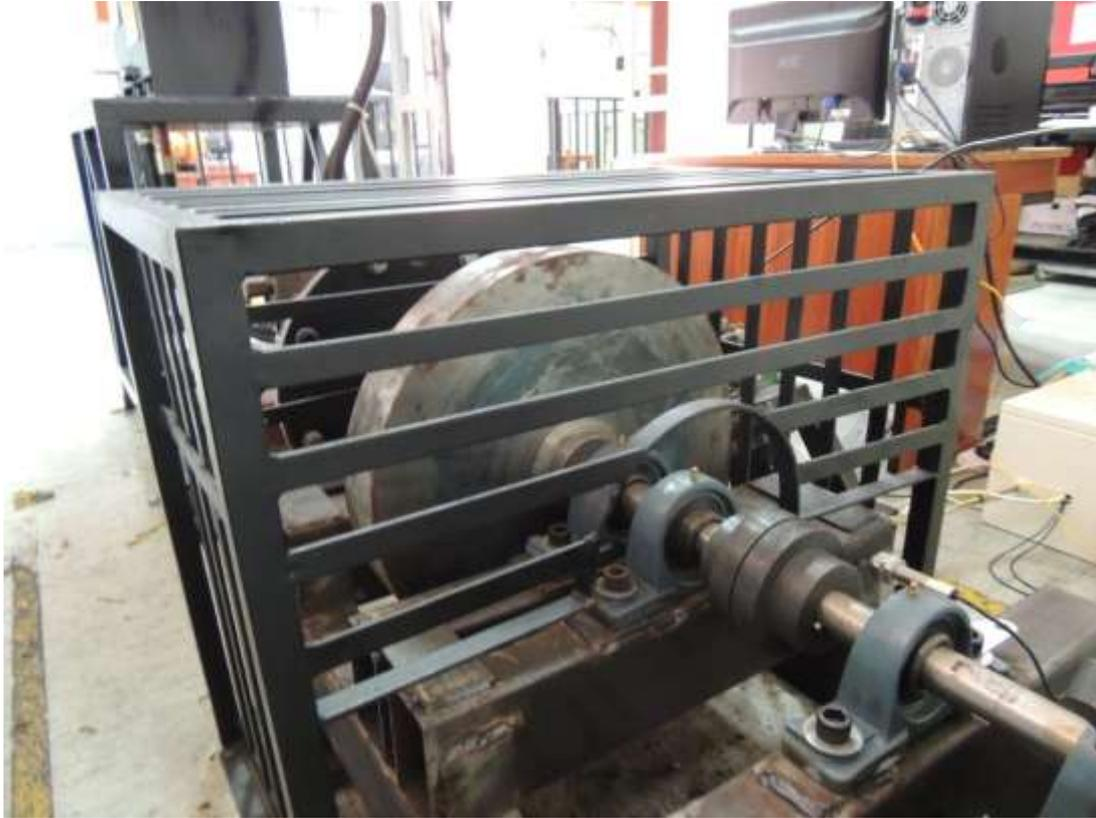
Figure 3.11 The flywheel inside a steel cage for safety purposes
