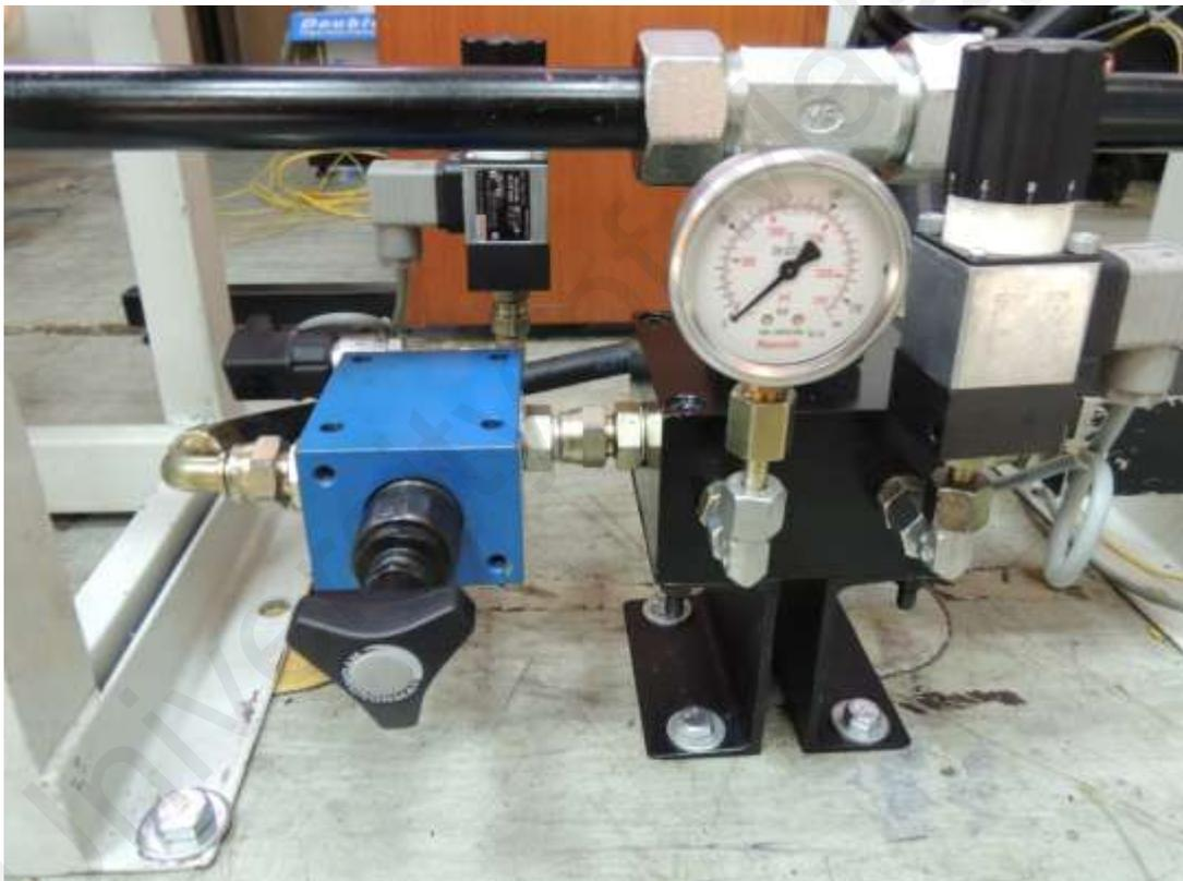
Figure 3.12 Pressure Relief Valve (blue block) with manual adjusting knob
