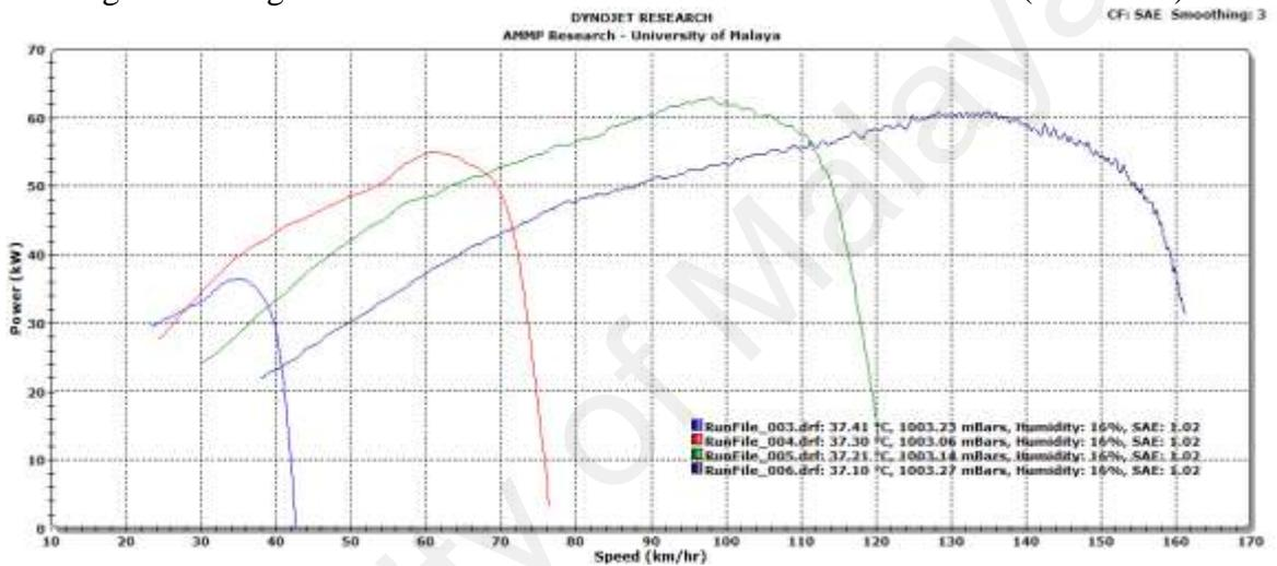
Figure 5.10 Engine Data for ISUZU NKR 71 E: Power versus Speed (Gear 1 – 4)
