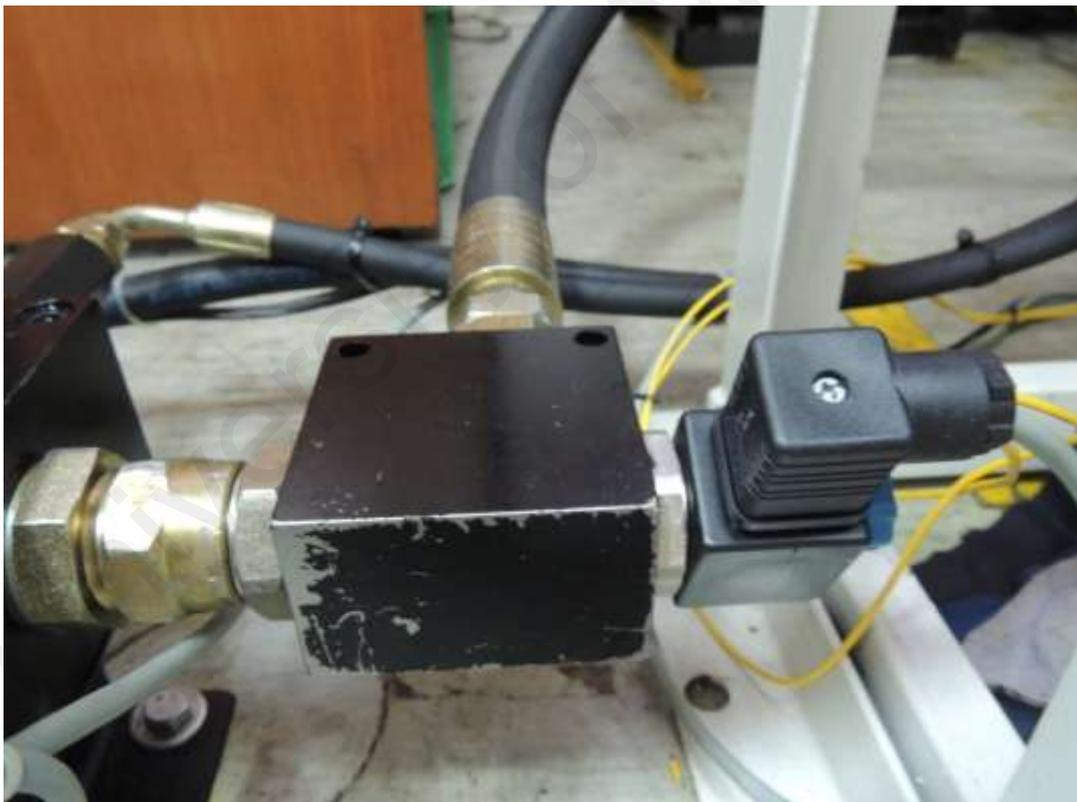
Figure 3.13 Valve B (inside black block) with coil compartment on its right.
