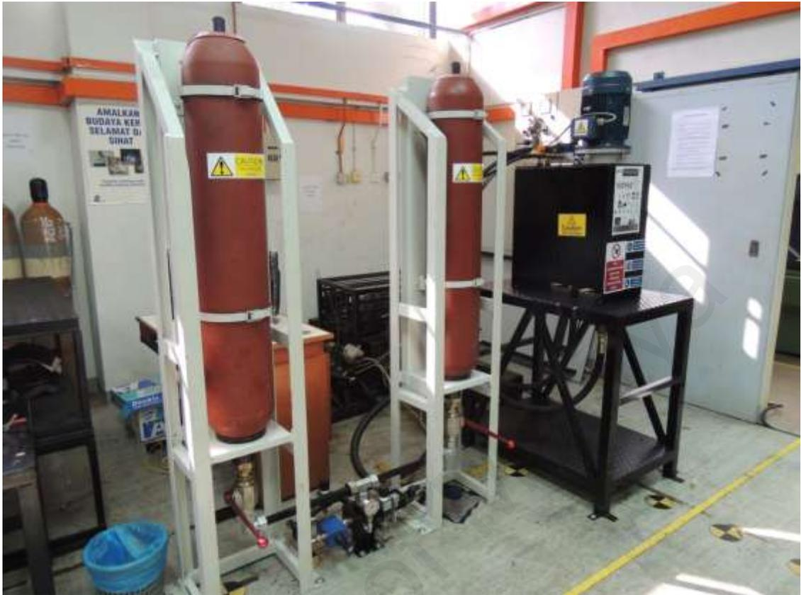
Figure 3.9 Accumulators in the form of red tanks are positioned beside the power pack.
