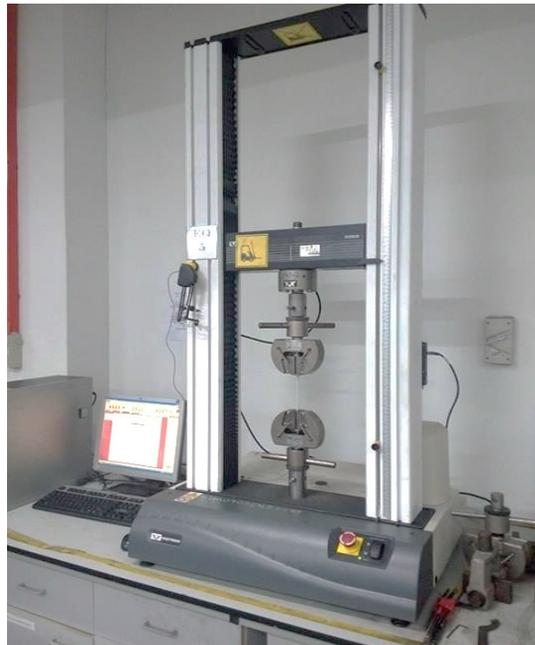
Figure 3.4: INSTRON universal testing instrument
