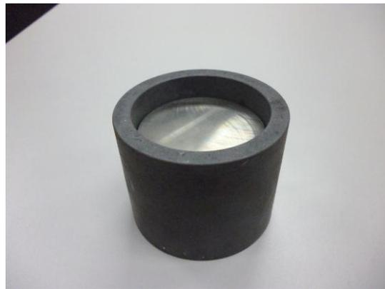
Figure 3.4: Fabricated die
