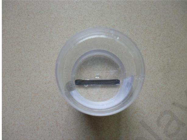
Figure 3.12: Embedded sample immersed in the 20 ml SBF
