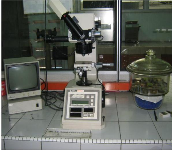
Figure 3.17: Microhardness tester
