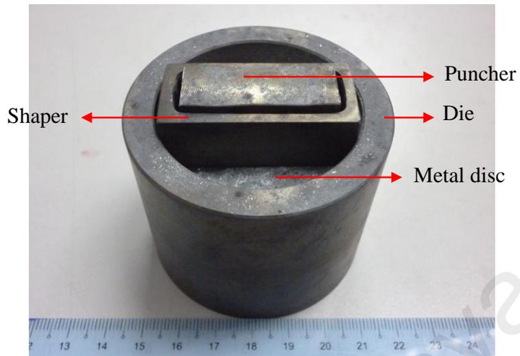
Figure 3.9: Fabricated die with the Ti-6Al-4V substrate and HA powder inside it, to be placed in the compression test machine for embedment process
