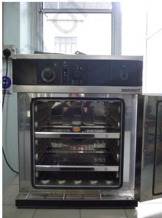
Figure 3.13: Sample in SBF is placed in the furnace at constant temperature of
