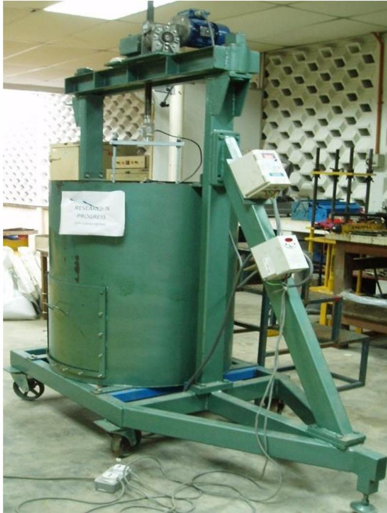
Figure 3.10: Laboratory pullout machine with specially designed wedge and barrel system
