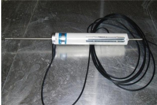
Figure 3.9: LVDT transducer
