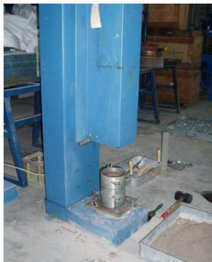
Figure 3.6: The automatic soil compactor
