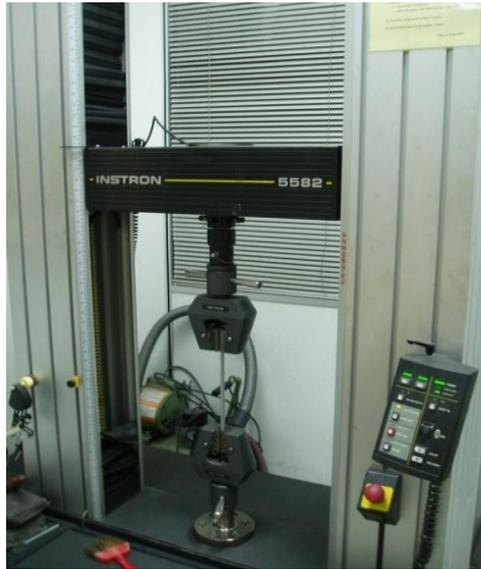
Figure 3.8: Universal Tensile Machine (INSTRON 5582)
