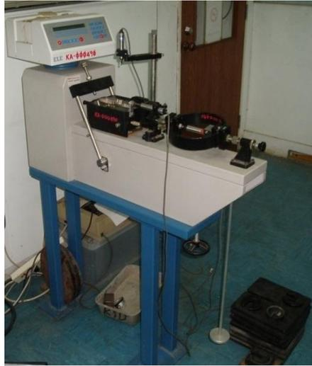
Figure 3.7: Shear box test machine
