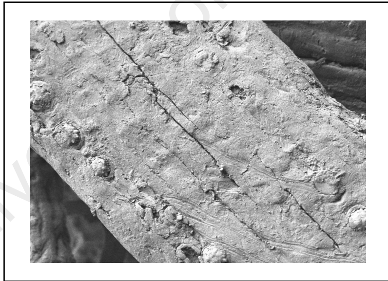
Figure 4.1 Surface View of Oil Palm Fiber at Magnification 500X
