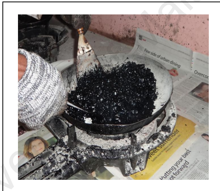
Figure 3.18 Mix the Specimen Coated with Bitumen
