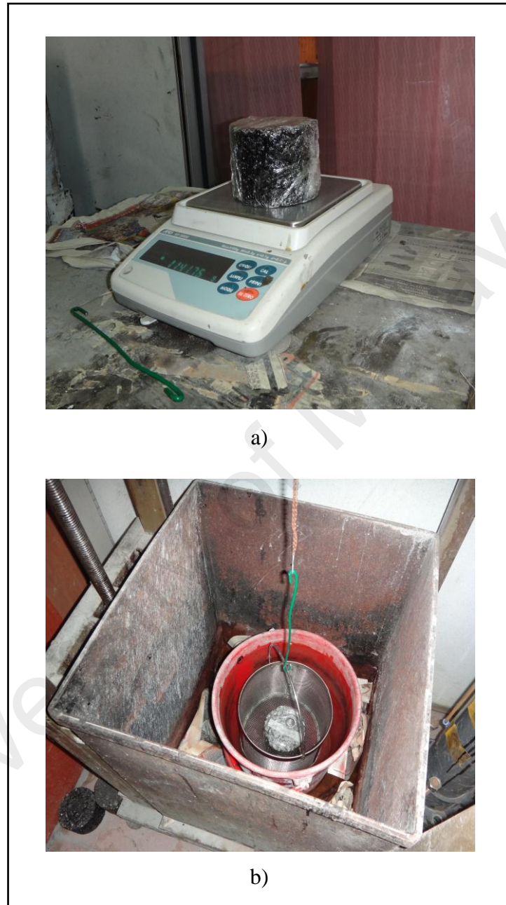
Figure 3.20 a) Specimen Weighted in Air and b) Specimen Weighted in Water
