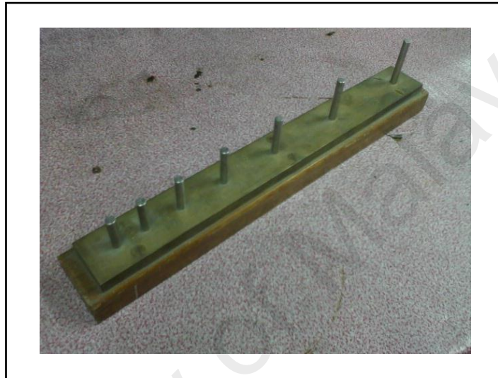
Figure 3.8 Elongation Index Value Equipment
