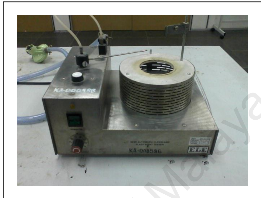
Figure 3.15 Cleveland Open Cup Apparatus (Semi Automatic)
