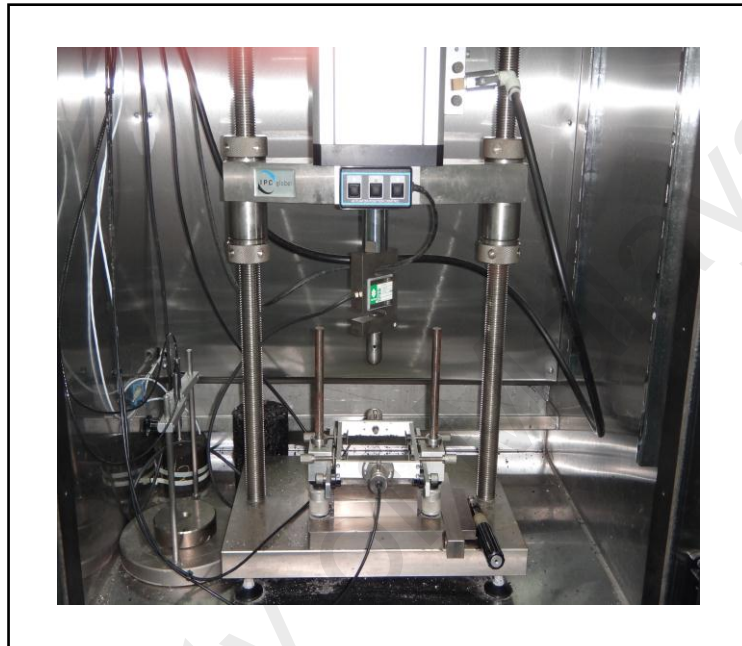
Figure 3.24 Indirect Tensile Stiffness Modulus Test
