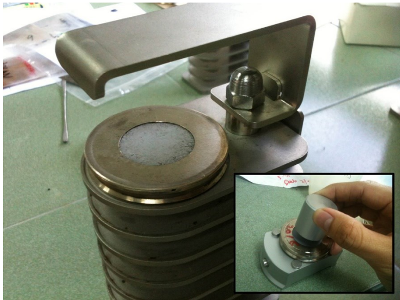
Figure D18: Specimen holder for XRD analysis
