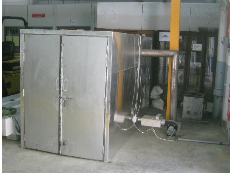
Figure D5: Curing chamber for geopolymer specimens
