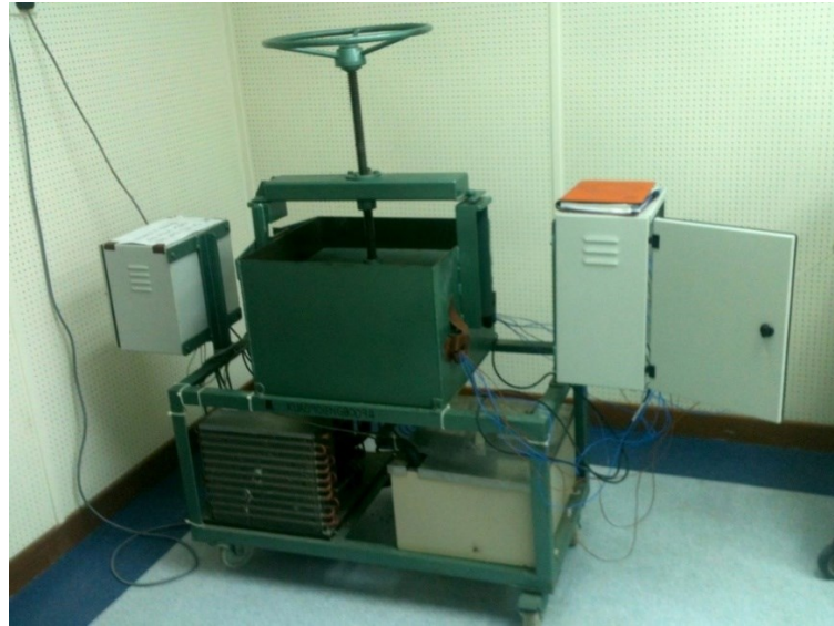
Figure 3.6: Thermal conductivity test equipment
