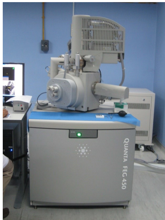
Figure D14: The Quanta FEG 450 and EDX system from Oxford
