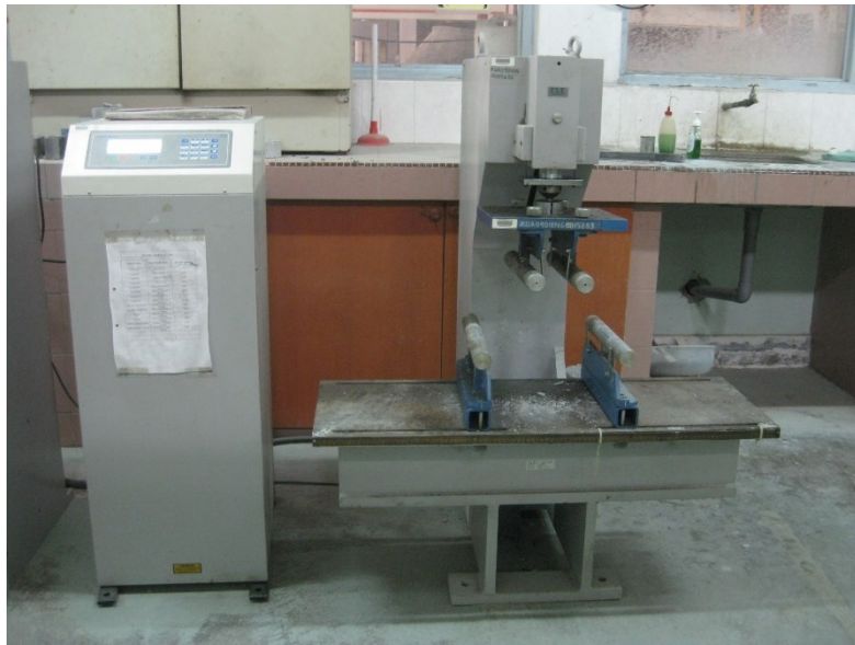
Figure D9: ADR-Auto EL37-6135 standard flexural machine by ELE International
