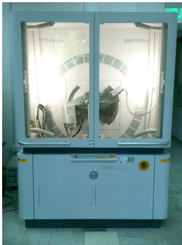
Figure D16: The PANalytical Empyrean diffractometer
