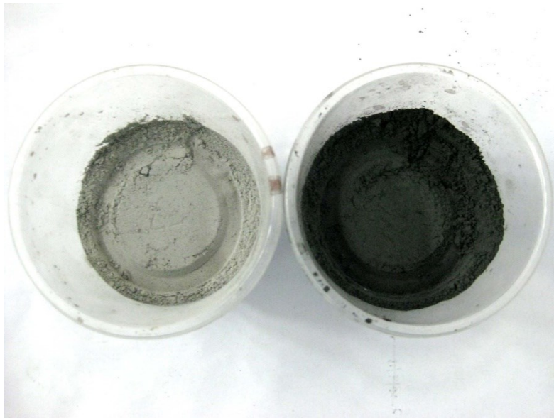
Figure D3: FA and POFA as binder of geopolymer concrete
