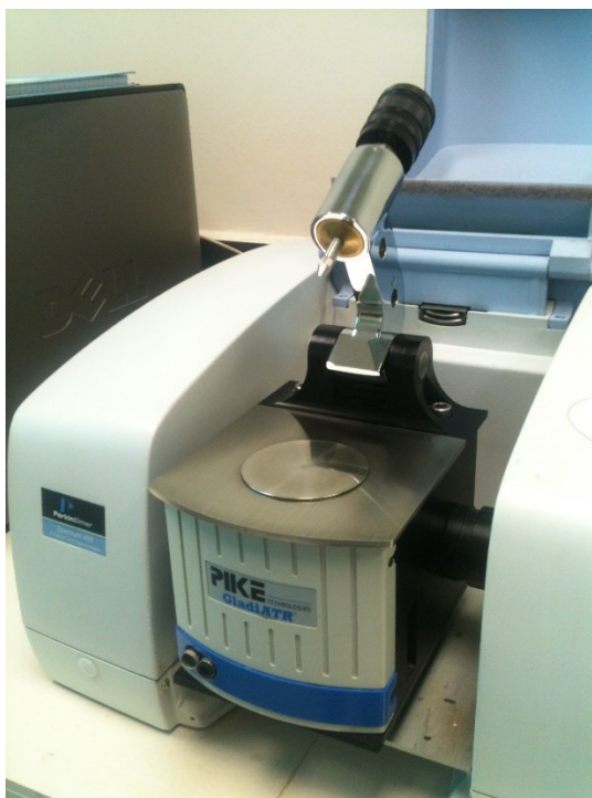
Figure D19: The Perkin Elmer Spectrum 400 spectrometer
