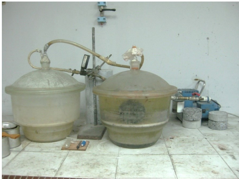
Figure D12: Test set-up for the porosity of geopolymer concrete
