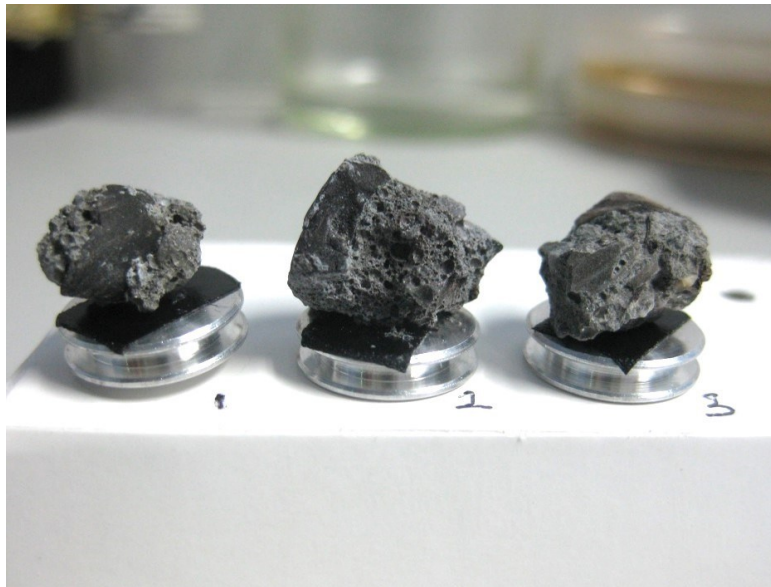
Figure D15: Placement of OPSGC specimens on stub with carbon tape
