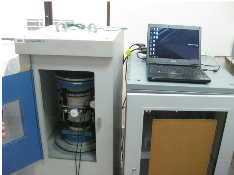
Figure D10: MOE test set up for geopolymer concrete
