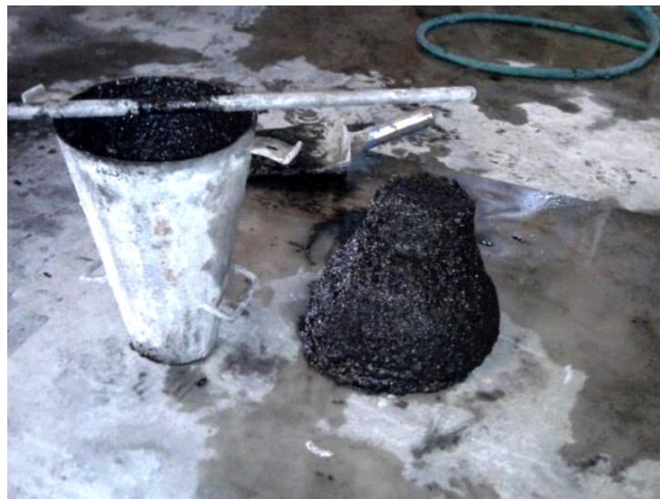
Figure 3.4: Slump measurement of fresh geopolymer concrete
