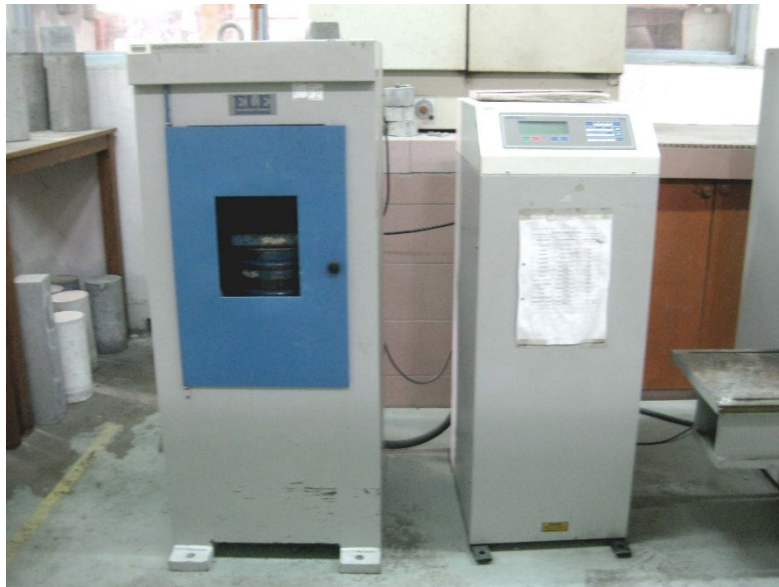
Figure D7: ADR-Auto 2000 standard compression machine by ELE International
