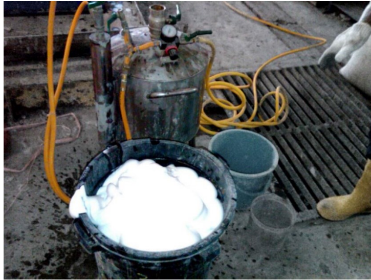
Figure 3.2: Foaming generator and stable foam
