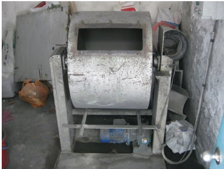
Figure D2: The LA abrasion machine used to ground POFA
