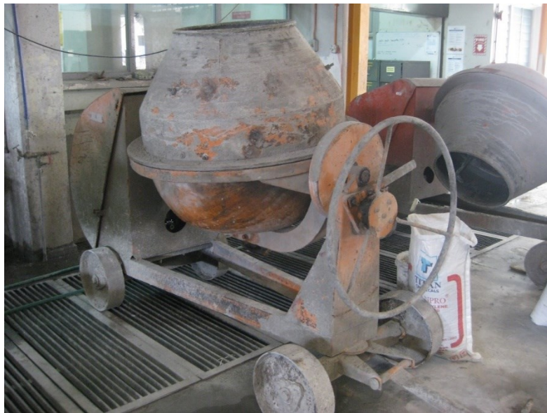
Figure D4: Rotary concrete mixer
