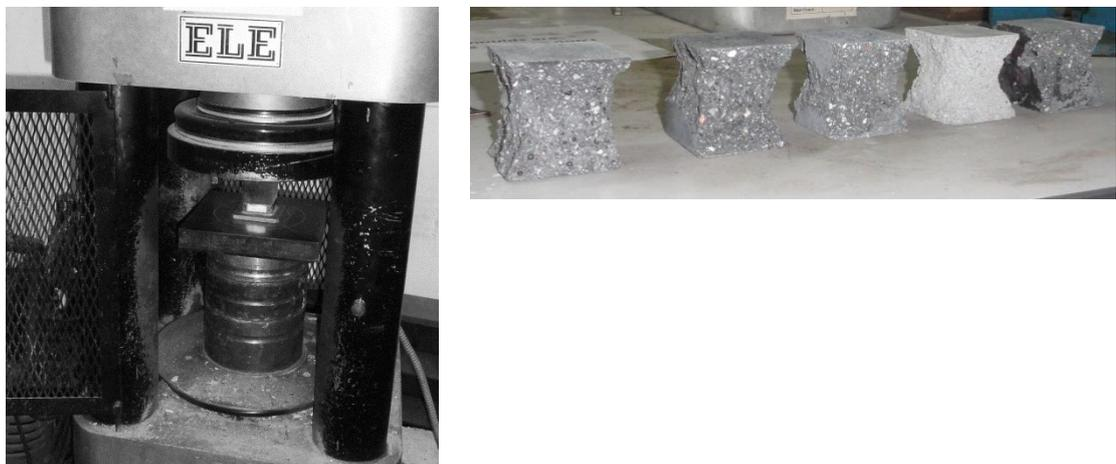
Figure 3.15: Compression testing machine and failure mode of cubes
