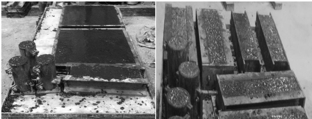
Figure 3.11: Casting specimens for impact test, compressive strength, splitting tensile strength, flexural strength and Young's modulus test
