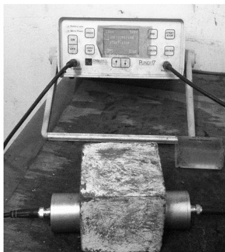
Figure 3.16: Measurement of UPV
