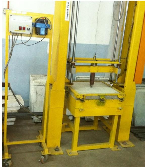
Figure 3.18: Impact test arrangement
