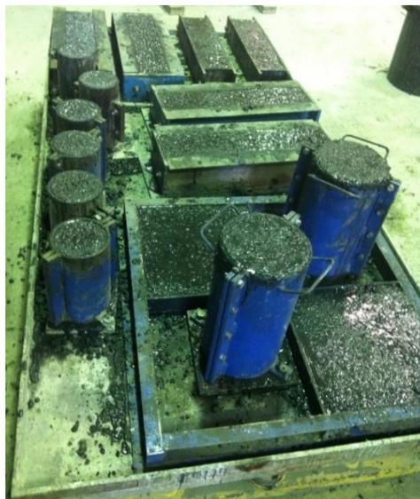
Figure 3.10: Casting specimens for compressive strength, splitting tensile strength, flexural strength and Young's modulus test
