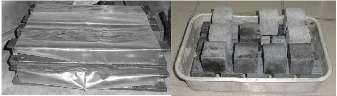
Figure 3.14: Test specimens covered with plastic film and specimens in air drying condition
