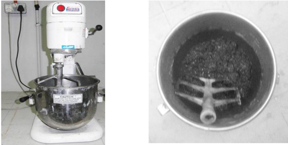
Figure 3.8: Preparation of geopolymer mortar
