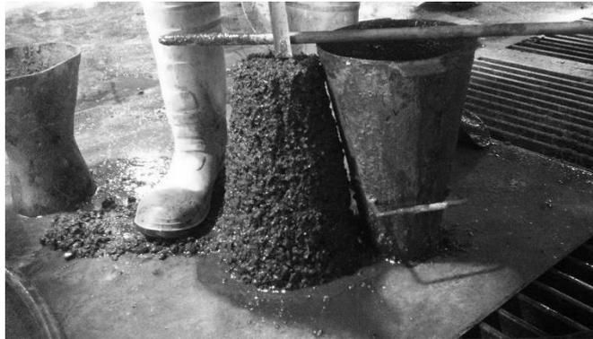
Figure 3.13: Slump test
