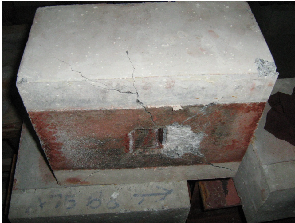
Figure 4.7. Typical fracture of angle shear connector for specimen with high strength concrete (Fractured angle in slab)
