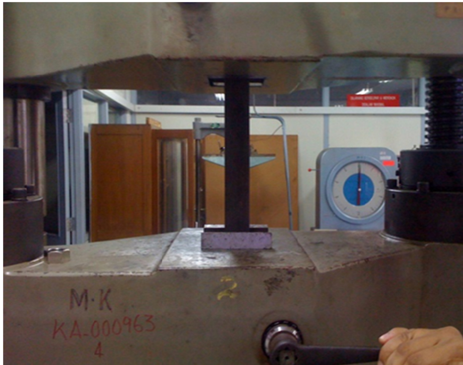
Figure. B.6. Specimen's installation for tensile testing
