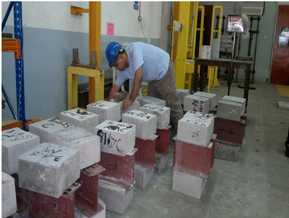
Figure. A.6. Specimens ready for push-out test
