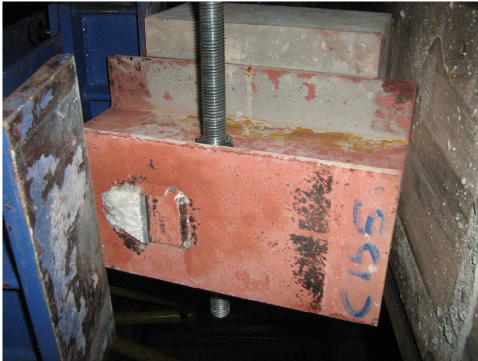
Figure 4.4. Connector fracture of failure
