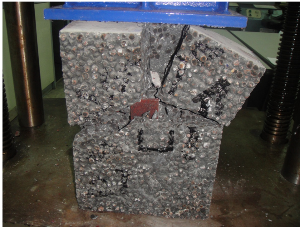
Figure 4.5. Failure of concrete crushing splitting
