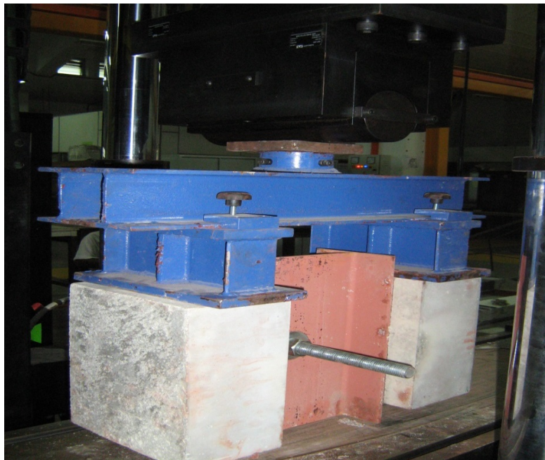
Figure 3.4. Specific support used for loading the slabs
