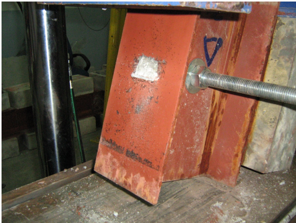
Figure 4.8. Typical fracture of angle shear connector for specimen with high strength concrete (Fractured angle attached to steel I beam)
