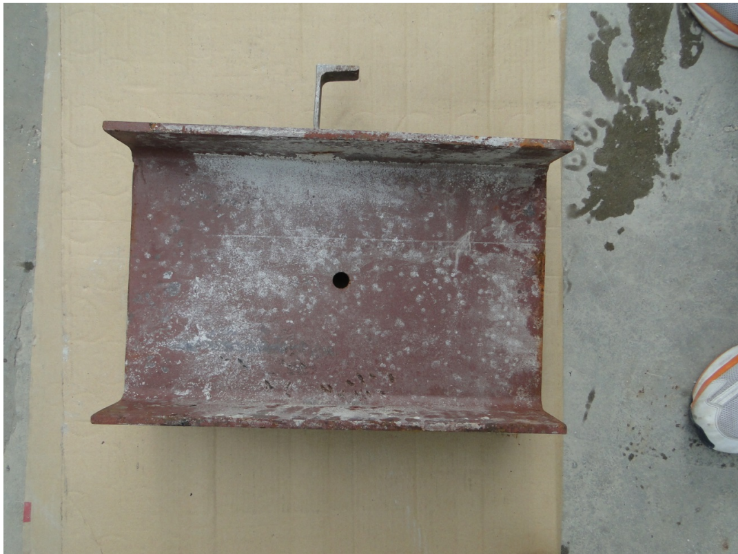
Figure 4.6. Combined failure mode of concrete and connector
