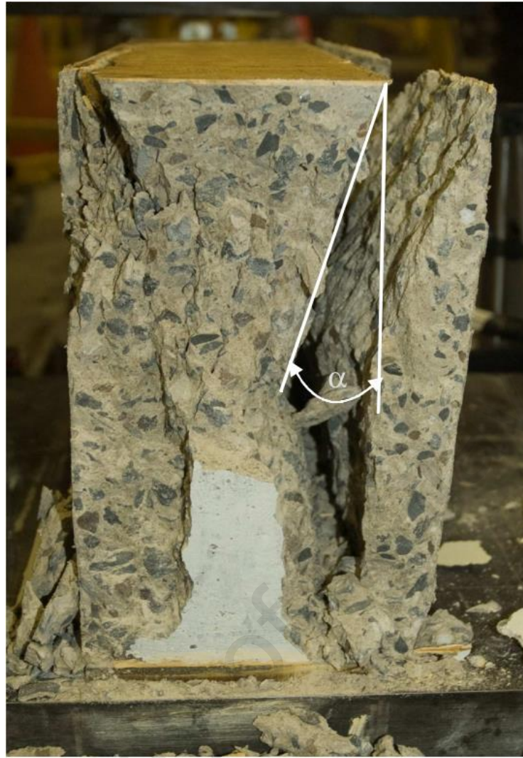
Figure 2.4: Concrete Wedge on Prism Specimen (Nurwidayati, 2011).
