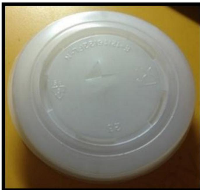
Figure 3.2: Polystyrene cup lids employed as PS waste precursor
