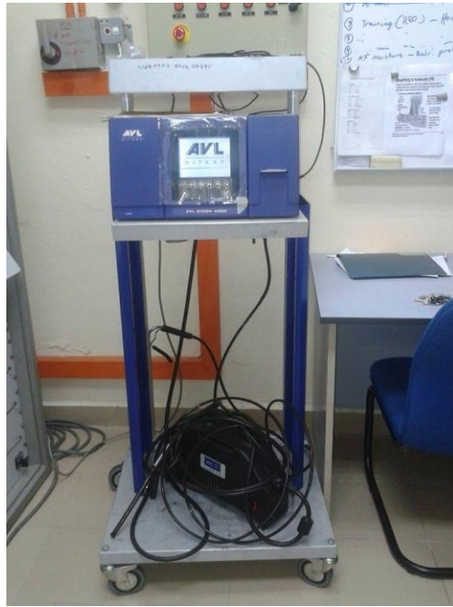
Figure 3.4: AVL DECOM 4000 emission analyzer
