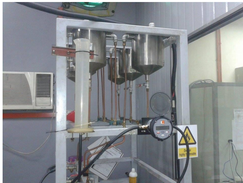
Figure 3.3: Fuel tank with KOBOLD fuel flow meter
