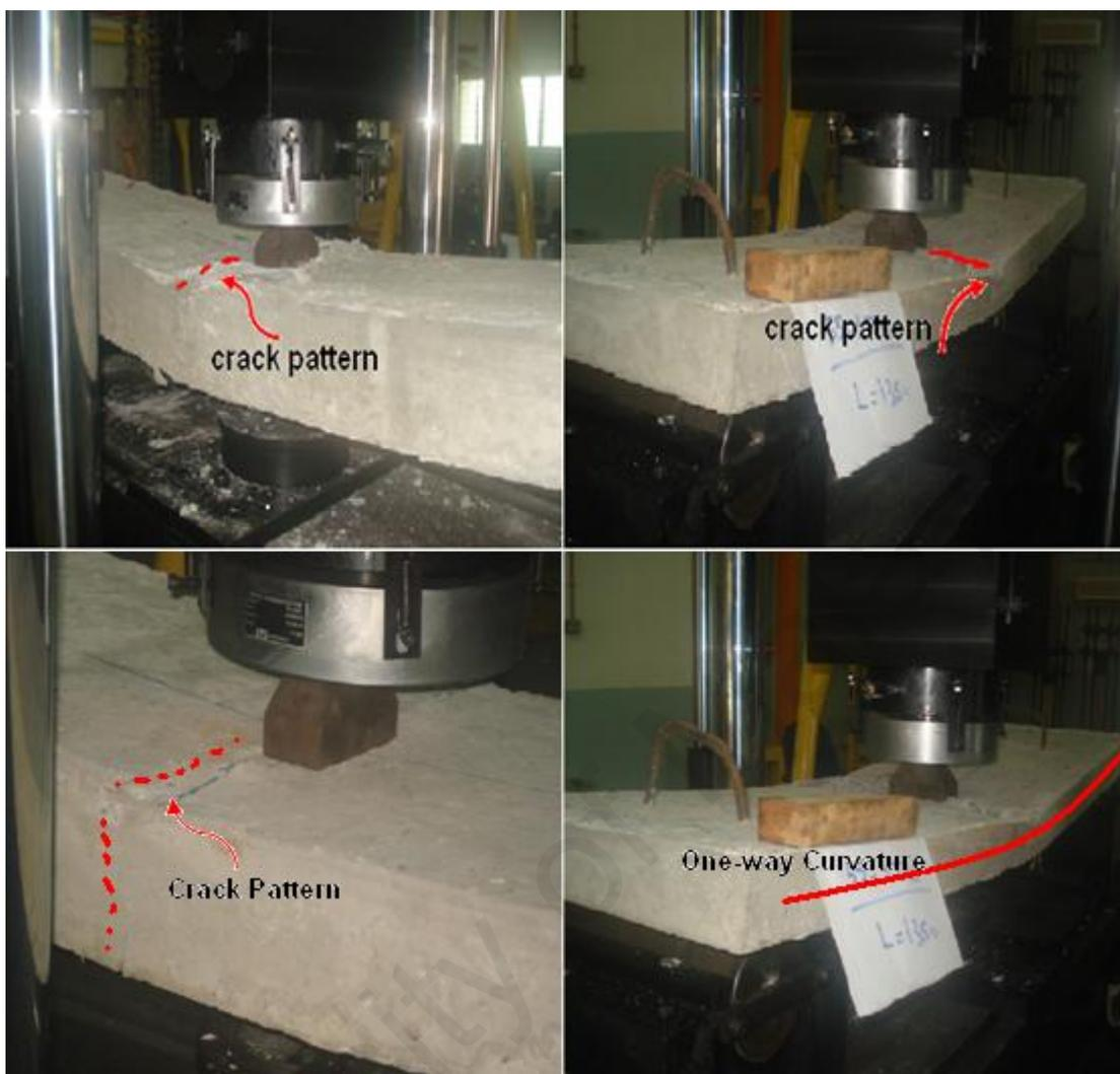
Figure 3.5: Experimental crack pattern of the non-strengthened RC slab under mid-span punching load
