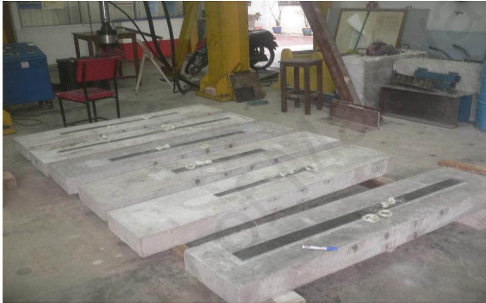
Figure 6.17: RC one-way slab strengthened by different lengths and width of CFRP
