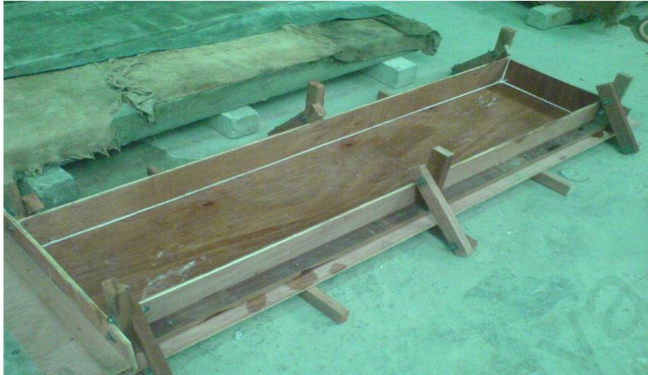
Figure 6.2: The formwork used for casting in the experimental work
