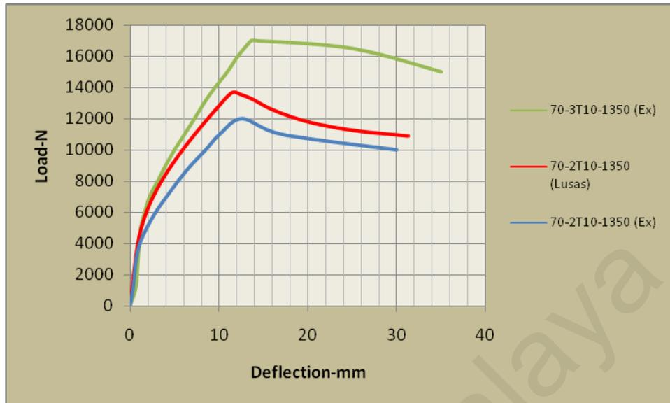
Figure 6.13: The experimental results of load-deflection curve for the samples 70-3T10-1350 and 70-2T10-1350 in compare with LUSAS results
