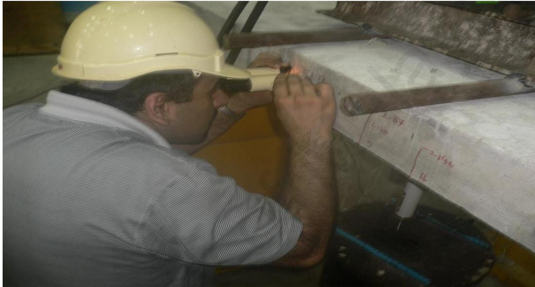
Figure 6.20: Crack measuring in each step of applied loading
