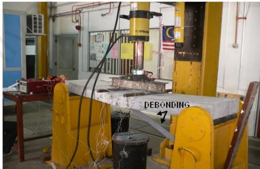
Figure 6.19: CFRP debonding at the CFRP/concrete interface under four point line load
