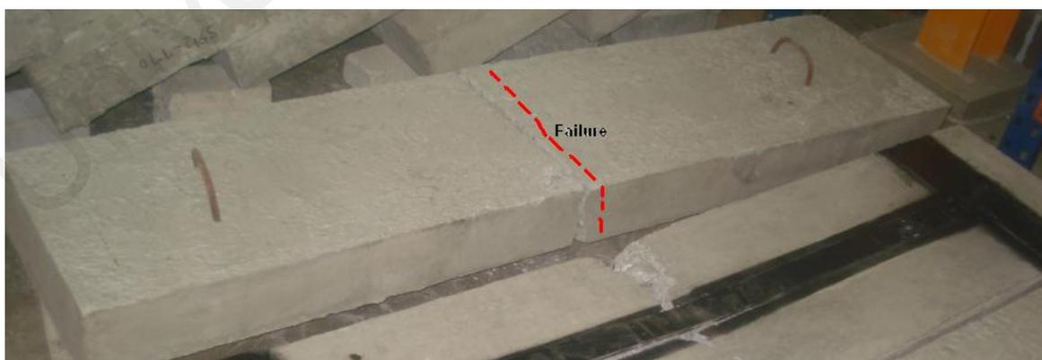
Figure 3.6: Non-strengthened RC slab under mid-span punching load after testing
