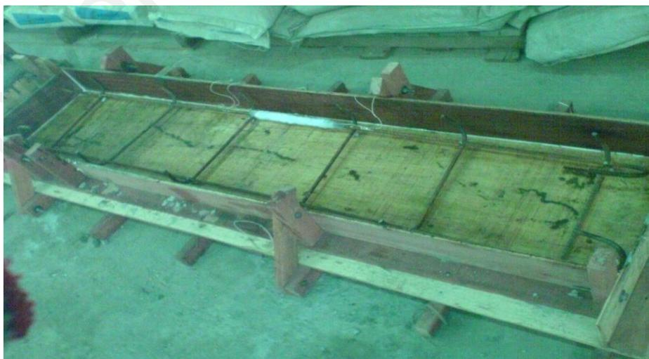
Figure 6.3: The longitudinal reinforcement used for the non-strengthened and CFRP strengthened RC one-way slab
