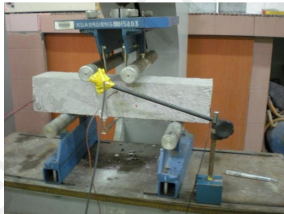
(b) Photograph of loading test for scale-model CB.
