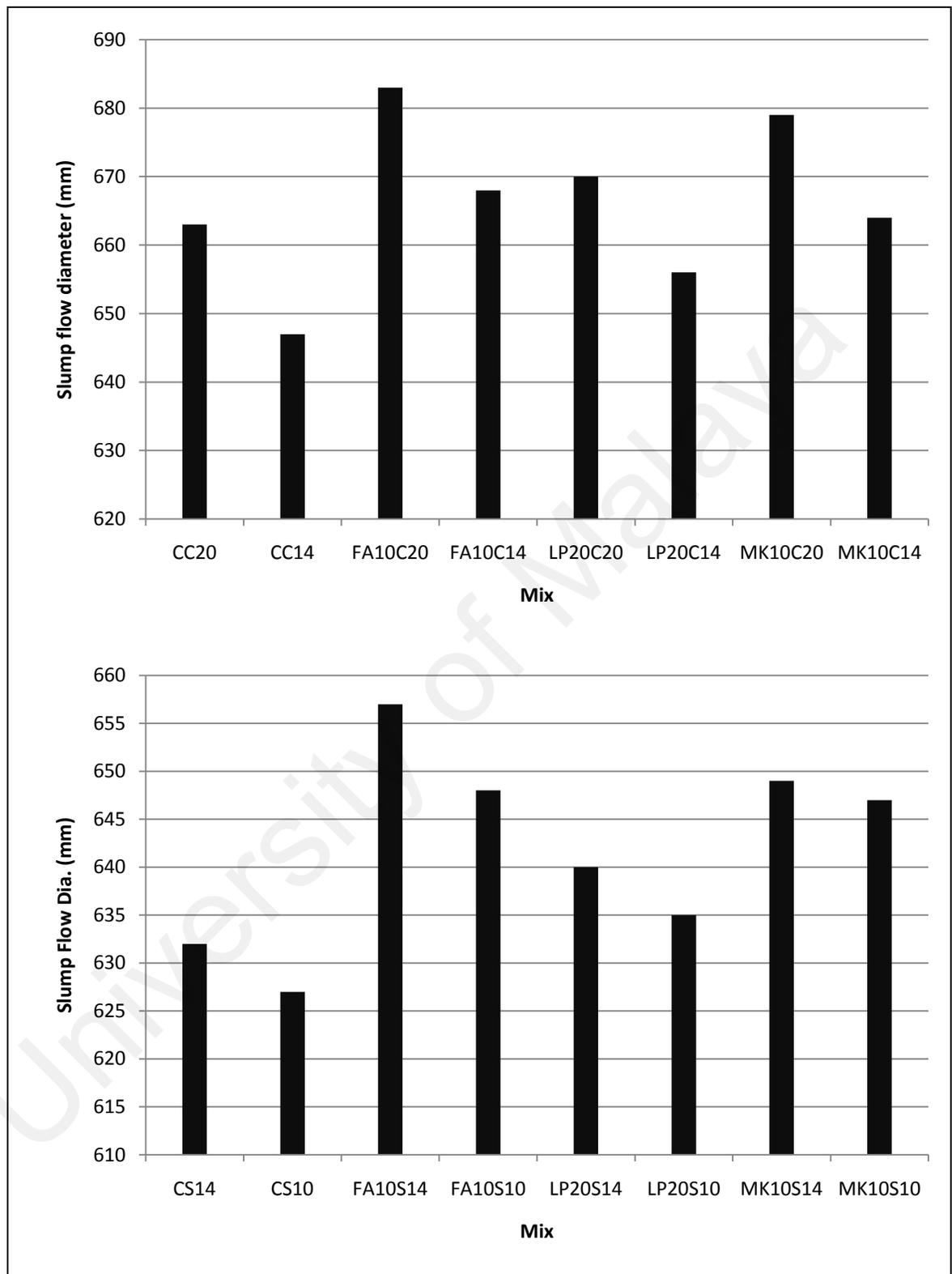
Figure 4.54: Slump flow diameter of different maximum size aggregate mixes
