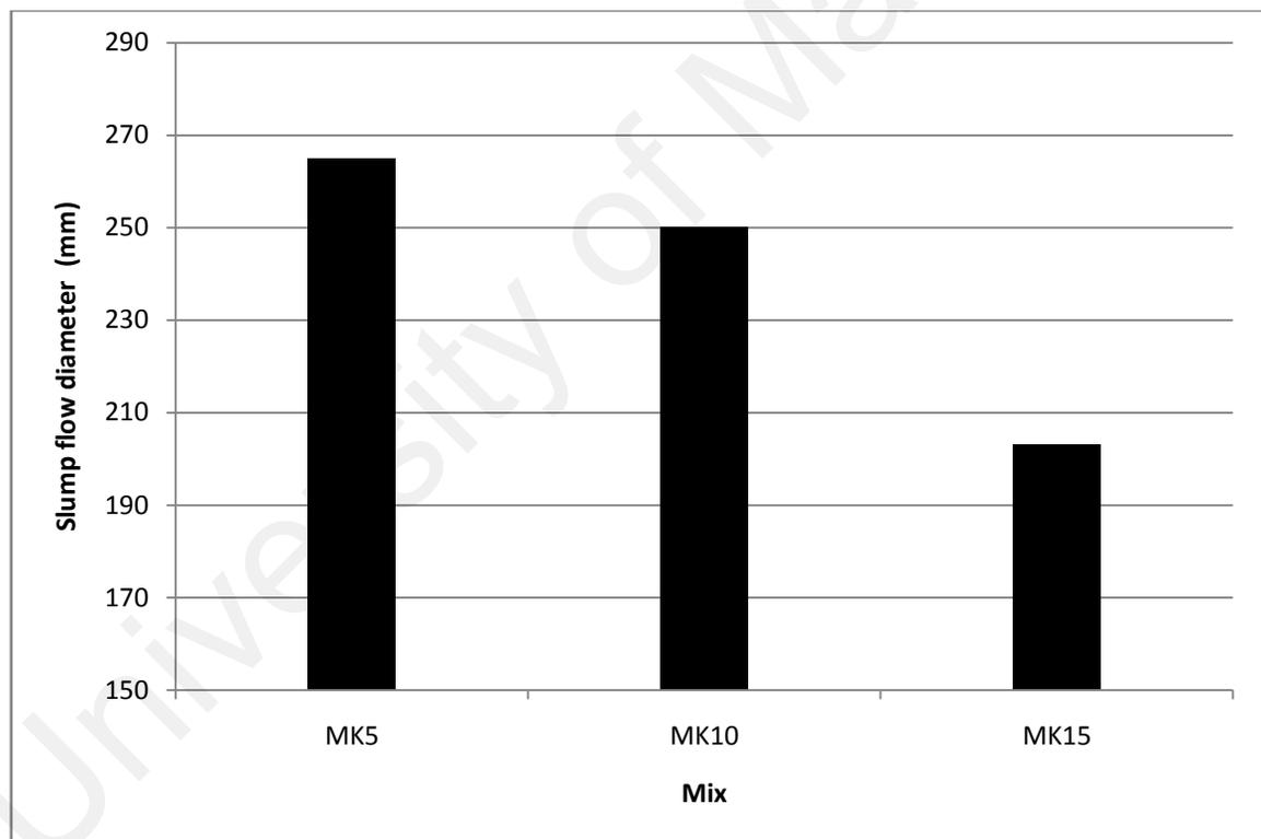
Figure 4.11: Slump flow diameter of metakaolin mixes with same w/p ratio and superplasticizer dosage
