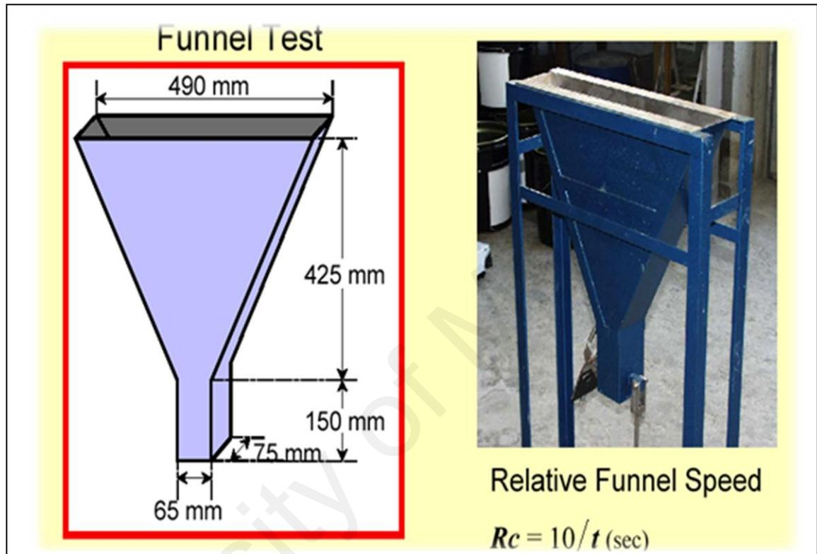
Figure 3.6: V-Funnel test
