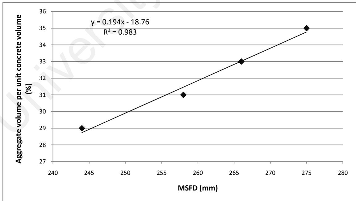
Figure 4.119: Relationship between coarse aggregate volume and MSFD of mortar at SFD of 650 mm for concrete
