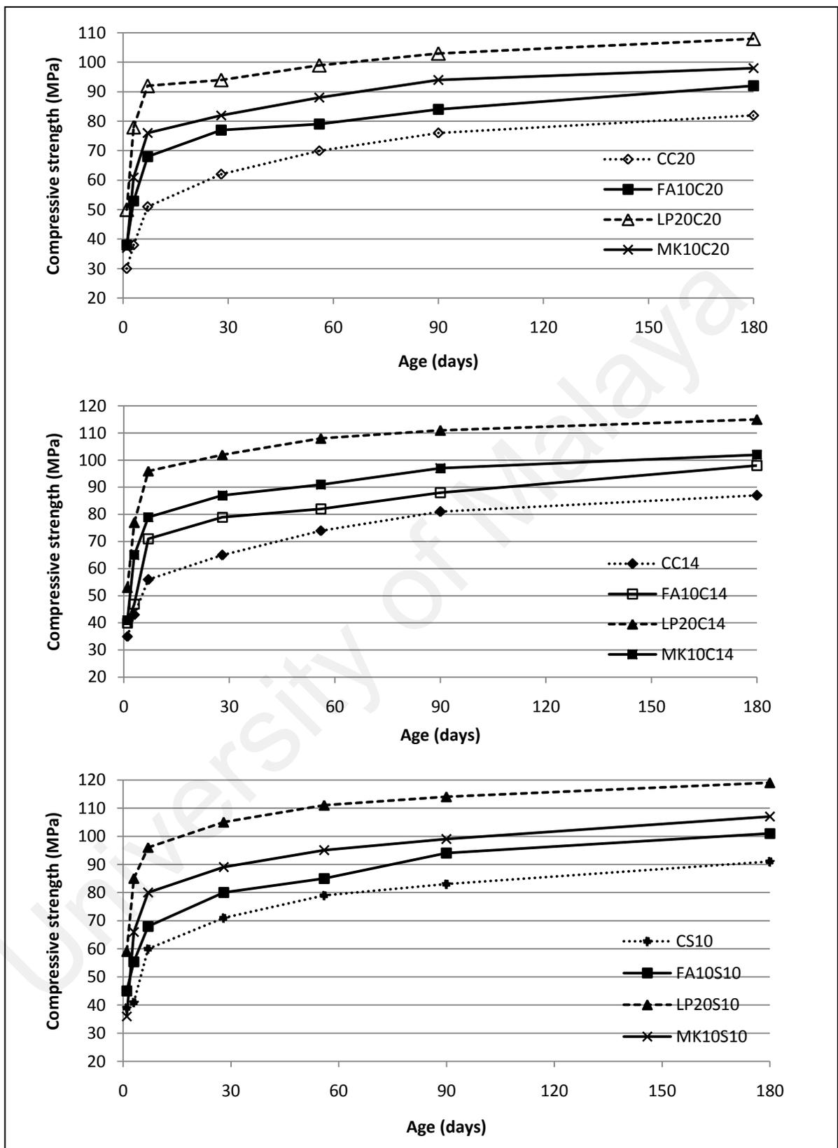
Figure 4.79: Compressive strength development for different mineral admixture mixes
