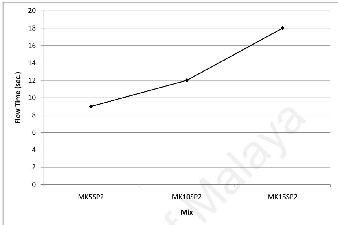
Figure 4.13: Flow time of metakaolin mixes with same w/p ratio and superplasticizer dosage
