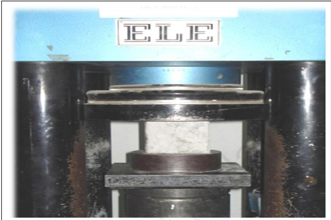
Figure 3.10: Compressive strength test
