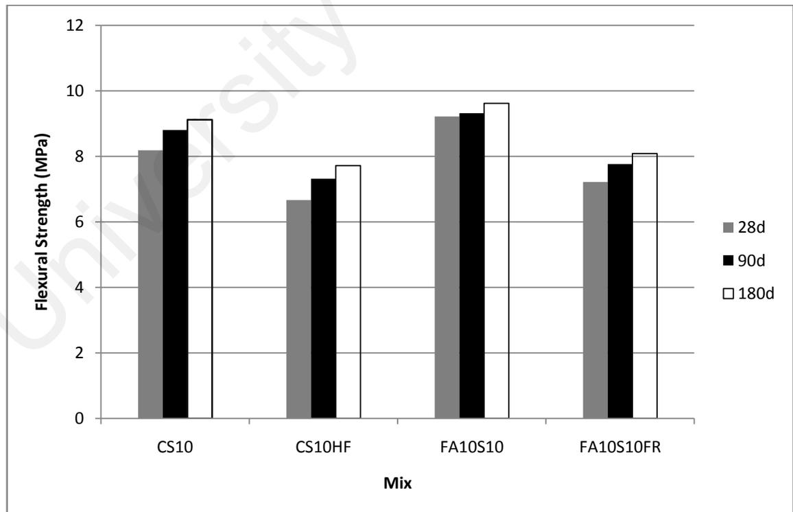
Figure 4.113: Flexural strength of concretes with different shape aggregate
