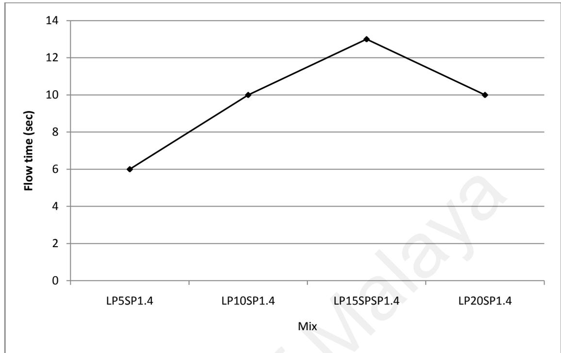
Figure 4.20: Flow time of limestone mixes with same w/p ratio and superplasticizer dosage
