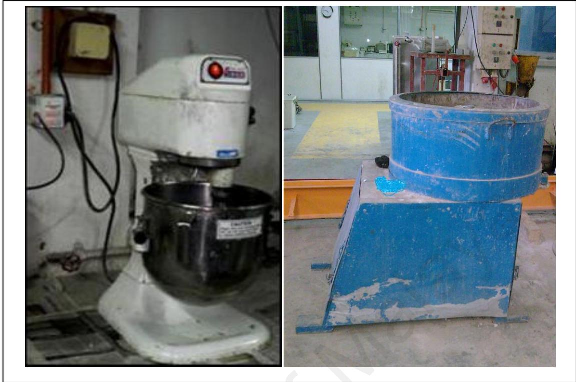
Figure 3.2: Bowl mixer for mortar (left) and pan mixer for concrete (right)
