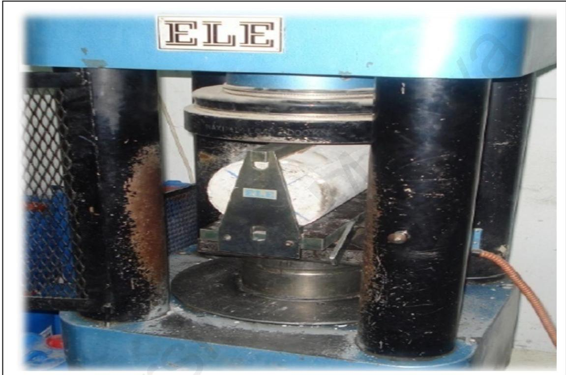
Figure 3.11: Splitting tensile strength test
