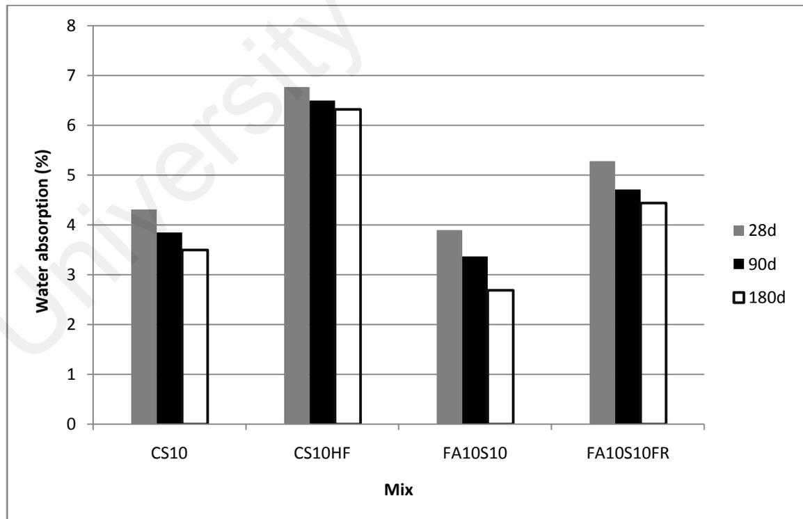
Figure 4.115: Water absorption of concretes with different shaped aggregate
