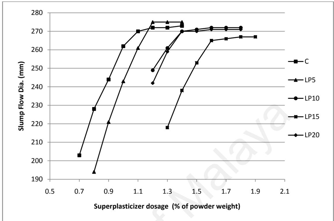
Figure 4.16: Optimum superplasticizer dosage of control and limestone mixes
