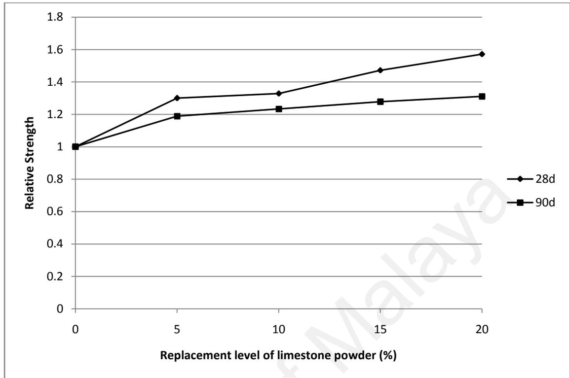
Figure 4.31: Relative strength of limestone mixes at 28 and 90 days
