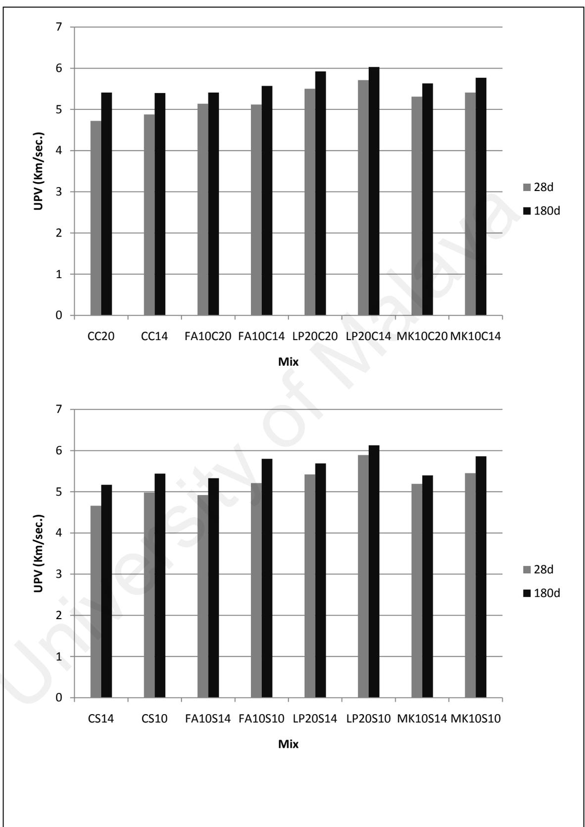
Figure 4.103: UPV values of concretes with different maximum size aggregate
