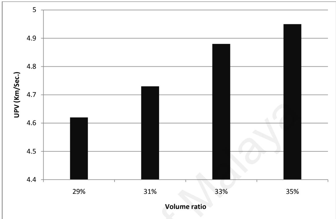
Figure 4.96: UPV of different aggregate ratios
