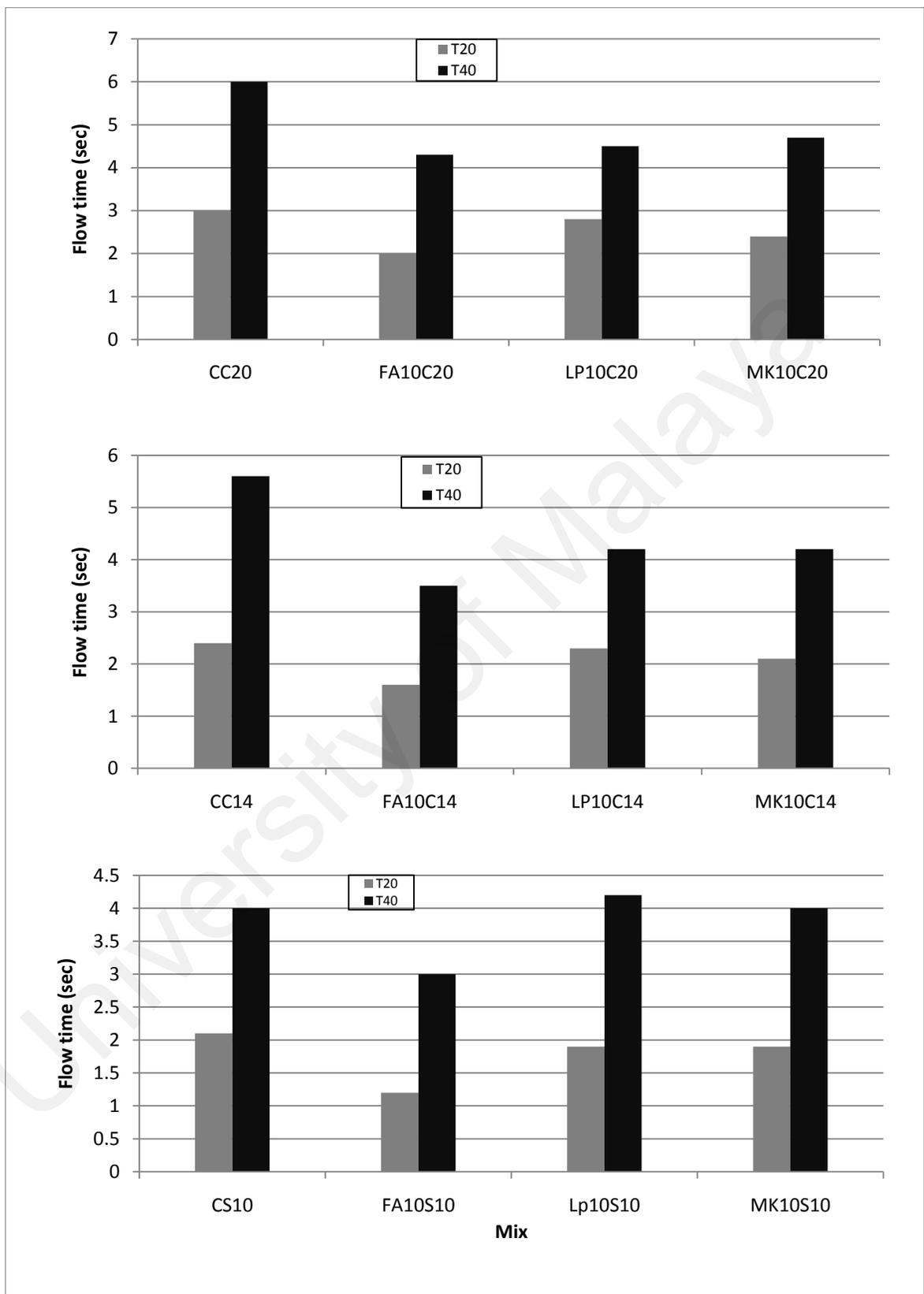
Figure 4.43: Flow times at 20 and 40 mm in L-box test of mixes with different mineral admixtures
