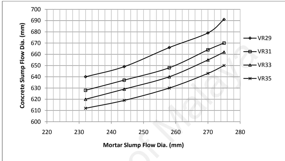
Figure 4.118: The relationship between SFD of mortars and concretes with different aggregate content
