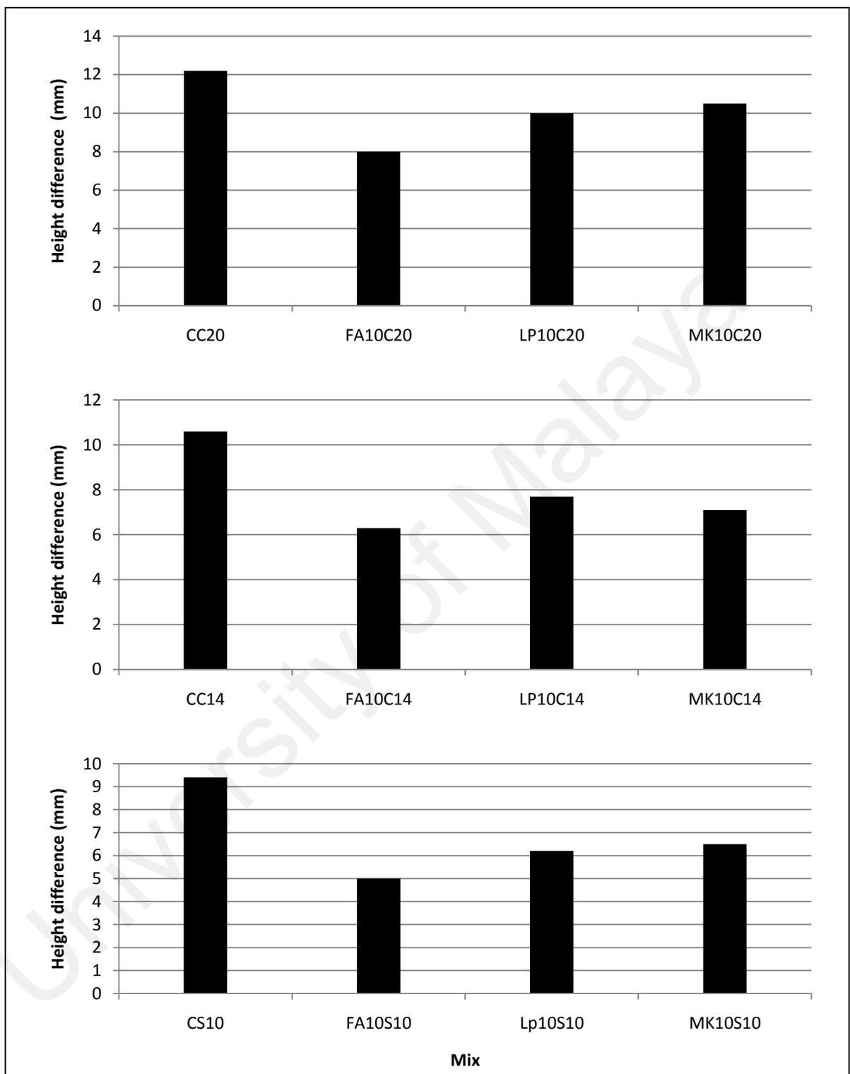
Figure 4.45: Height difference ( $\Delta H$ ) of mixes with different mineral admixtures
