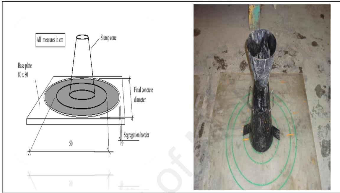
Figure 3.5: Slump Flow Test
