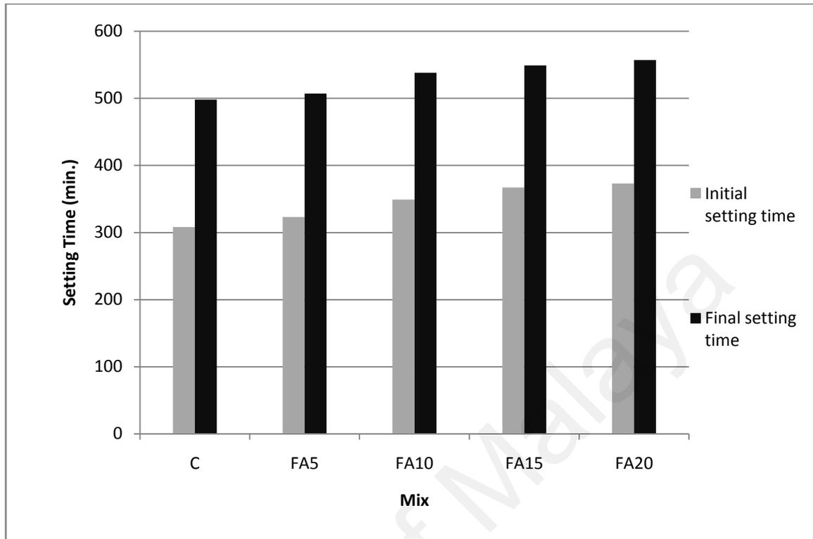
Figure 4.14: Initial and final setting time of control and fly ash mixes
