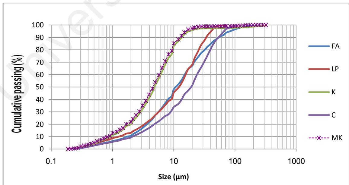
Figure 4.1: Particle size distribution of powders
