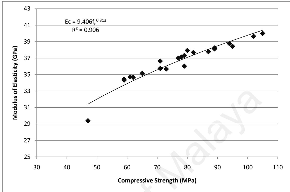
Figure 4.126: Relationship between modulus of elasticity and compressive strength of HSSCC
