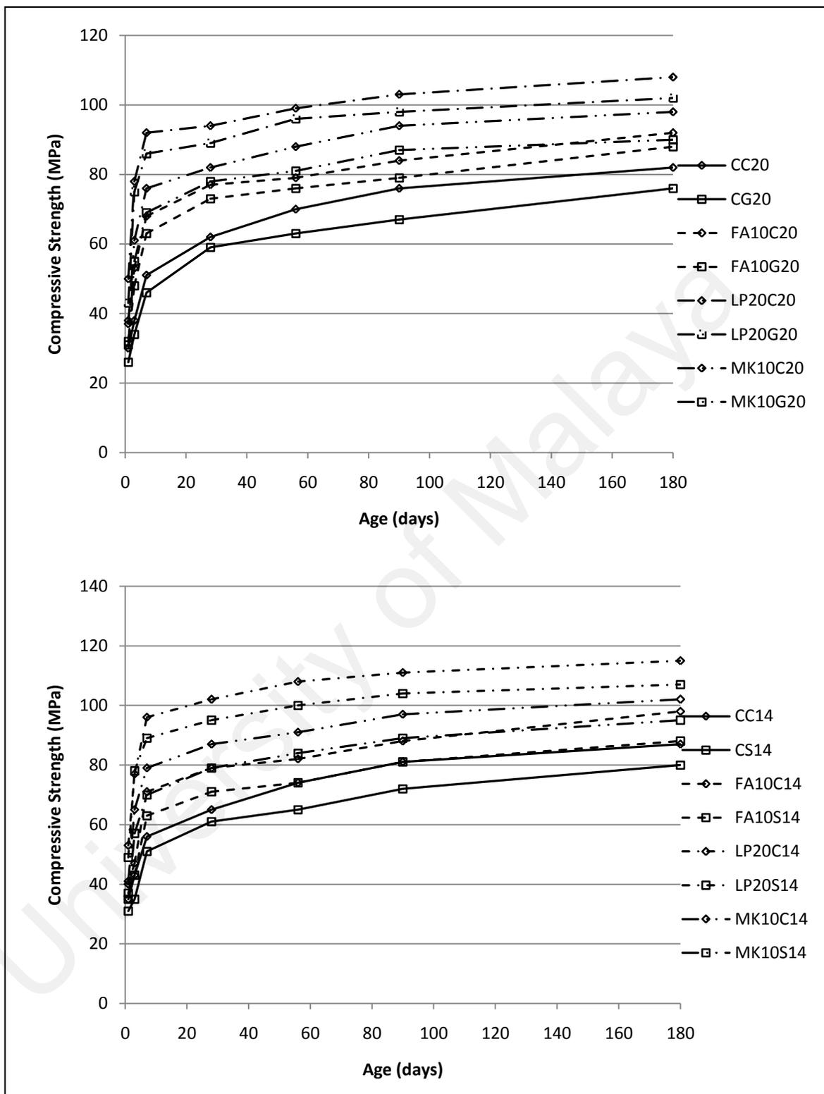
Figure 4.104: Compressive strength of concretes with different grade aggregate
