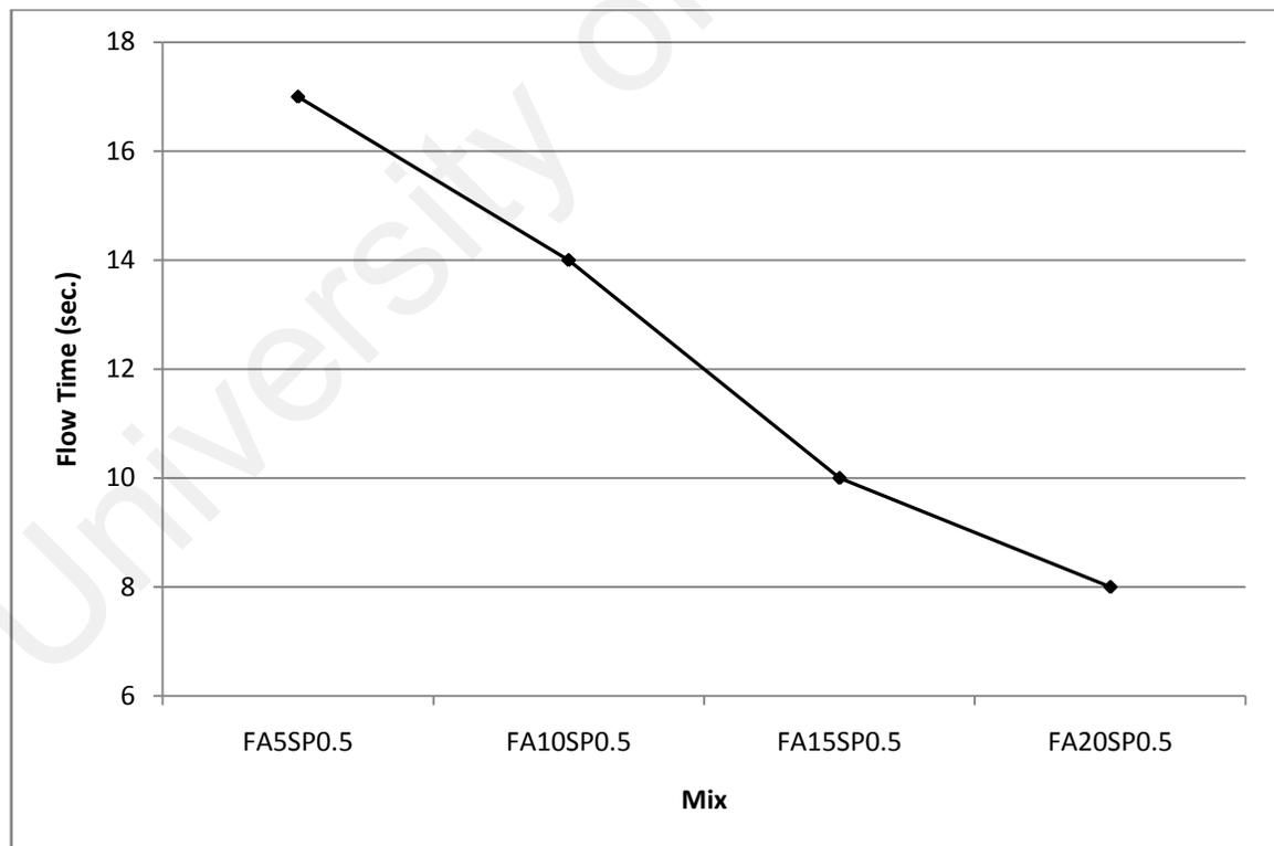
Figure 4.12: Flow time of fly ash mixes with same w/p ratio and superplasticizer dosage
