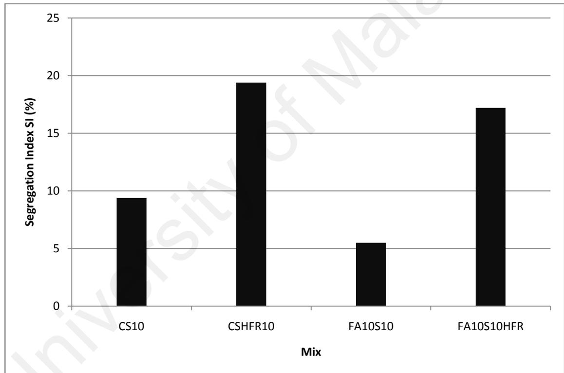
Figure 4.77: Segregation index of different shape aggregate concretes
