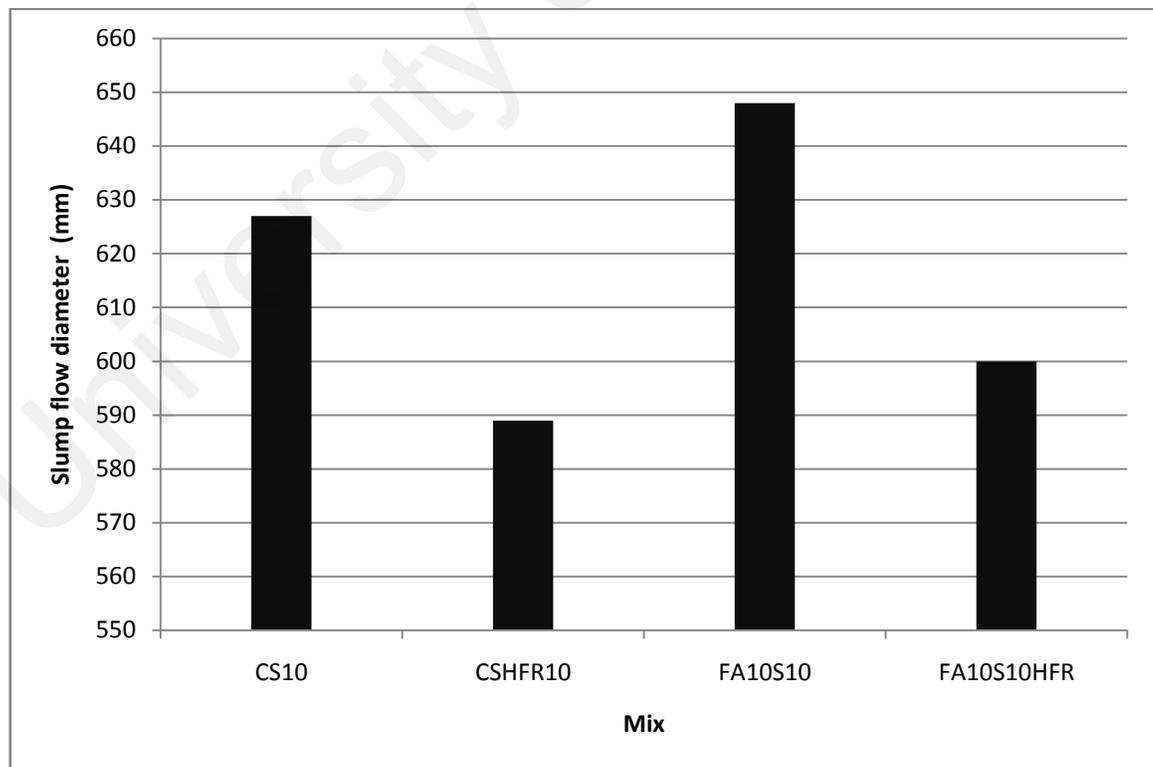
Figure 4.70: Slump flow diameter of different shape of aggregate concrete mixes
