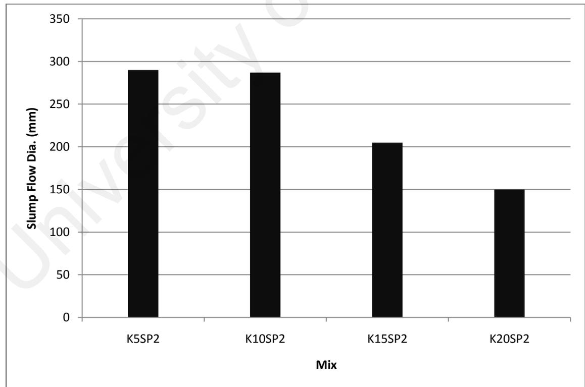
Figure 4.19: Flow spread of kaolin mixes with same w/p ratio and superplasticizer dosage
