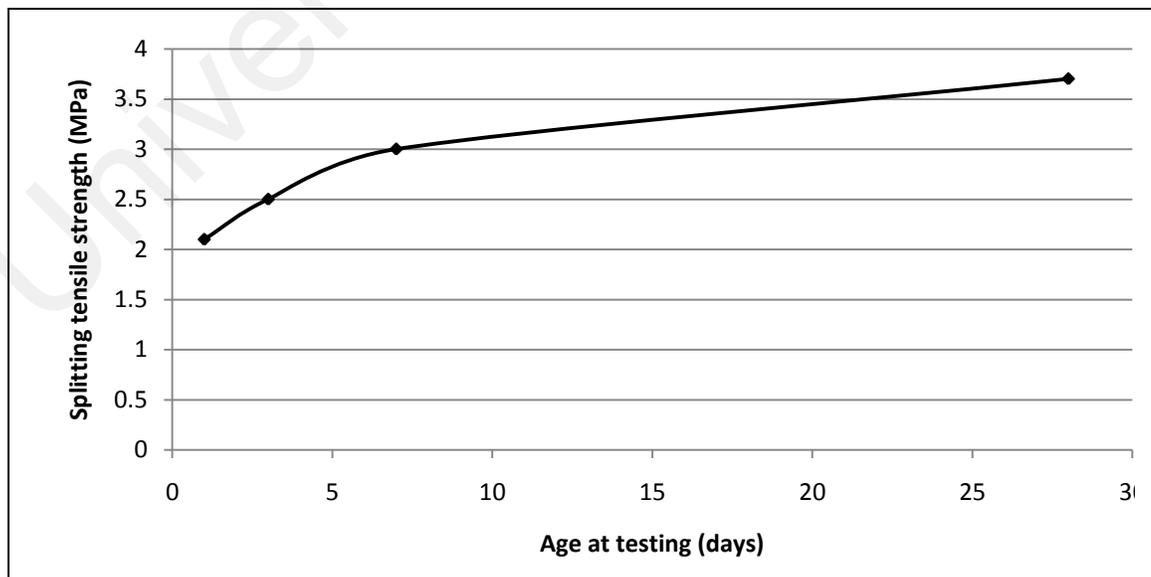
Figure 2.11: Time development of the splitting tensile strength of SCC (Dehn et al., 2000)
