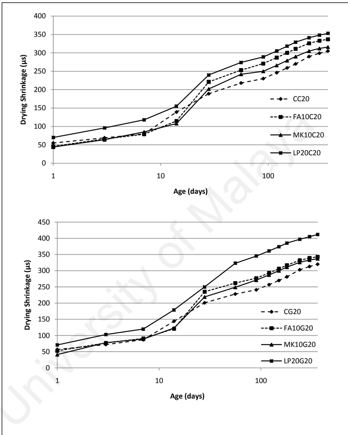
Figure 4.87: Drying shrinkage of different mineral admixture mixes
