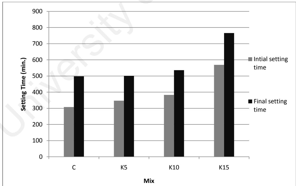
Figure 4.23: Initial and final setting time of K mixes
