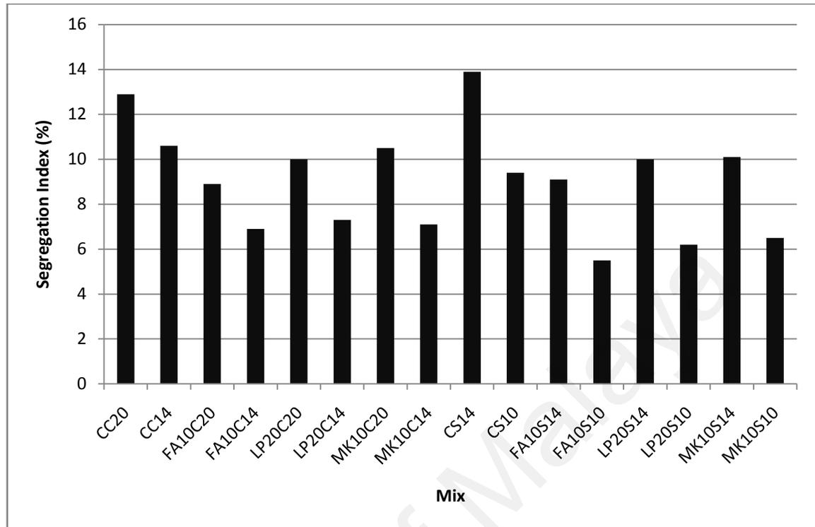
Figure 4.61: Segregation index of different maximum size mixes
