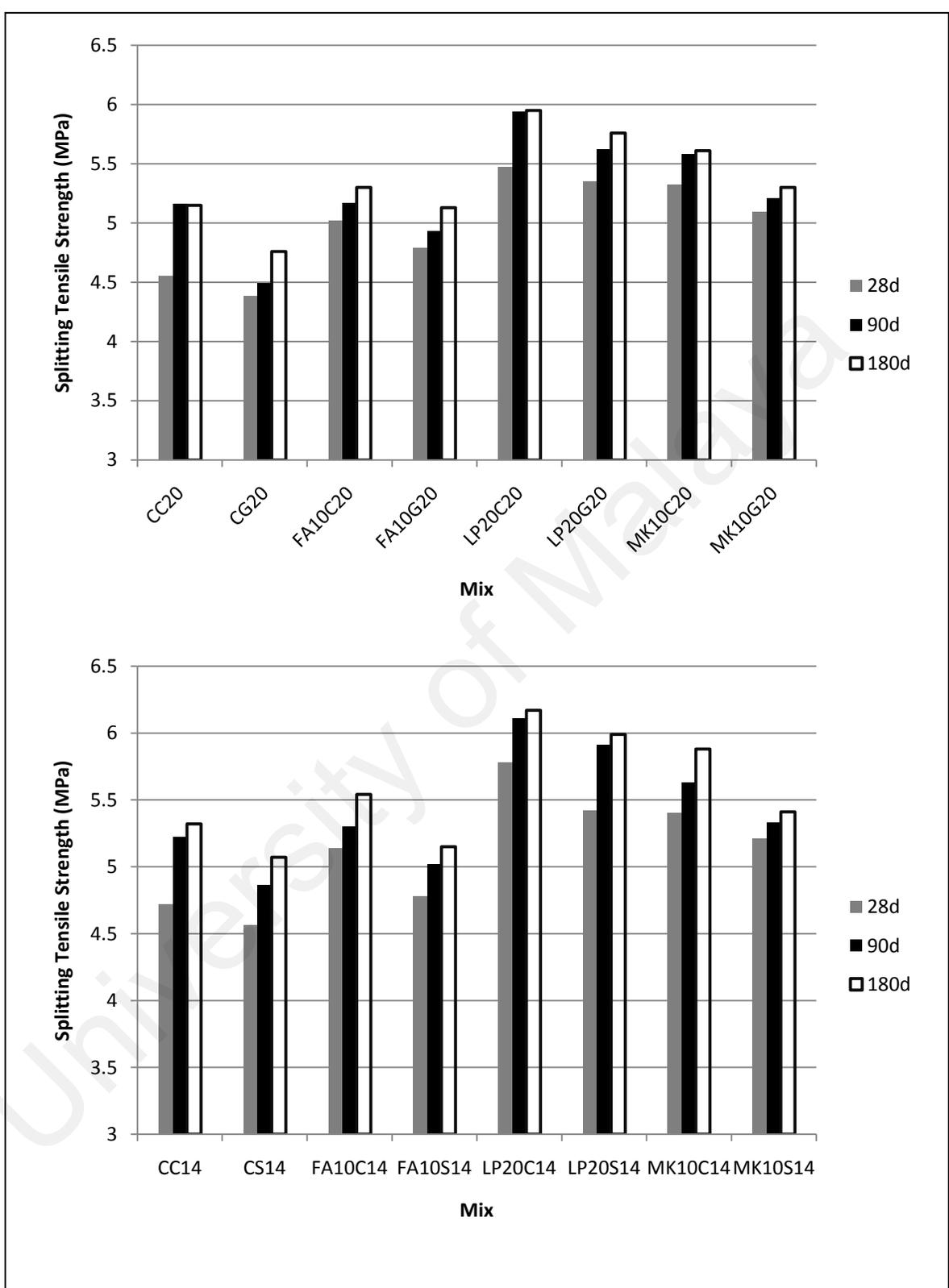
Figure 4.105: Splitting tensile strength of concretes with different grade aggregate
