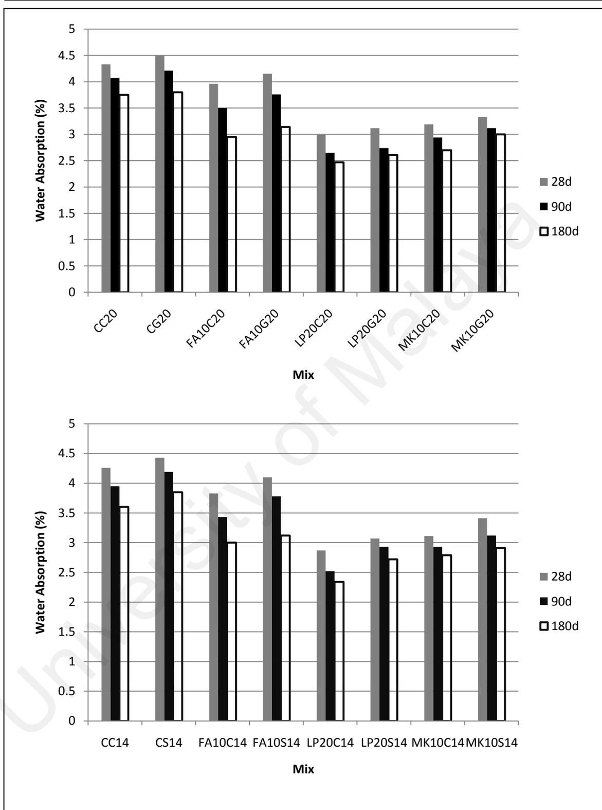
Figure 4.108: Water absorption of concretes with different graded aggregate
