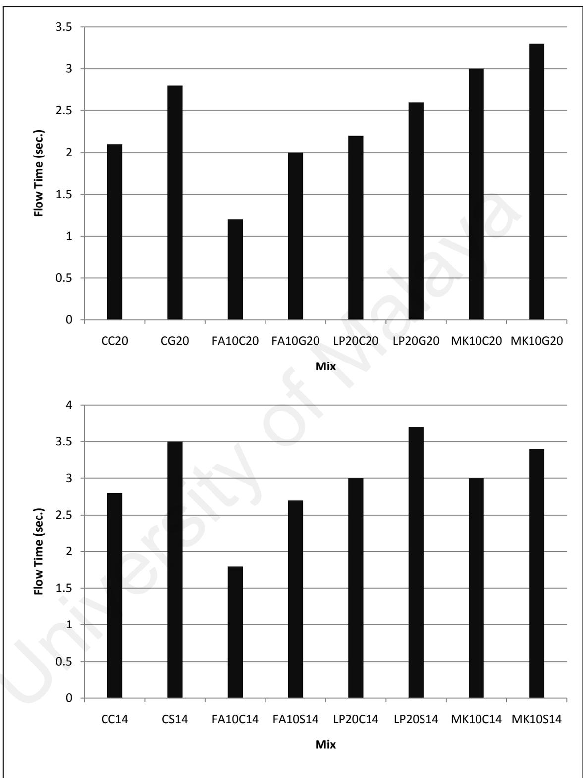
Figure 4.63: Flow time at spread of 50cm of different aggregate grades (graded, gap and single) of mixes
