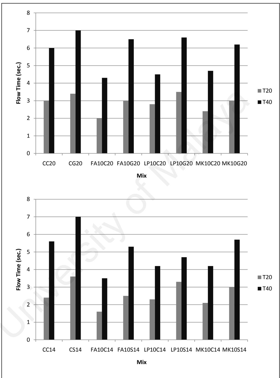
Figure 4.66: T20 & T40 of different aggregate grades (graded and single) of mixes
