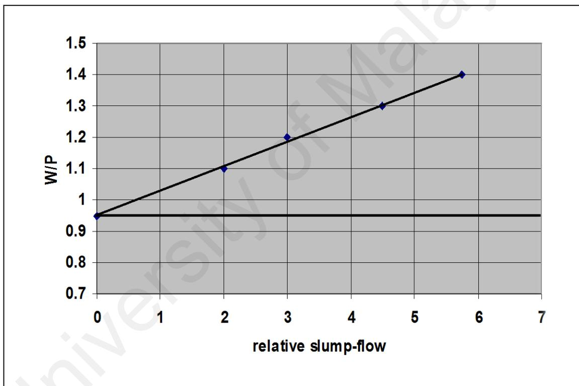
Figure 2.7: Determination of water to powder ratio  $\beta_p$  (EFNARC, 2002)
