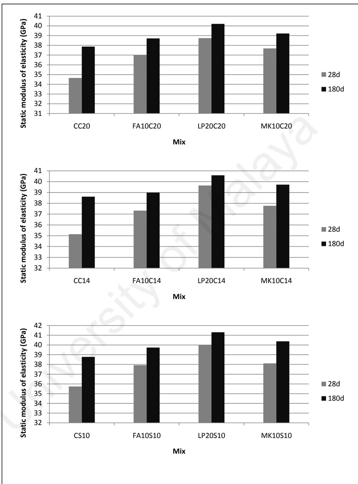
Figure 4.84: Modulus of elasticity of different mineral admixture mixes
