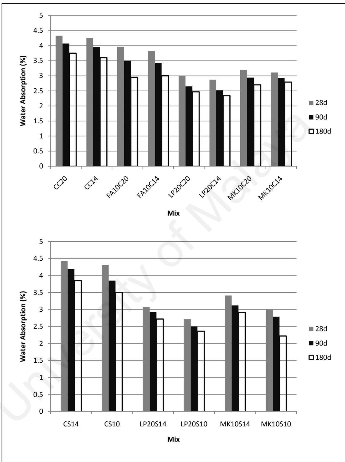
Figure 4.101: Water absorption of concretes with different maximum size aggregate
