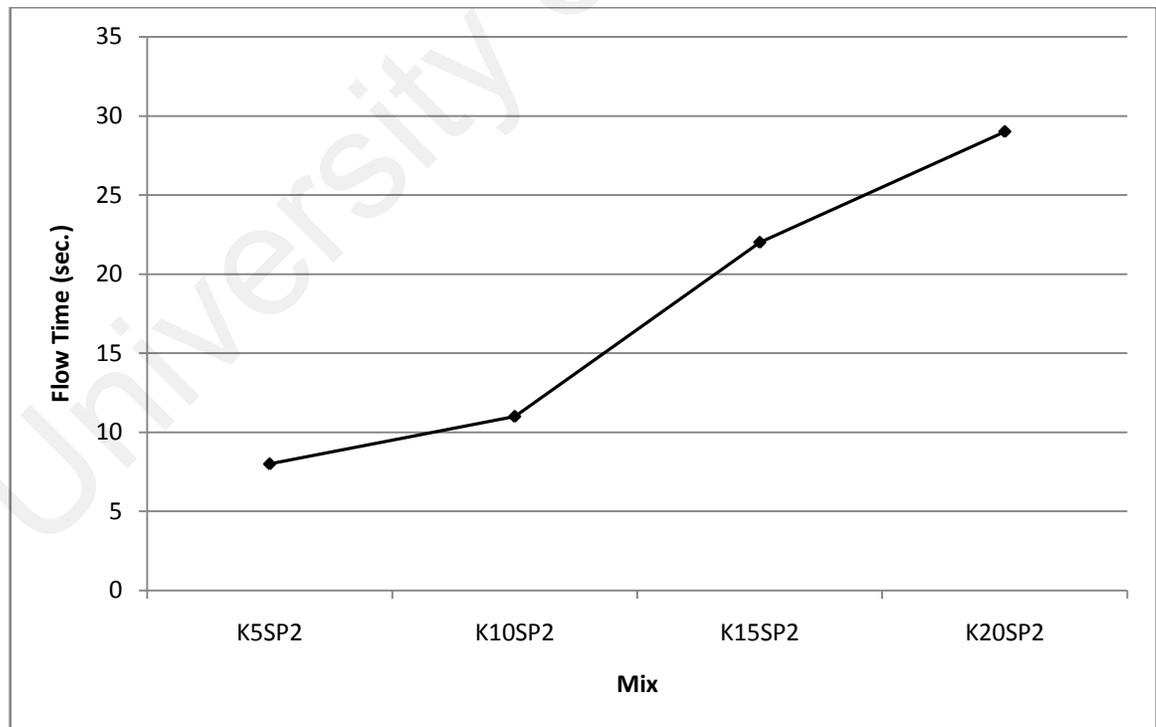
Figure 4.21: Flow time of kaolin mixes with same w/p ratio and superplasticizer dosage.
