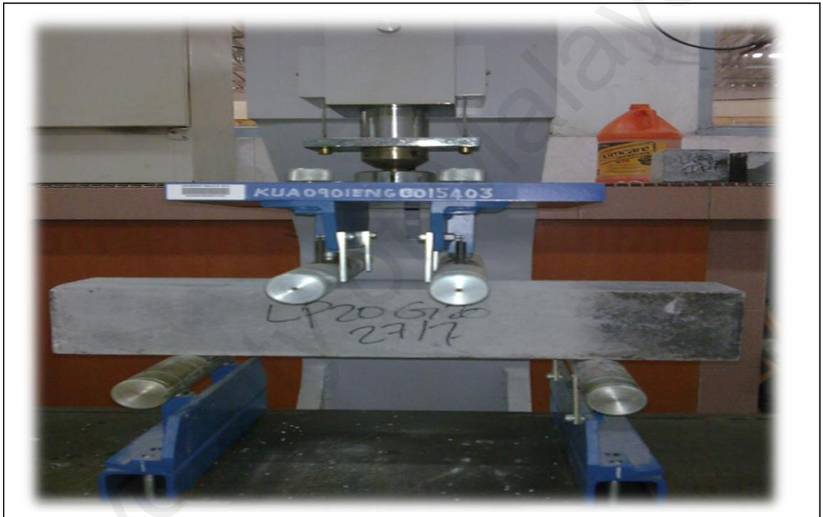
Figure: 3.12: Flexural strength test
