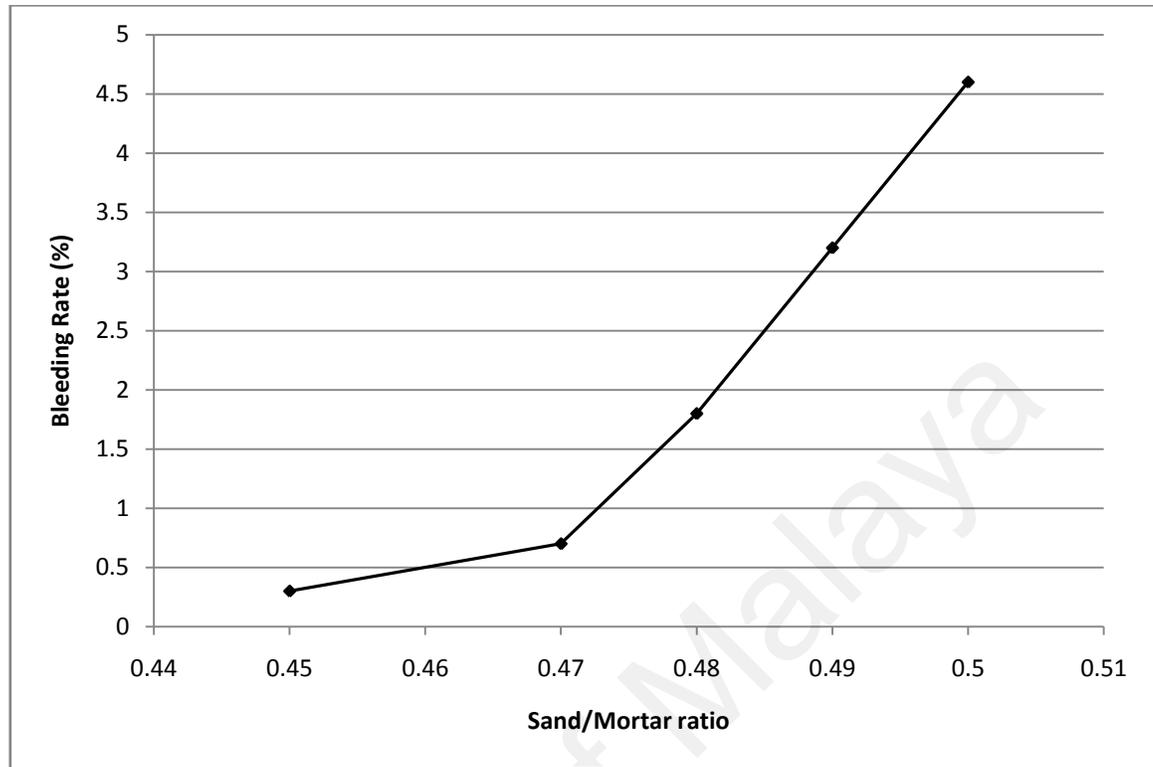
Figure 4.7: The relationship between the water bleeding rate of mortar and S/M ratio
