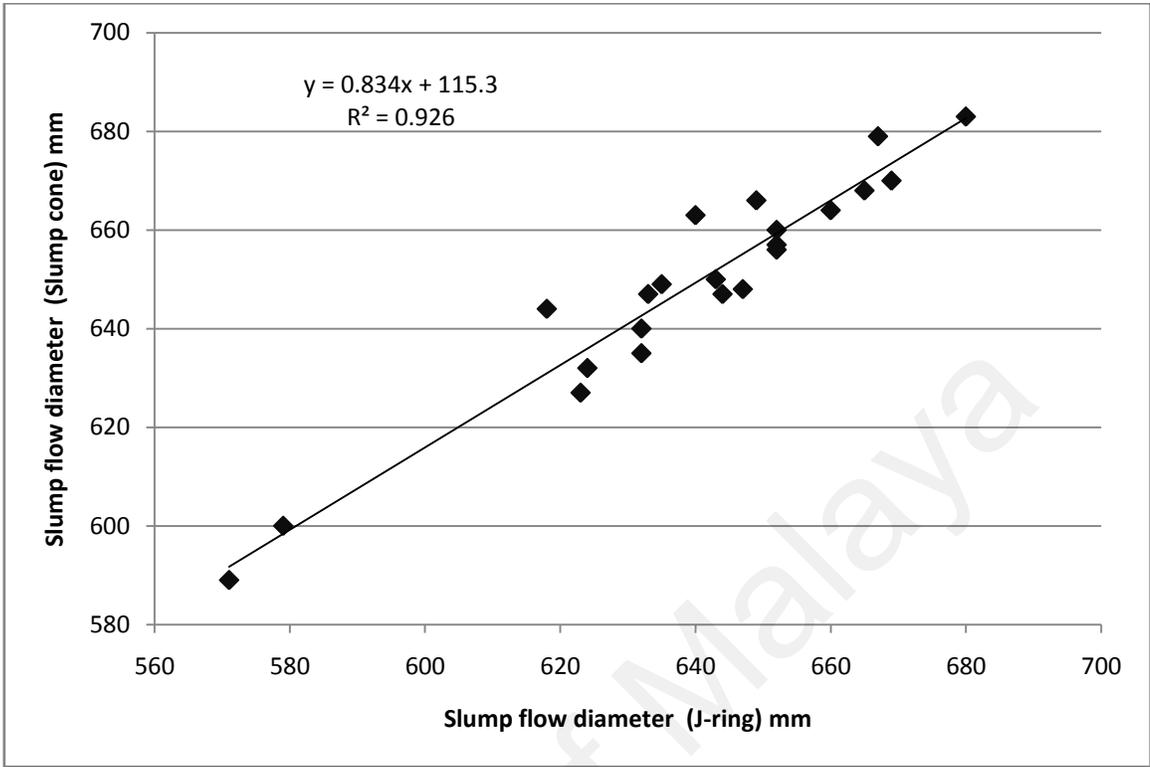
Figure 4.121: The relationship between slump flow diameter of J-ring and slump flow tests
