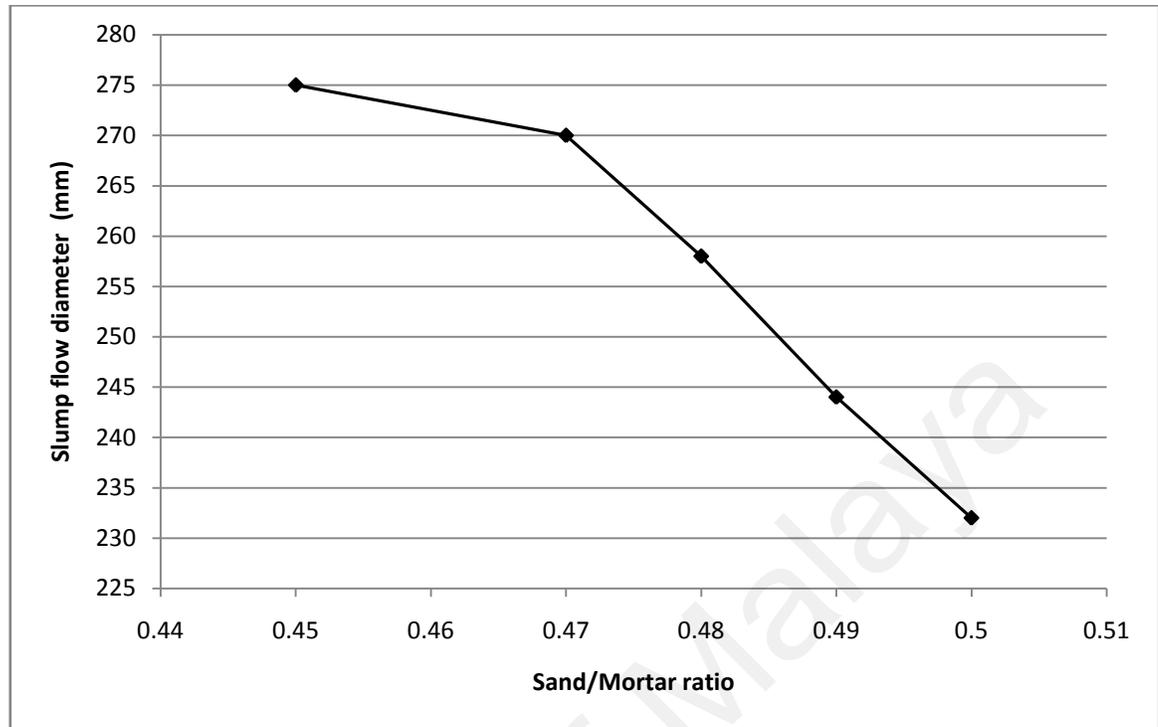
Figure 4.5: The relationship between the flow spread of mortar and S/M ratio
