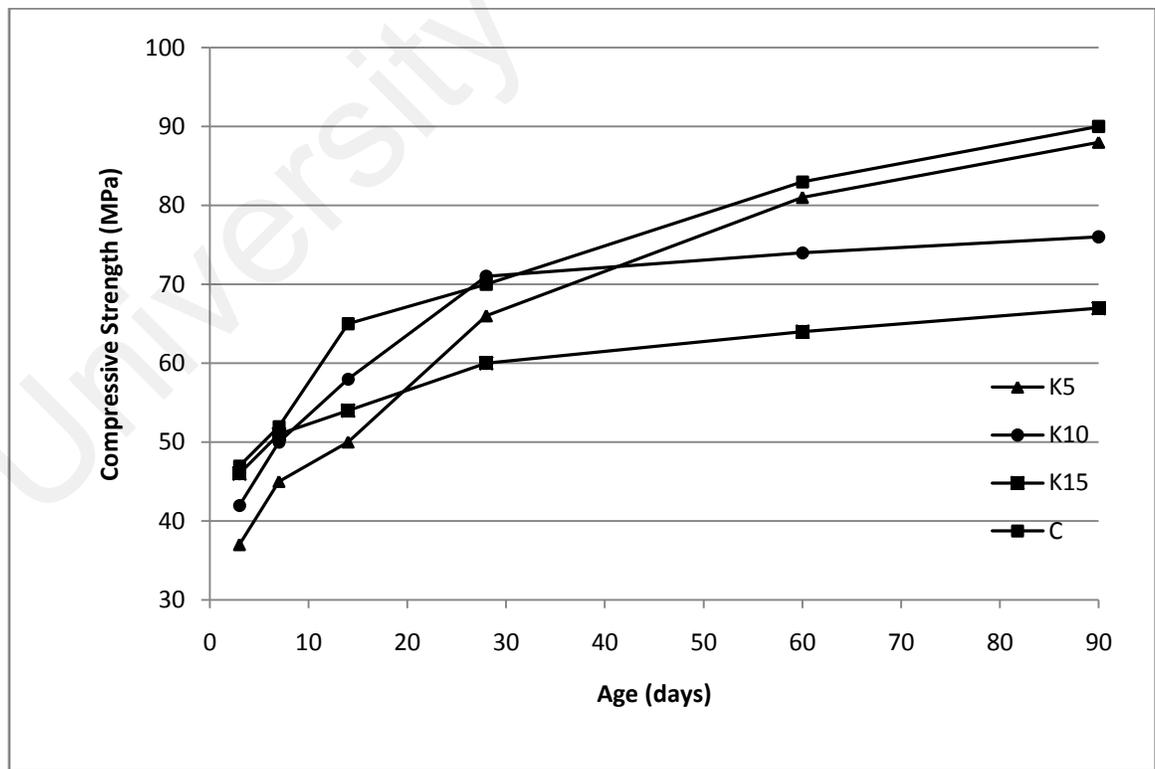
Figure 4.32: Compressive strength of kaolin mixes with age
