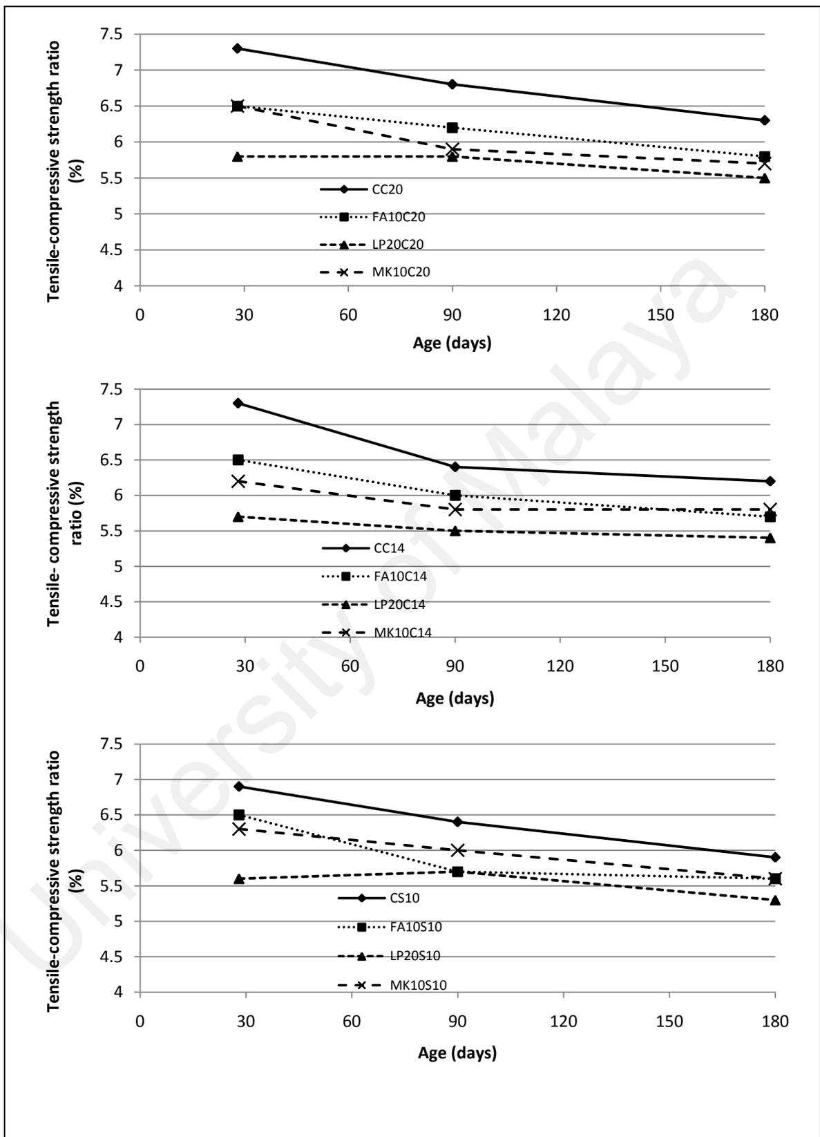
Figure 4.82: Tensile- compressive strength ratio of different mineral admixture concrete mixes
