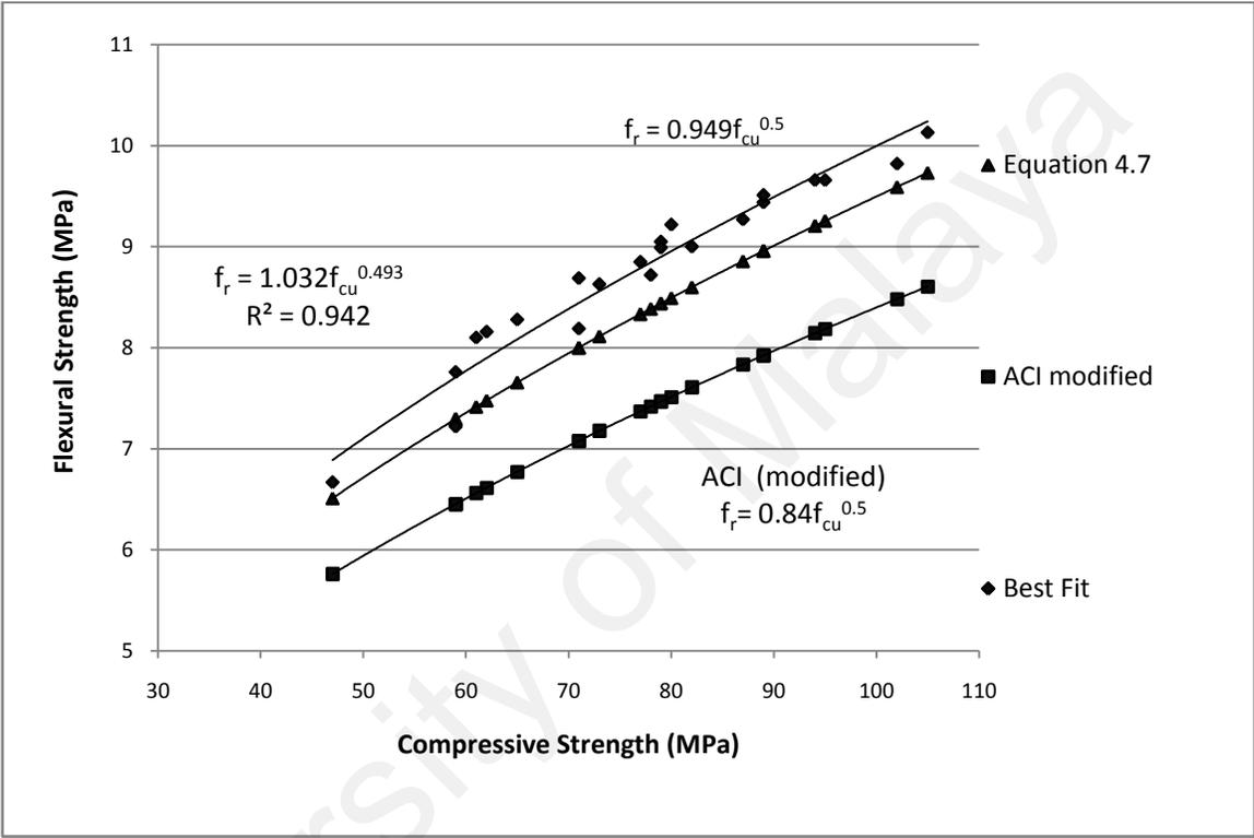
Figure 4.124: The comparison between the present study and other study of the relationship between flexural and compressive strength
