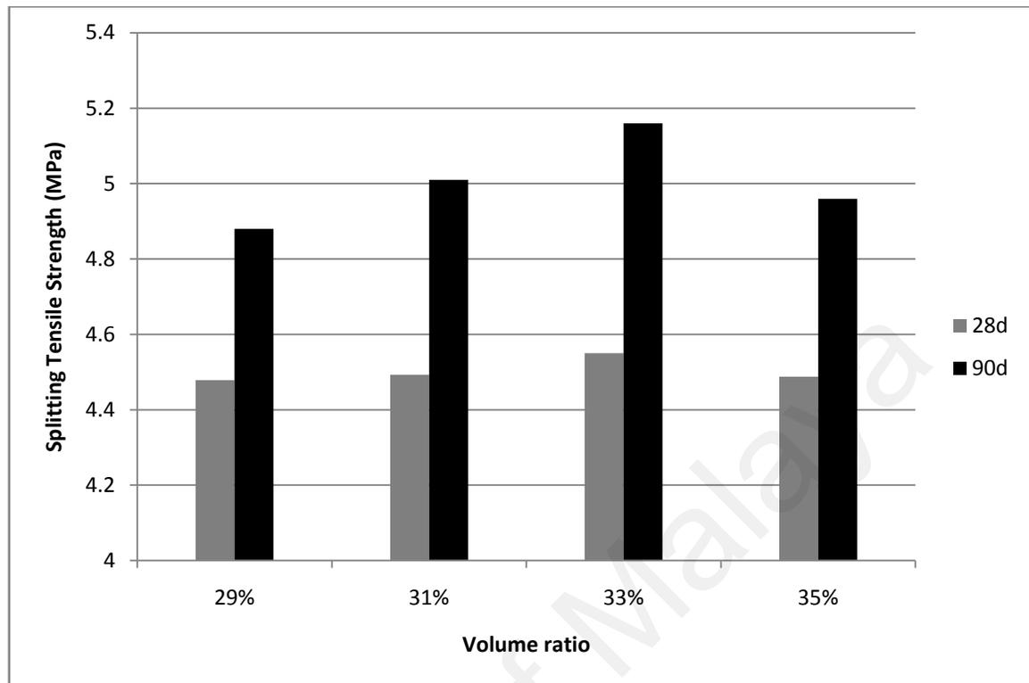
Figure 4.91: Splitting tensile strength of different aggregate contents
