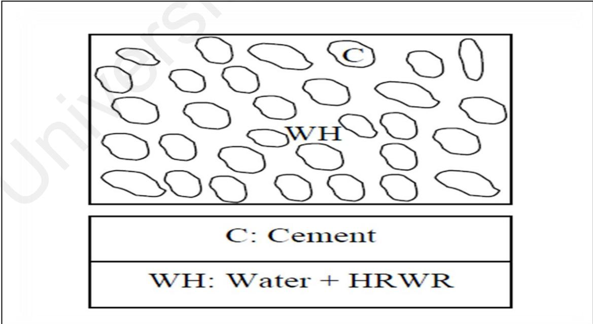
Figure 2.5: Dispersion of cement particles in presence of HRWR (Safiuddin, 2008)
