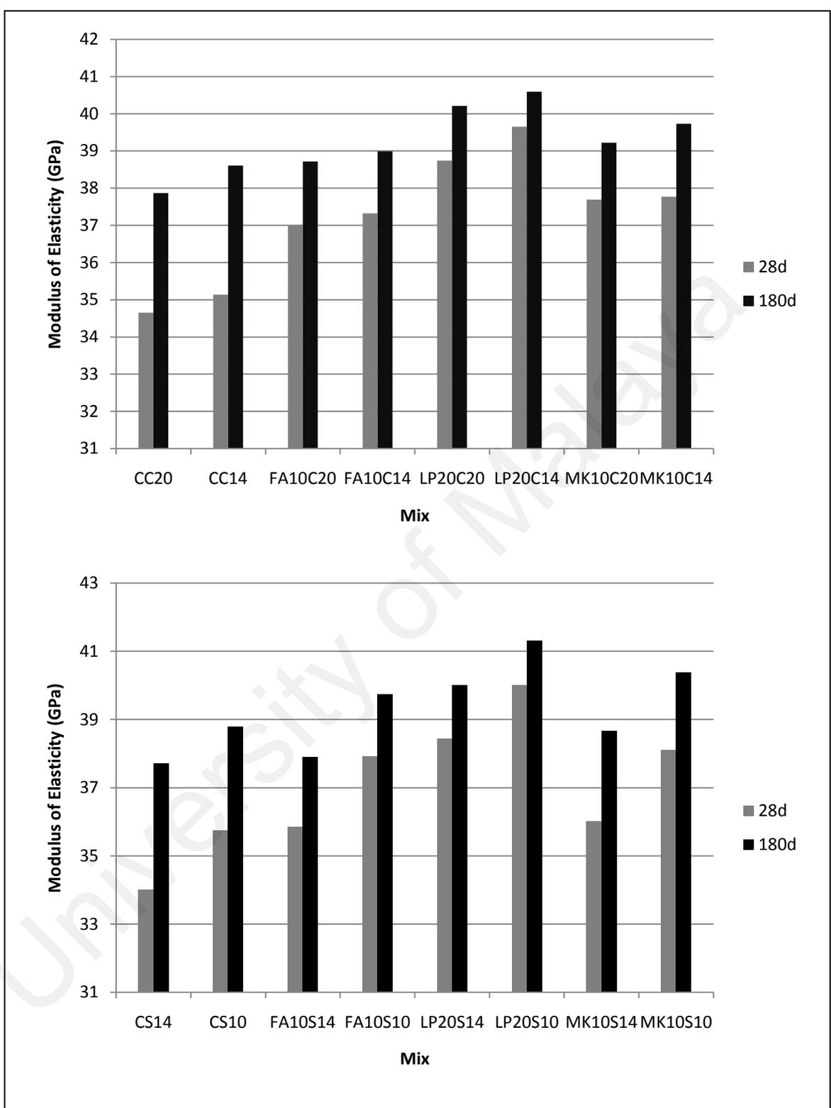
Figure 4.100: Modulus of elasticity of concretes with different maximum size aggregate
