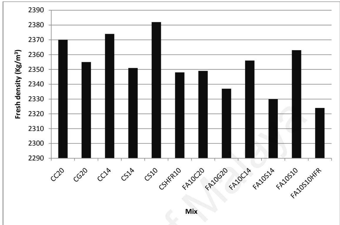
Figure 4.36: Fresh densities of fly ash and control concrete mixes
