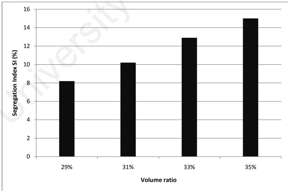
Figure 4.53: Segregation index of different coarse aggregate content mixes
