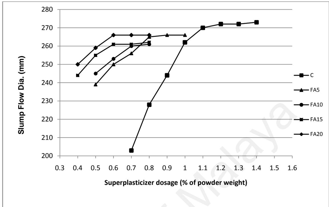
Figure 4.8: The optimum superplasticizer dosage of control and fly mixes
