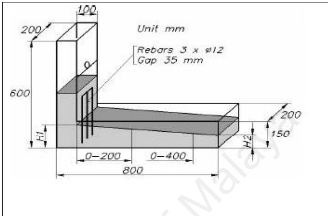
Figure 3.8: L-Box test
