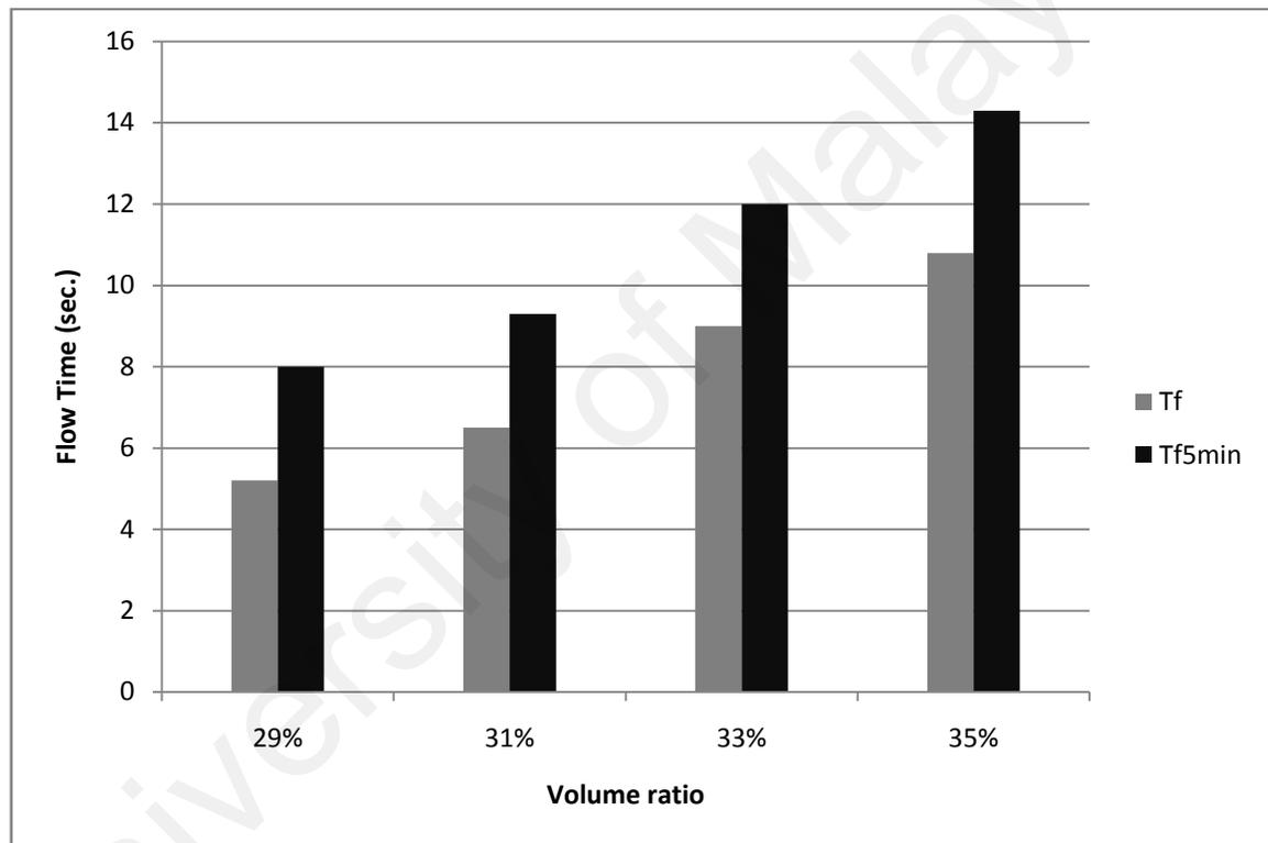
Figure 4.49: Flow time and flow time after 5min. of different coarse aggregate volume control mixes
