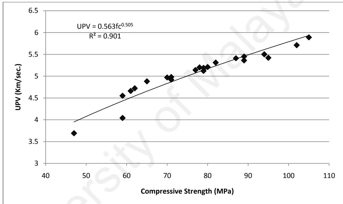
Figure 4.128: The relationship between UPV and compressive strength
