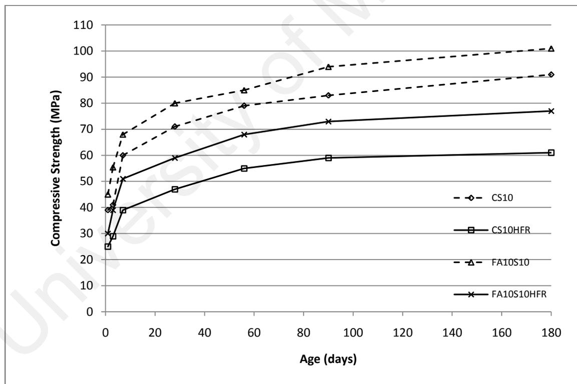
Figure 111: Compressive strength of concretes with different shape aggregate
