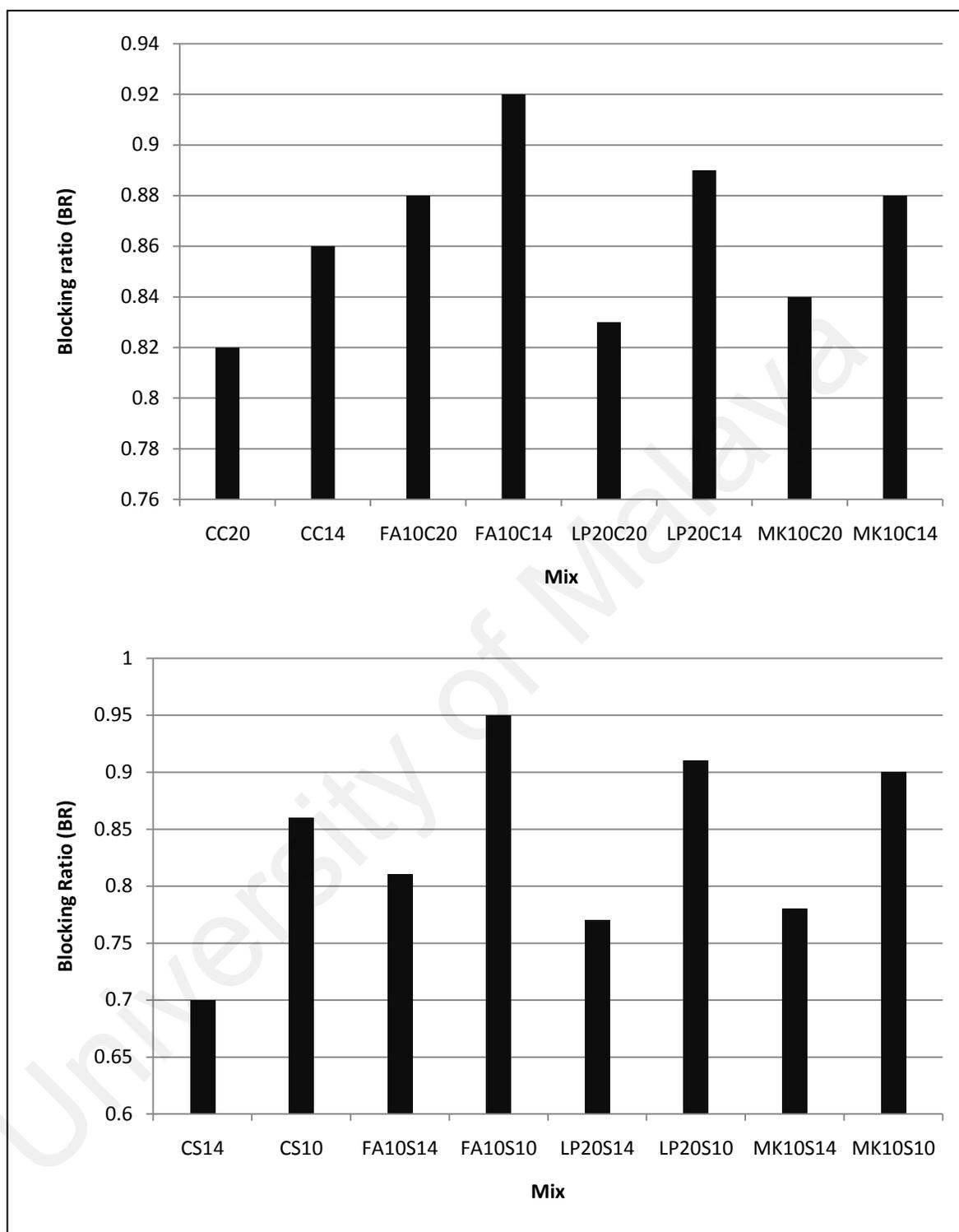
Figure 4.57: Blocking ratio different maximum size aggregate mixes
