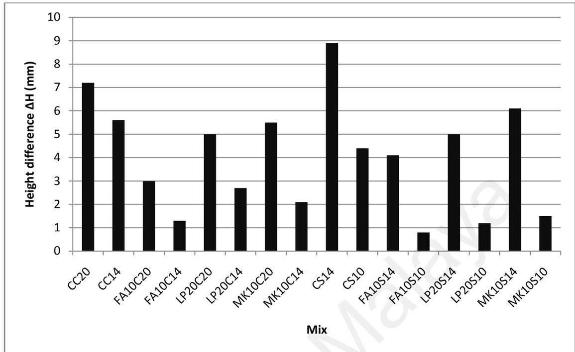
Figure 4.59: Height difference  $\Delta H$  of J-ring test of different maximum size mixes
