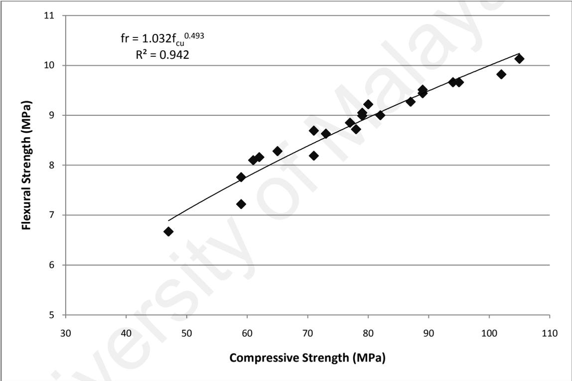
Figure 4.123: The relationship between flexural and compressive strength
