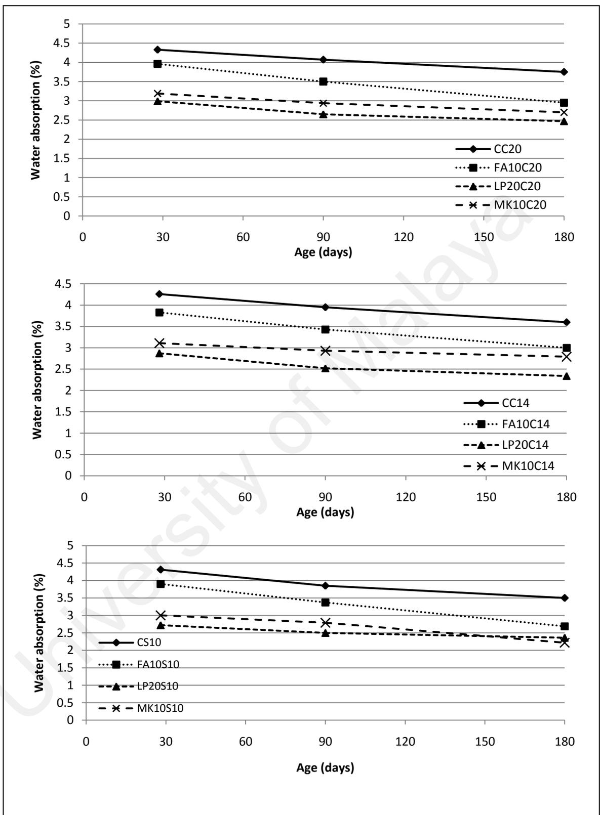
Figure 4.86: Water absorption of different mineral admixture mixes
