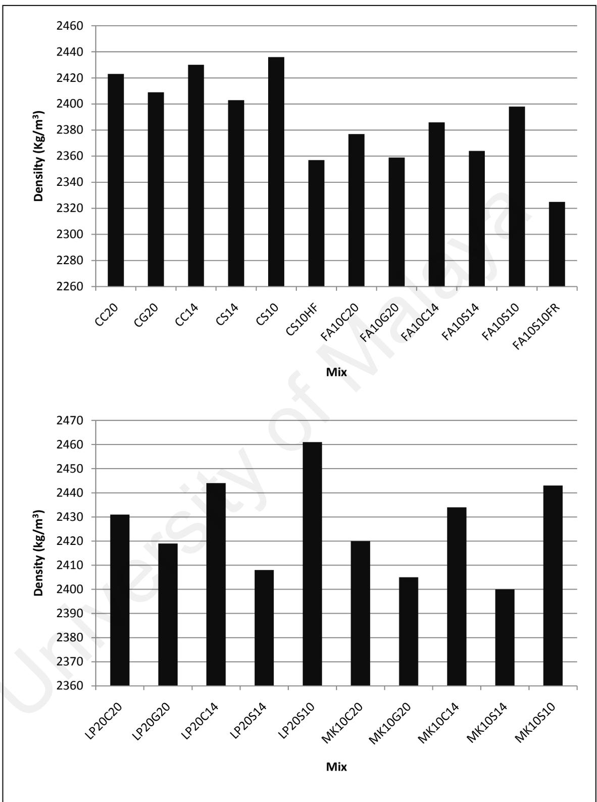
Figure 4.78: Hardened densities of all concrete mixes
