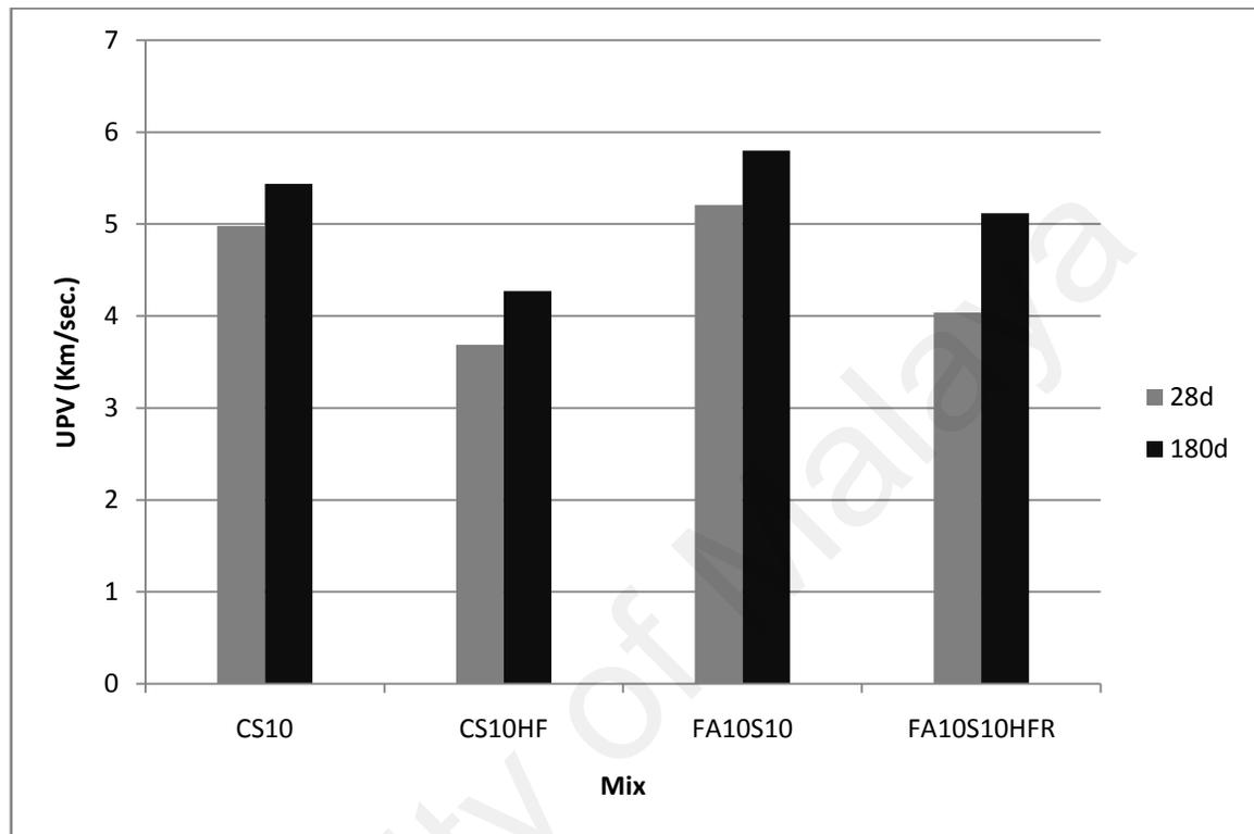
Figure 4.117: UPV of concretes with different shaped aggregate
