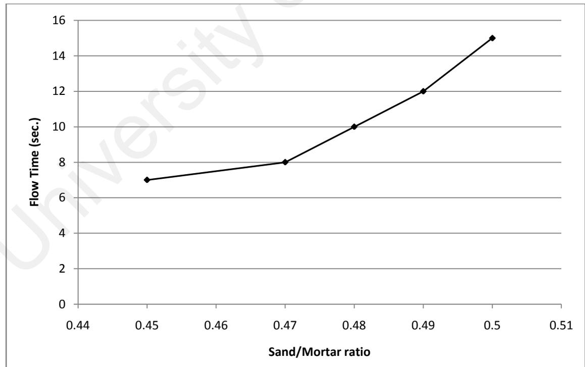
Figure 4.6: The relationship between the flow time of mortar and S/M ratio
