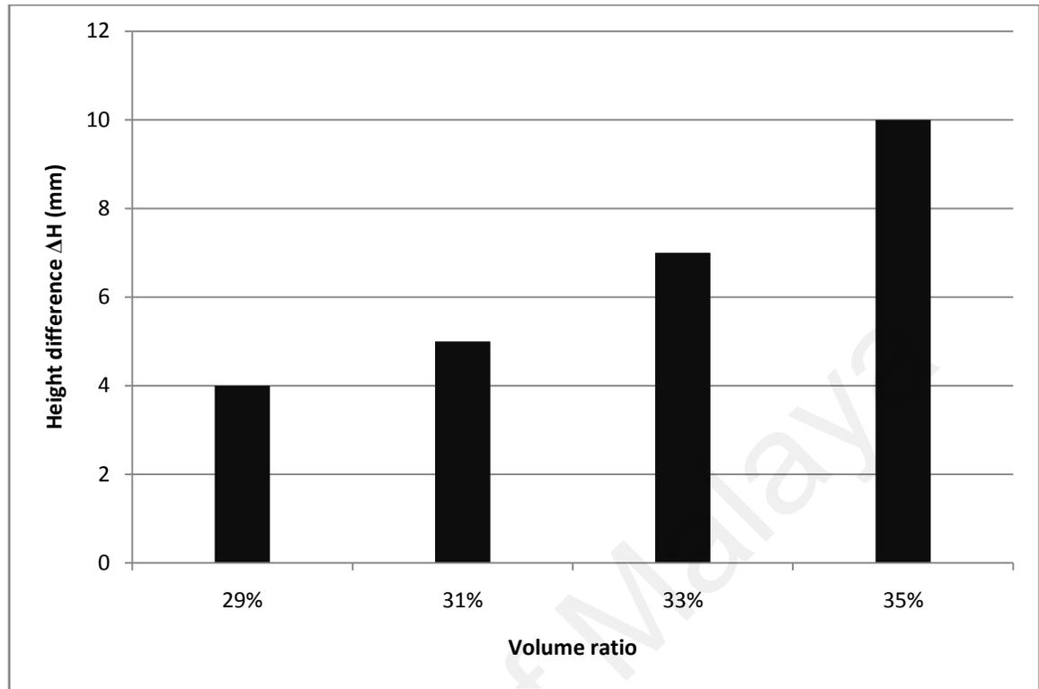
Figure 4.52: Height difference ( $\Delta H$ ) of J-ring test of different coarse aggregate content mixes
