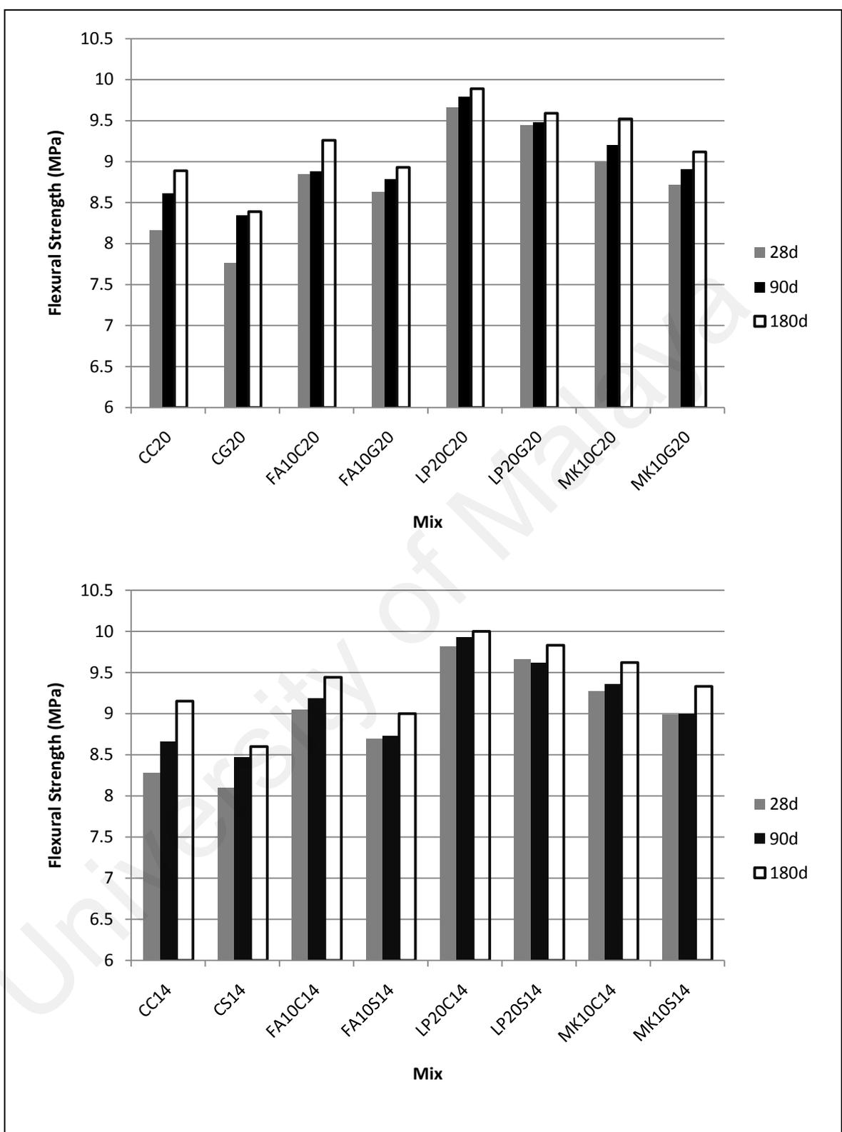
Figure 4.106: Flexural strength of concretes with different graded aggregate
