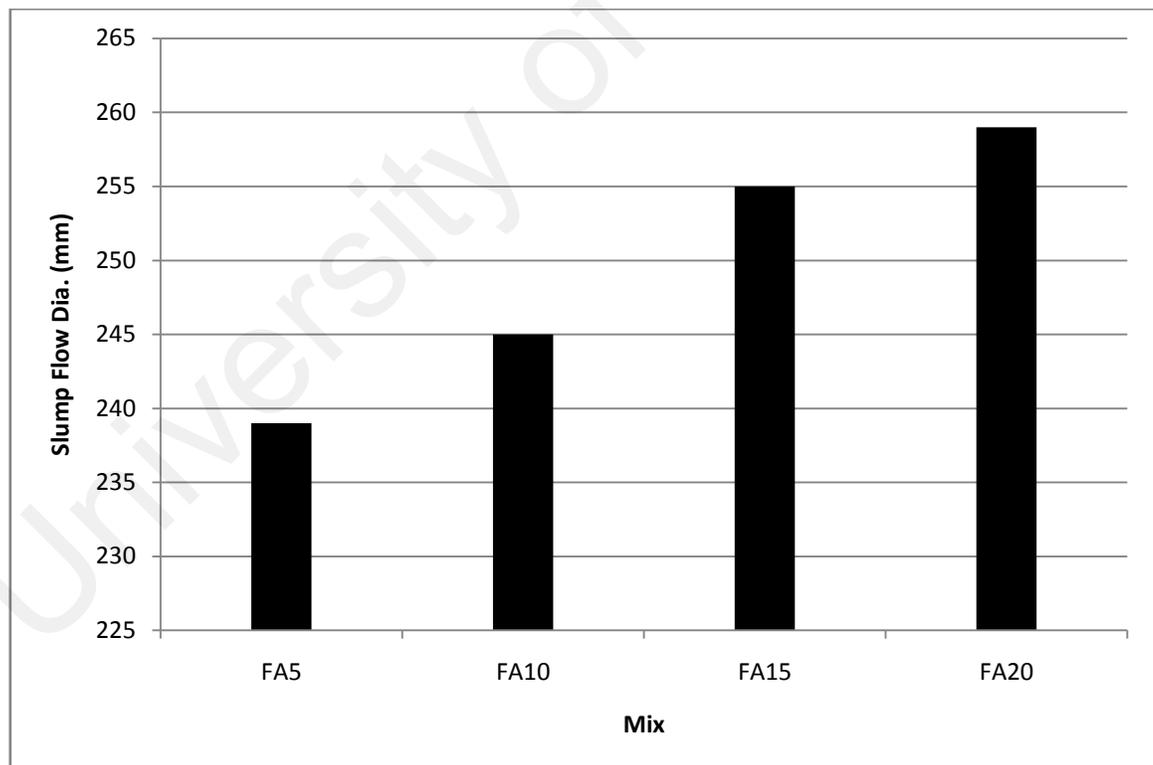
Figure 4.10: Flow spread of fly ash mixes with same w/p ratio and superplasticizer dosage
