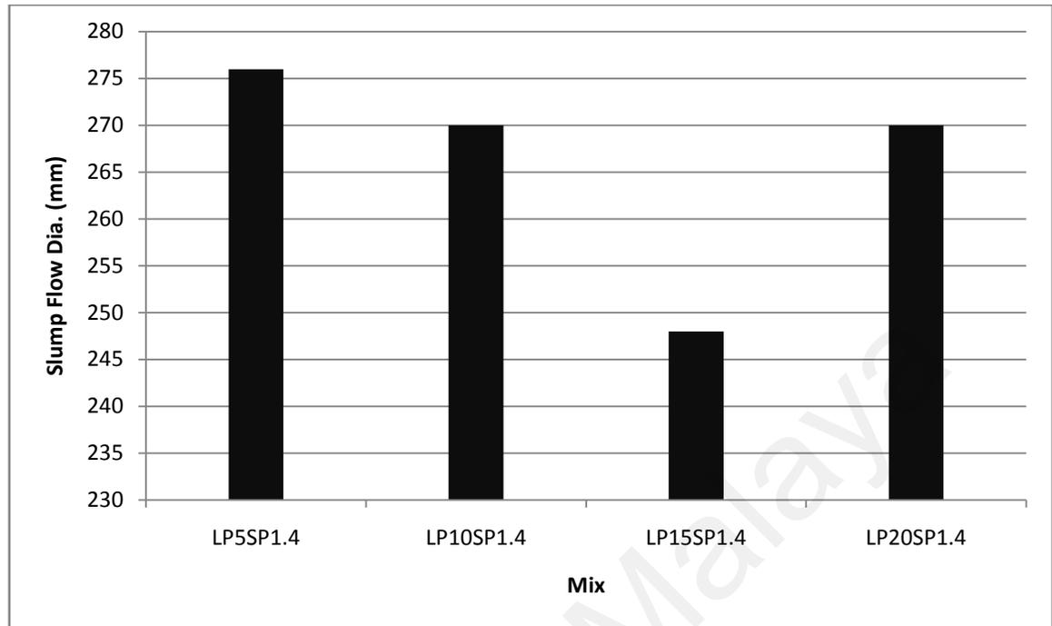
Figure 4.18: Flow spread of limestone mixes with same w/p ratio and superplasticizer dosage
