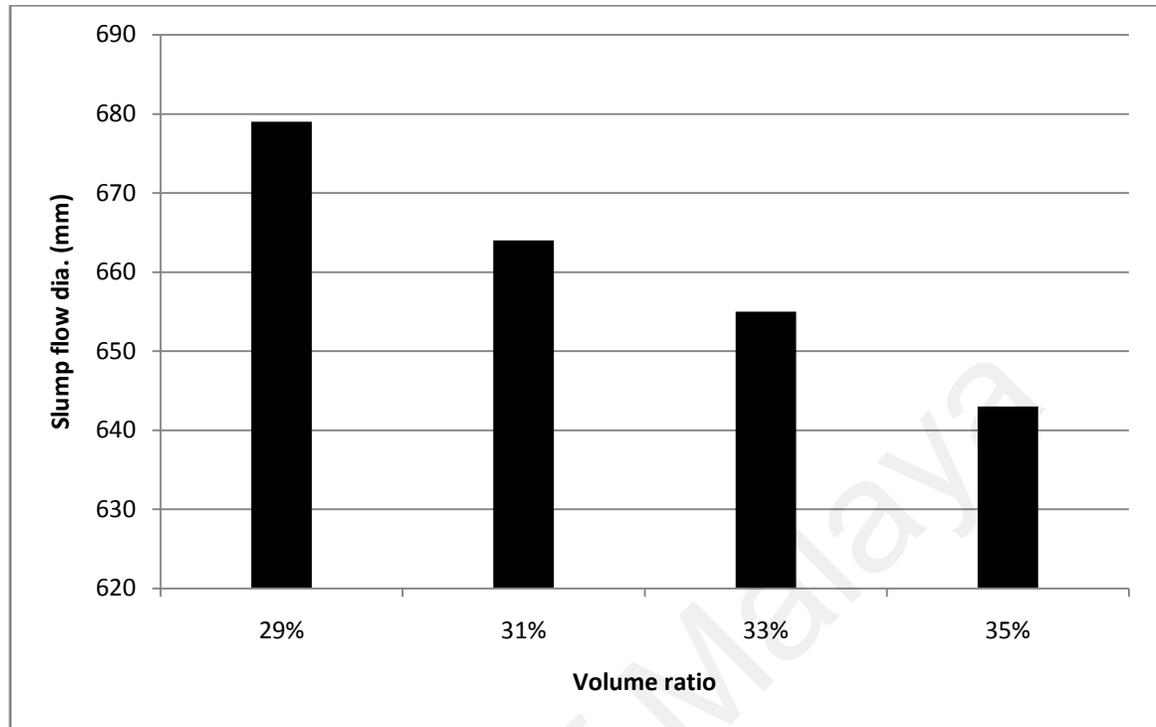
Figure 4.47: Slump flow diameter of different coarse aggregate volume control mixes
