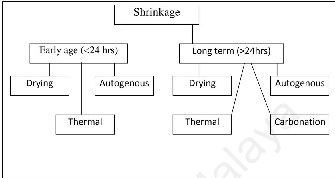
Figure 2.12: Diagram of shrinkage stages and types (Holt, 2001)
