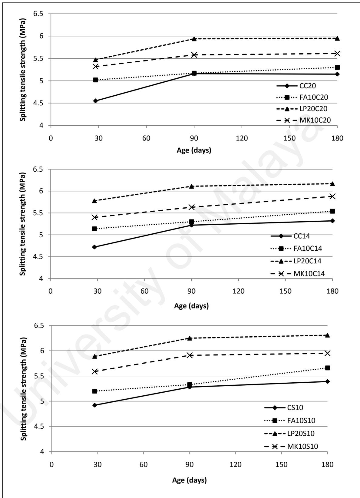
Figure 4.81: Splitting tensile strength of different mineral admixture mixes
