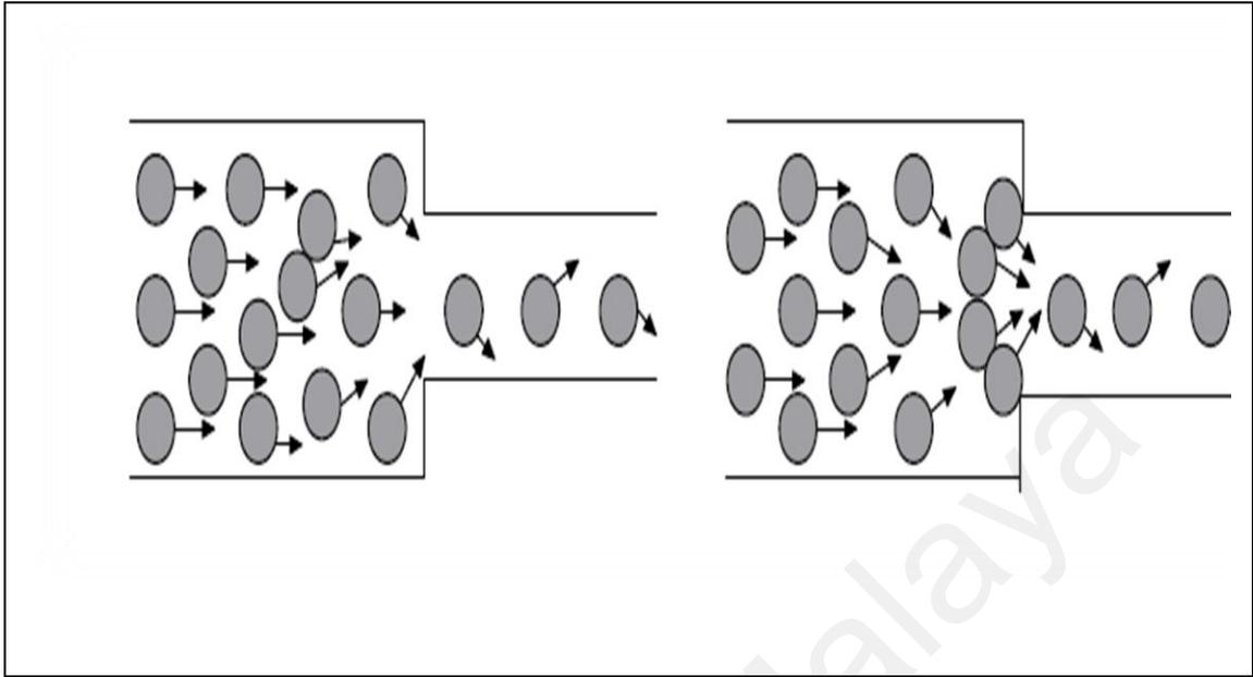
Figure 2.9: Schematic of blocking (RILEM TC 174 SCC, 2000)
