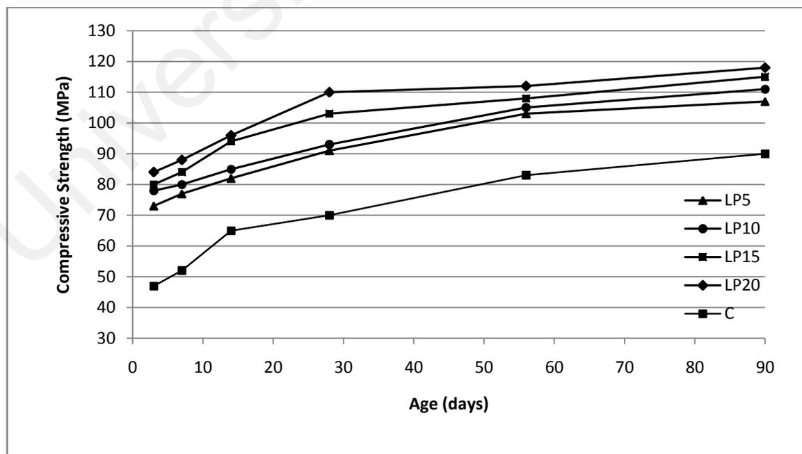
Figure 4.30: Compressive strength of limestone mixes with age
