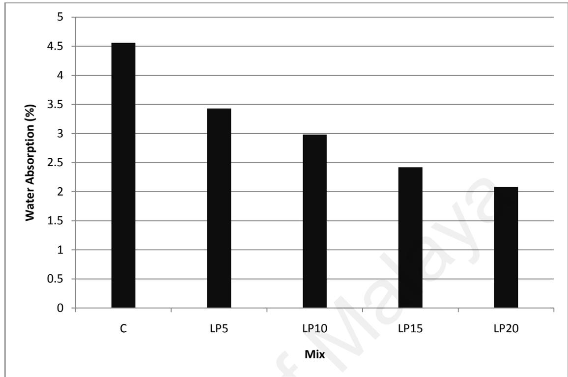
Figure 4.34: Water absorption of all limestone mixes and control mix
