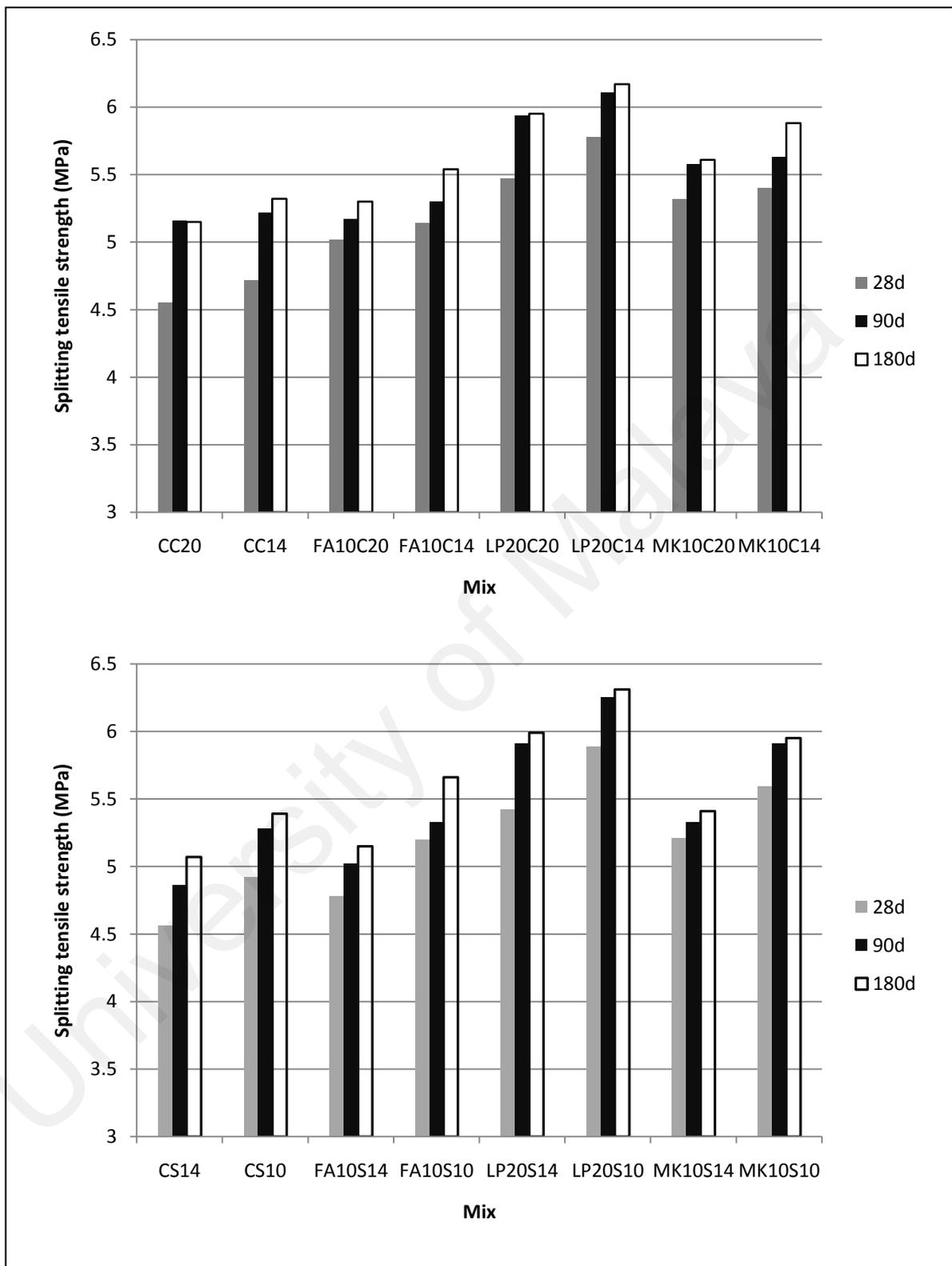
Figure 4.98: Splitting tensile strength of concretes with different maximum size aggregate
