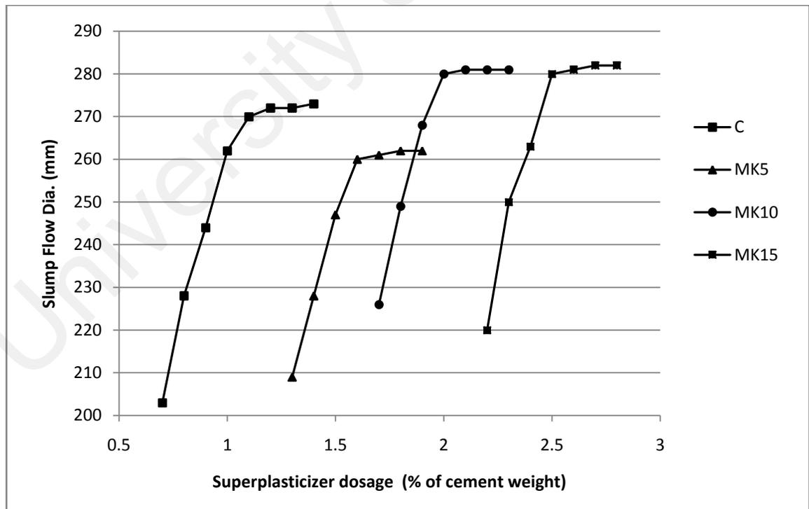
Figure 4.9: The optimum superplasticizer dosage of control and metakaolin mixes
