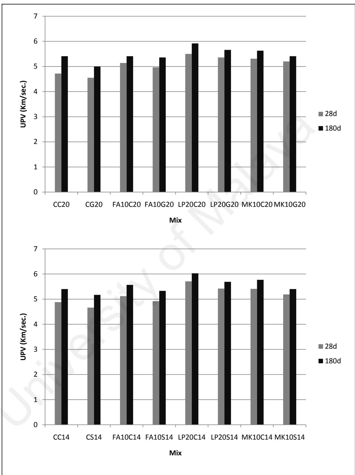
Figure 4.110: UPV values of concretes with different graded aggregate
