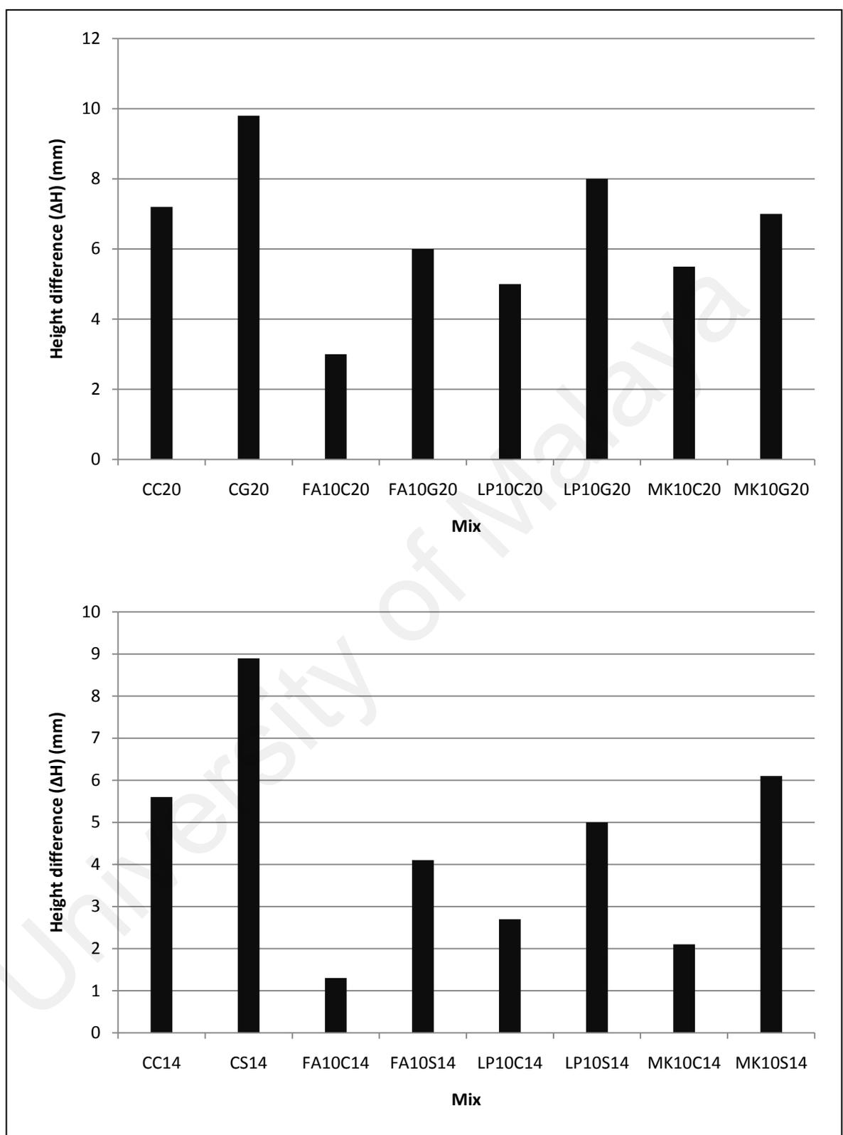
Figure 4.67: Height difference of different aggregate grades (graded and single) of mixes
