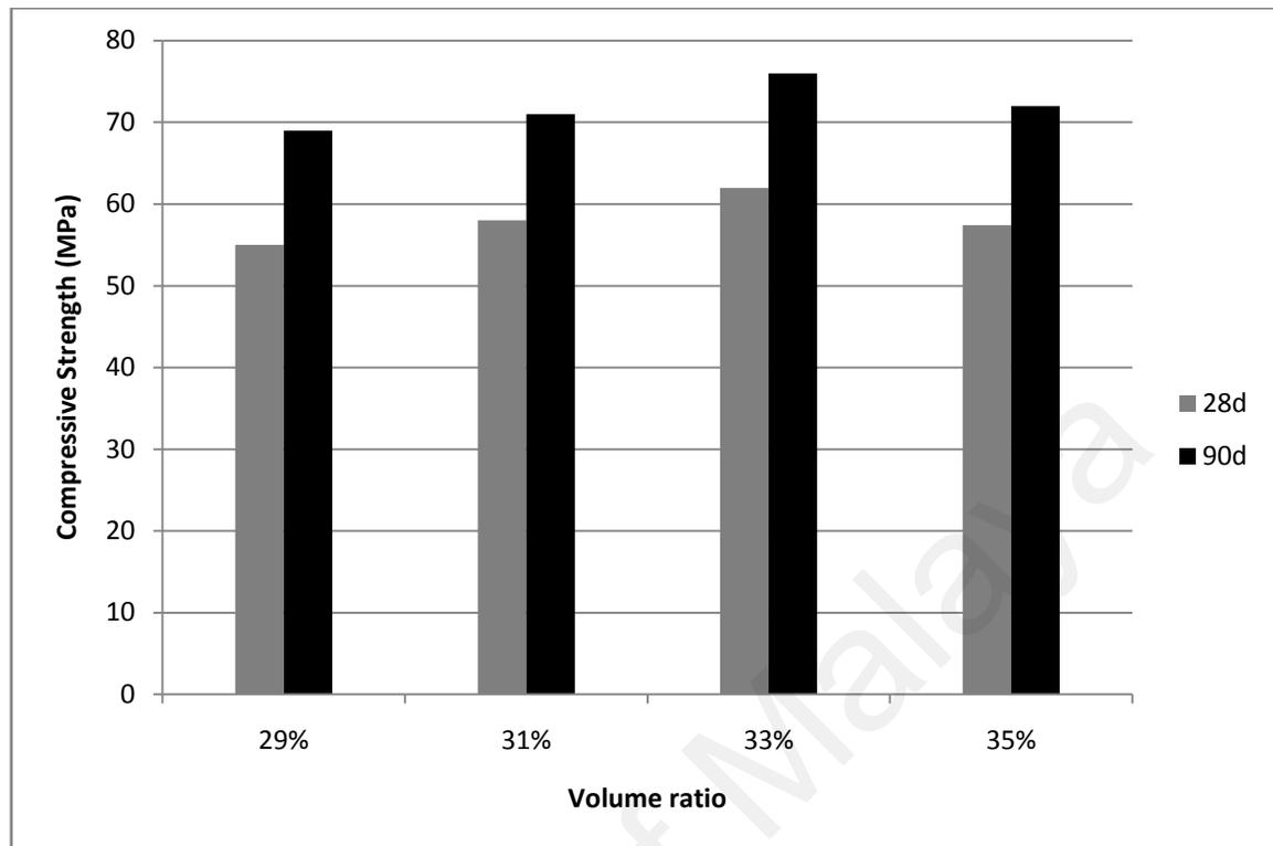
Figure 4.90: Compressive strength with different aggregate contents
