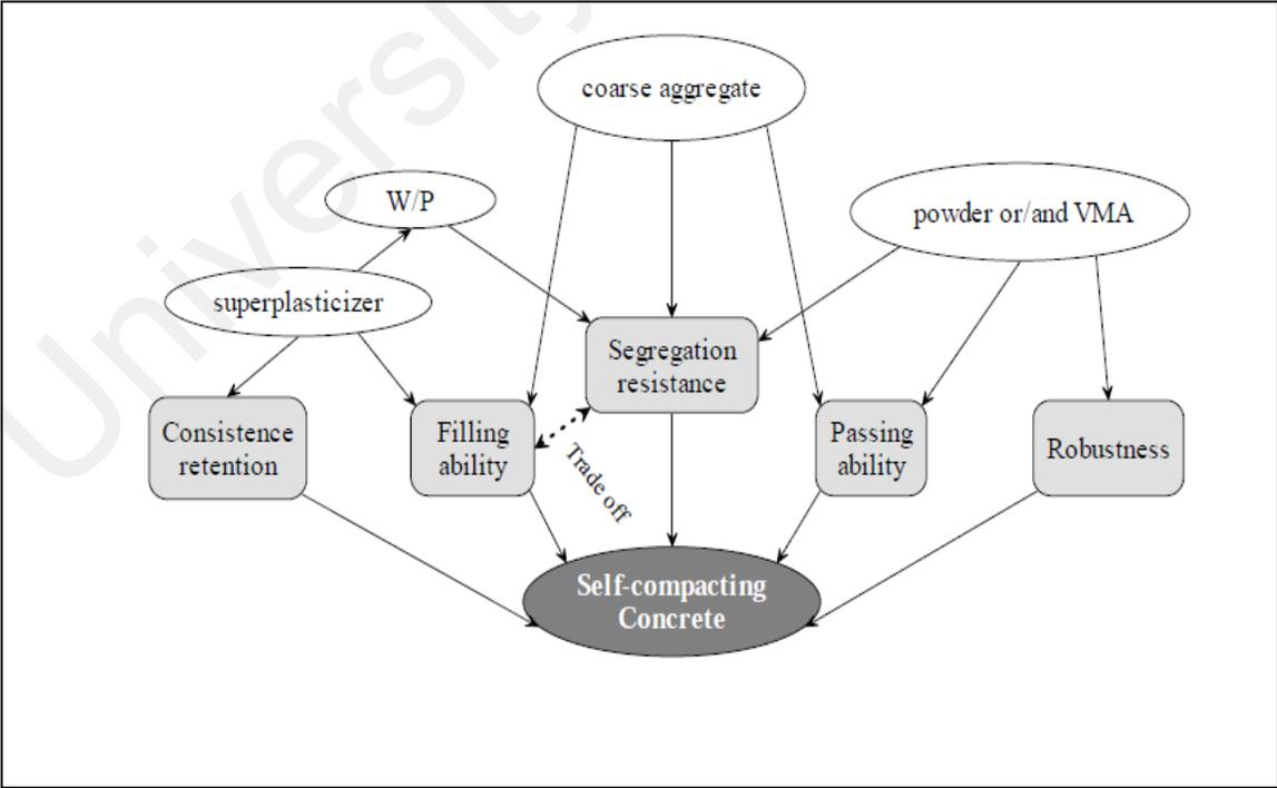
Figure 2.1: Flow chart for achieving self compactibility of concrete (Liu, 2009)
