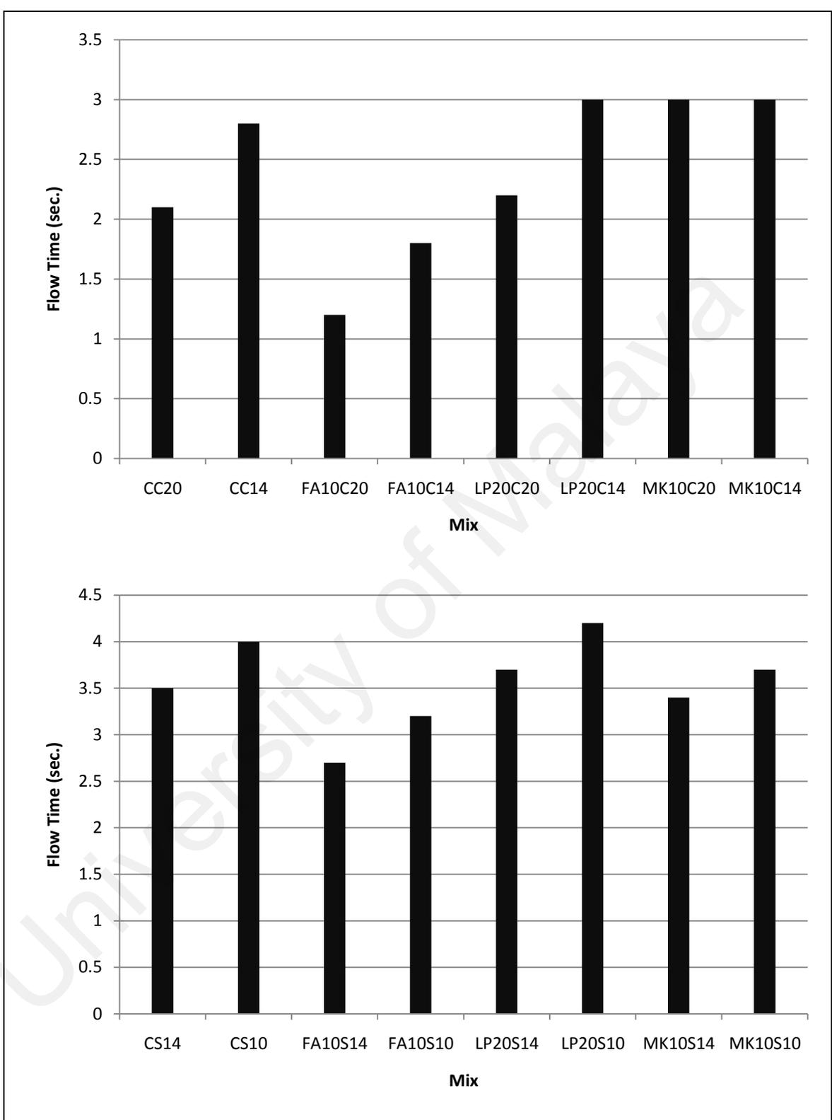
Figure 4.55:  $T_{50cm}$  of different maximum size aggregate (14 & 10mm single) mixes
