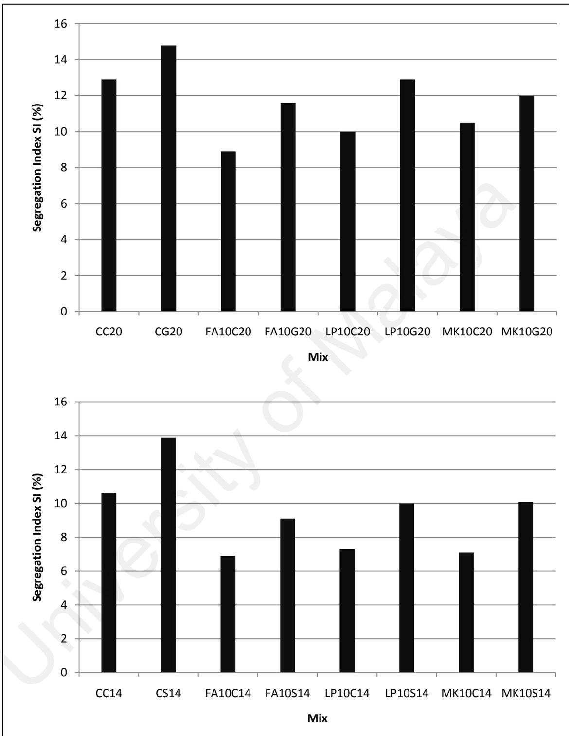
Figure 4.69: Segregation index of graded and single size aggregate concrete mixes
