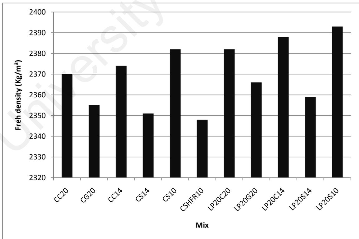
Figure 4.37: Fresh densities of limestone and control concrete mixes
