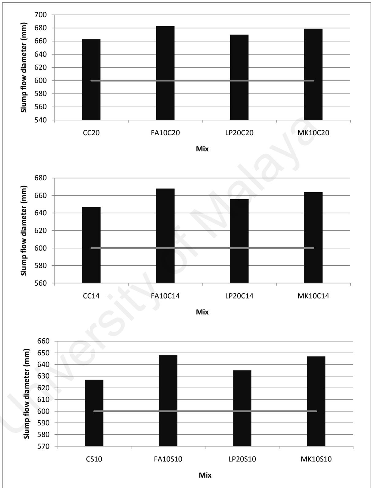
Figure 4.39: Slump flow diameter of different mineral admixture concrete mixes
