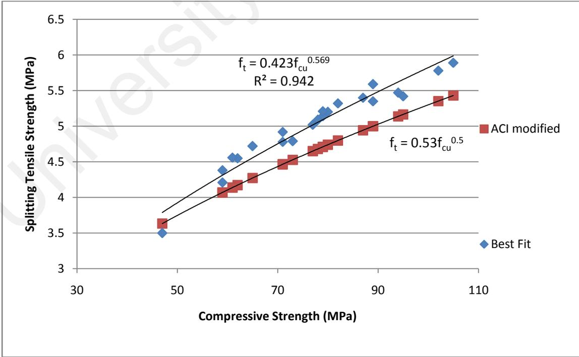
Figure 4.122: The relationship between splitting tensile and compressive strength of HSSCC
