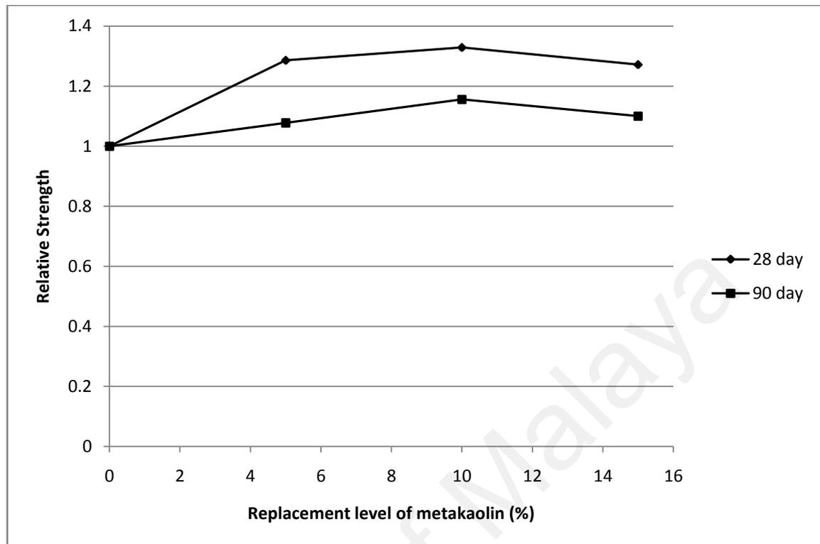
Figure 4.27: Relative strength of metakaolin mixes at 28 and 90 days
