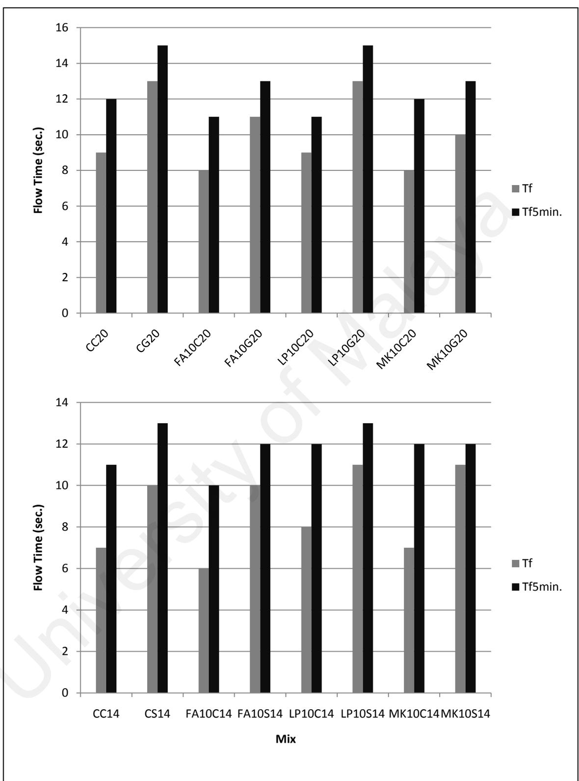
Figure 4.64: Flow time through V-funnel of different aggregate grades of mixes
