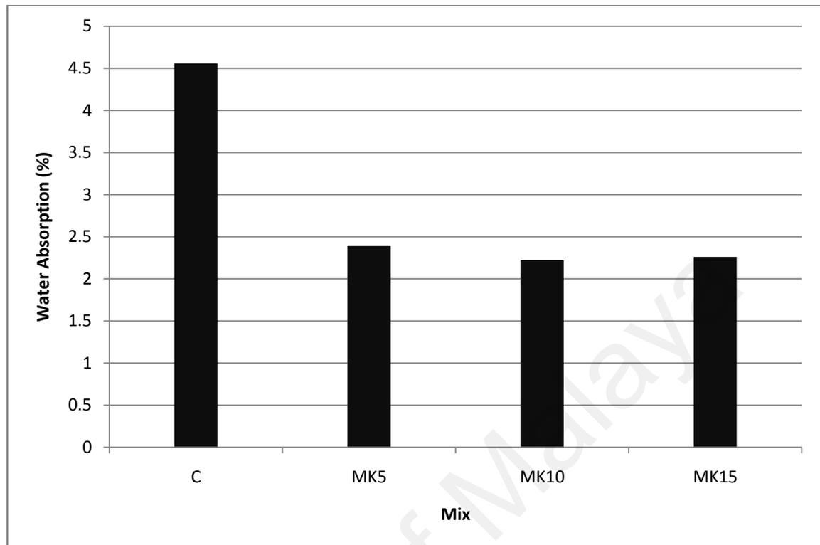
Figure 4.29: Water absorption of all metakaolin mixes and control mix
