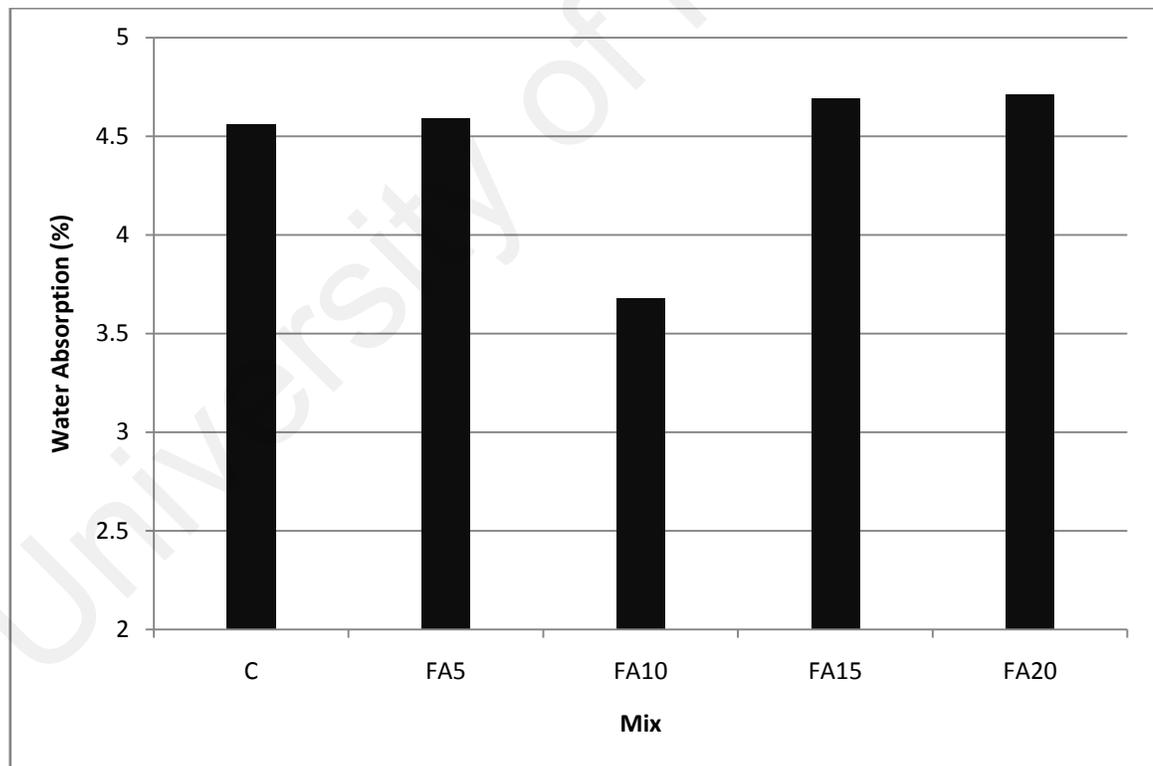
Figure 4.28: Water absorption of all fly ash mixes and control mix
