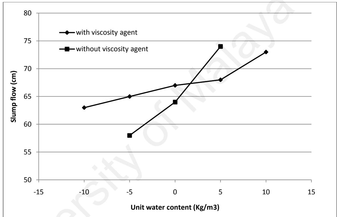
Figure 2.6: Slump flow with and without viscosity agent when water content is varied (water cement ratio 0.53) (Emborg, 2000).
