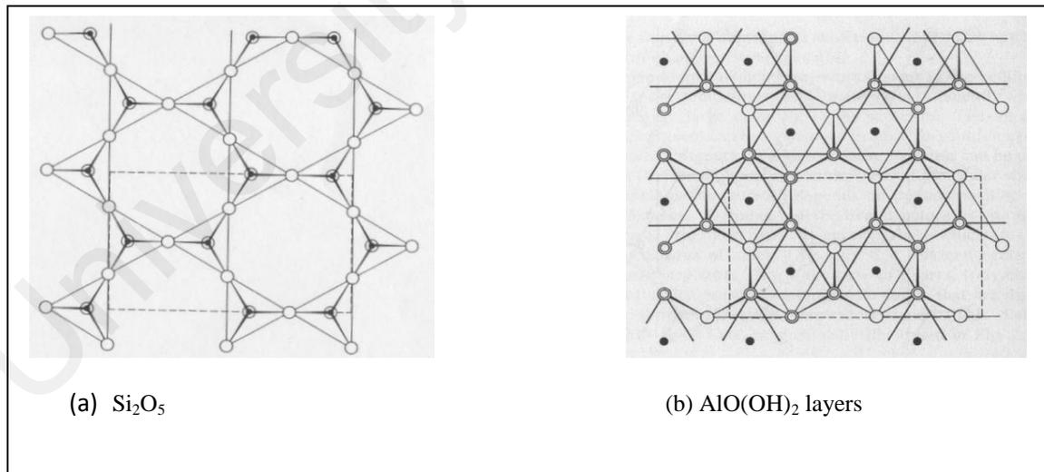
Figure 2.2: Atomic arrangements of (a)  $\text{Si}_2\text{O}_5$  and (b)  $\text{AlO}(\text{OH})_2$  layers – ( Justice, 2005)
