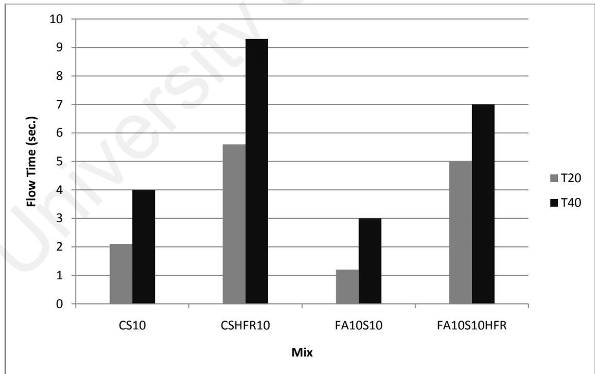
Figure 4.74: T20 & T40cm of different shape aggregate concrete mixes
