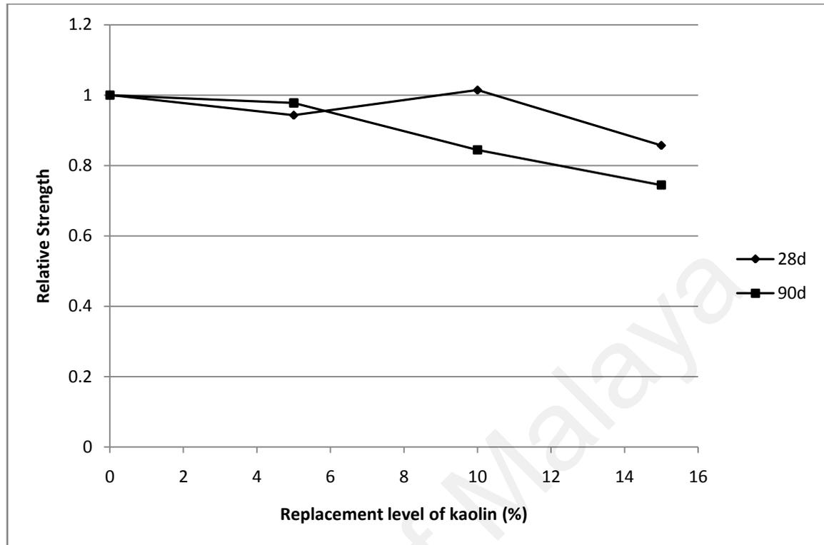
Figure 4.33: Relative strength of kaolin mixes at 28 and 90 days
