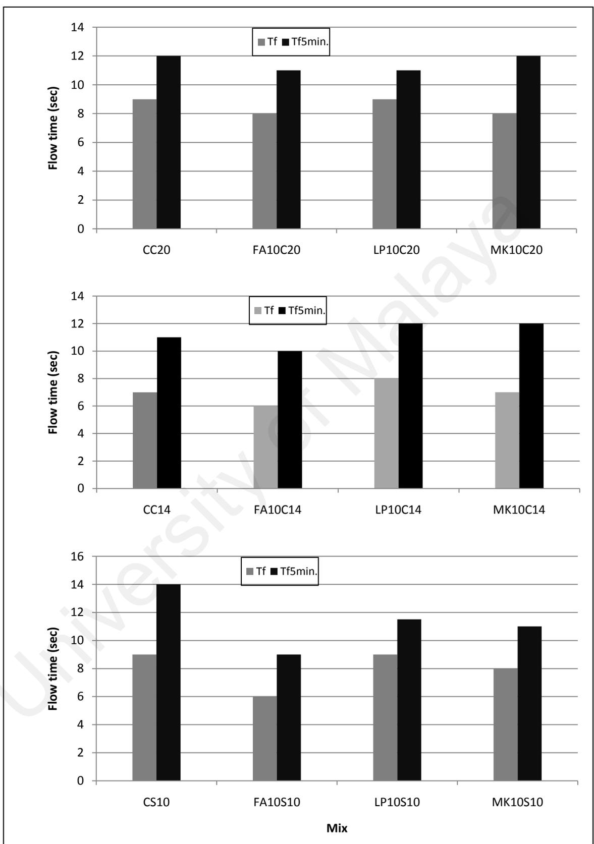
Figure 4.41: Flow time and flow time after 5min. of different mineral admixture concrete mixes
