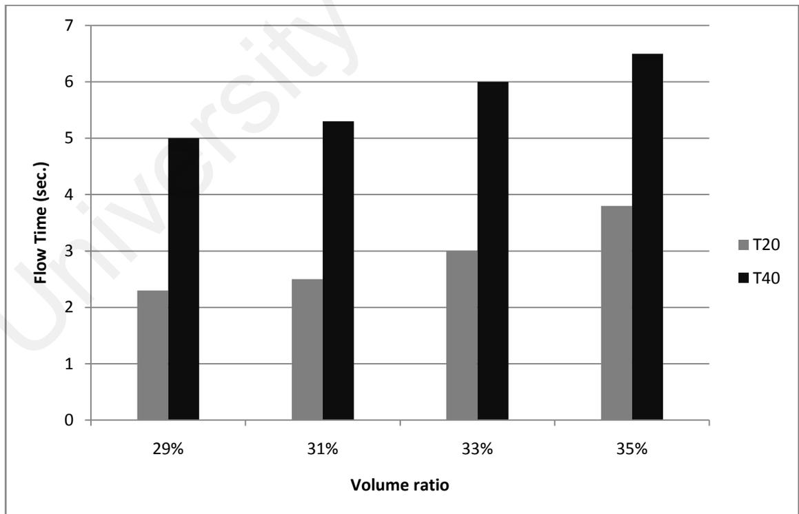
Figure 4.51: Flow time at 20cm & 40cm of different volume ratio of coarse aggregate
