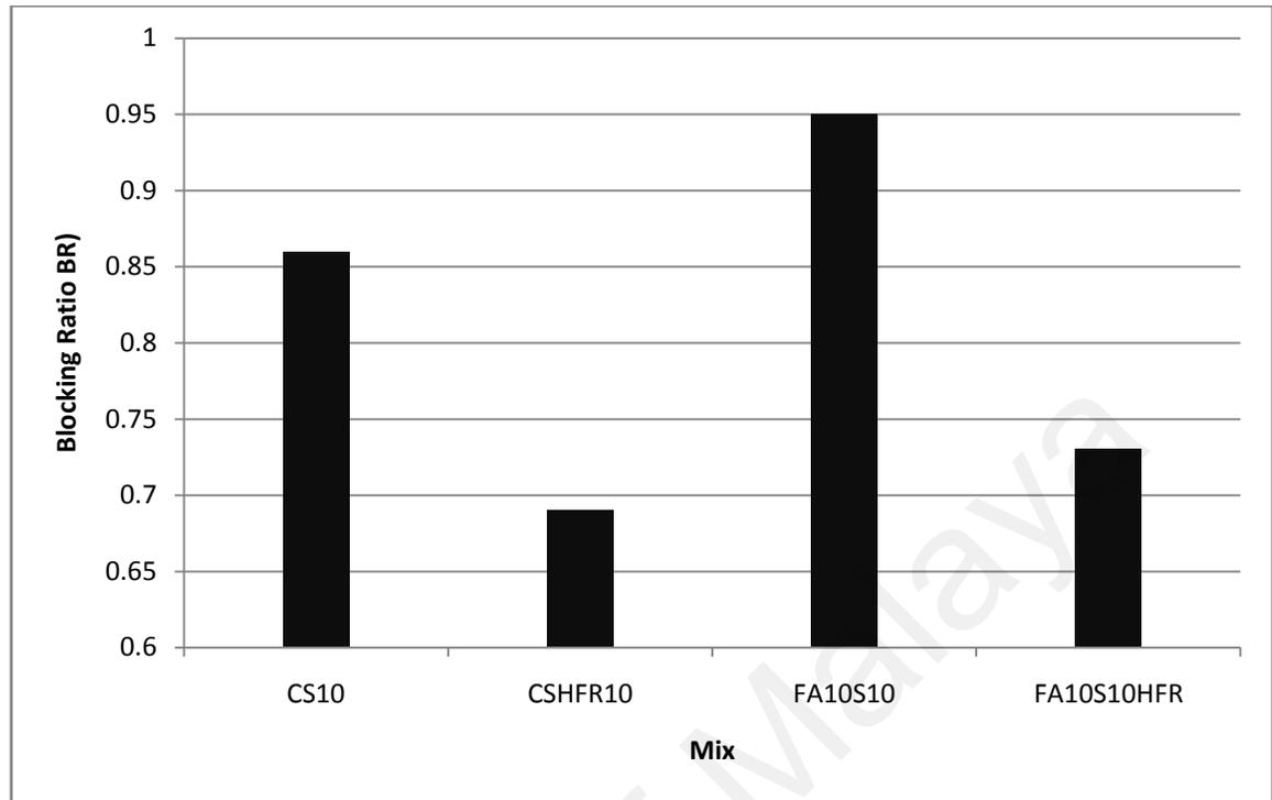
Figure 4.73: BR of different shape aggregate concrete mixes
