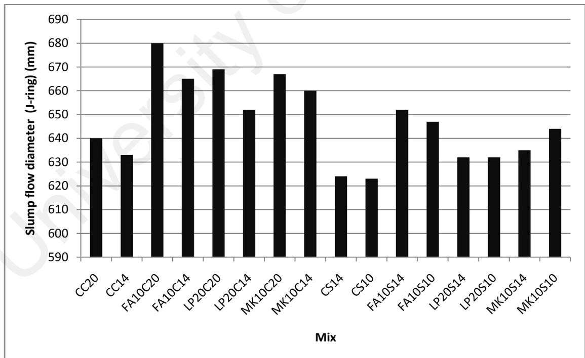
Figure 4.60: Slump flow diameter of different maximum size mixes
