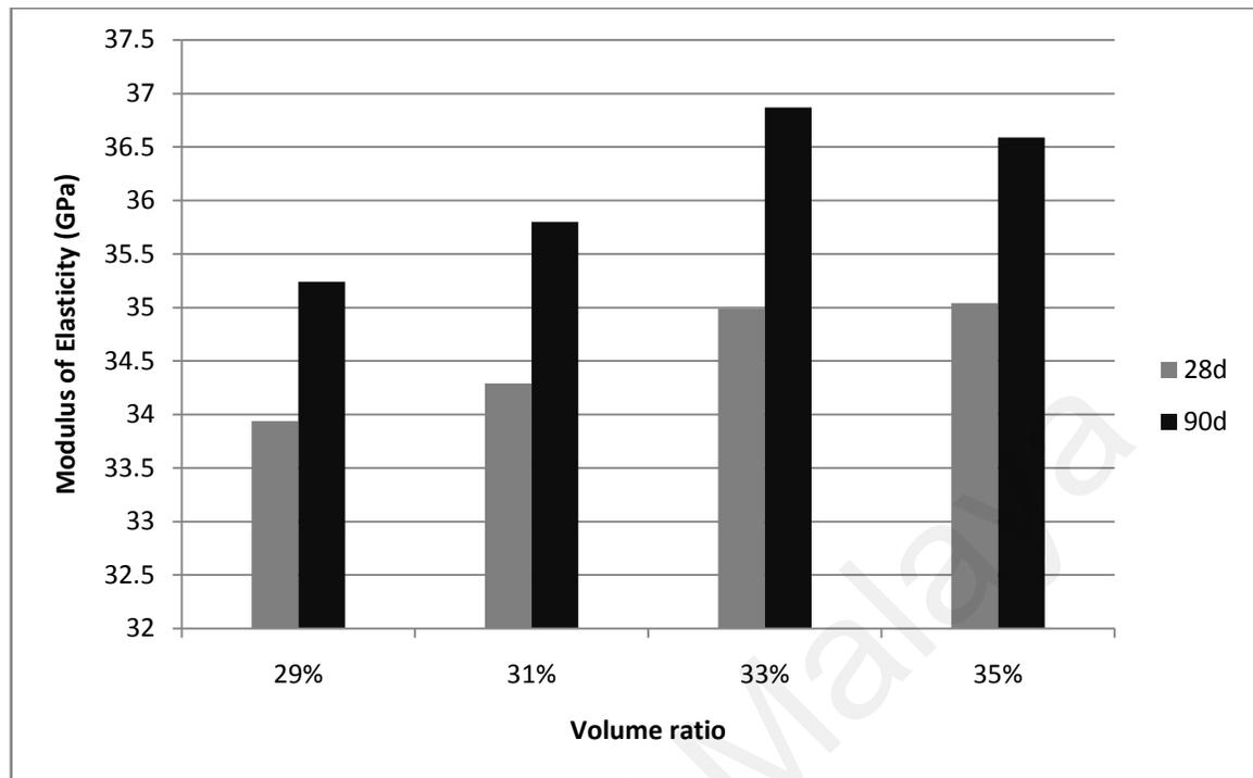
Figure 4.93: Modulus of elasticity of different aggregate contents
