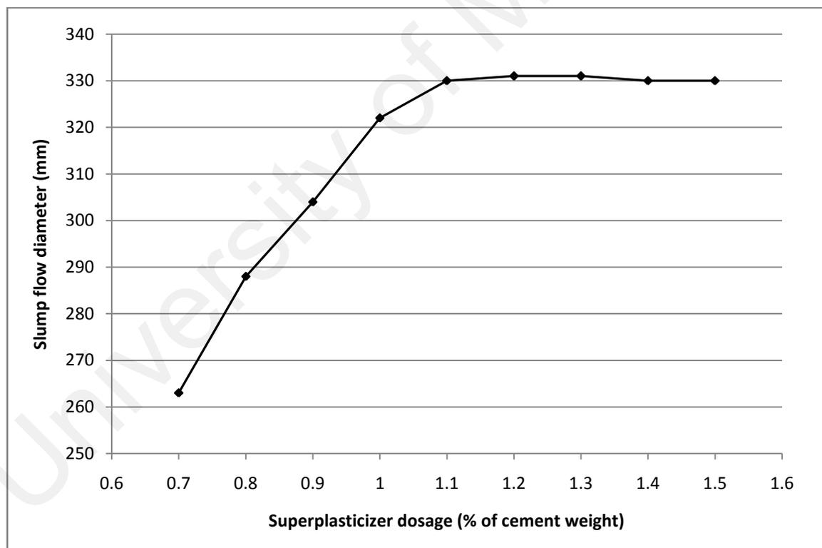
Figure 4.4: Flow spread of cement based paste
