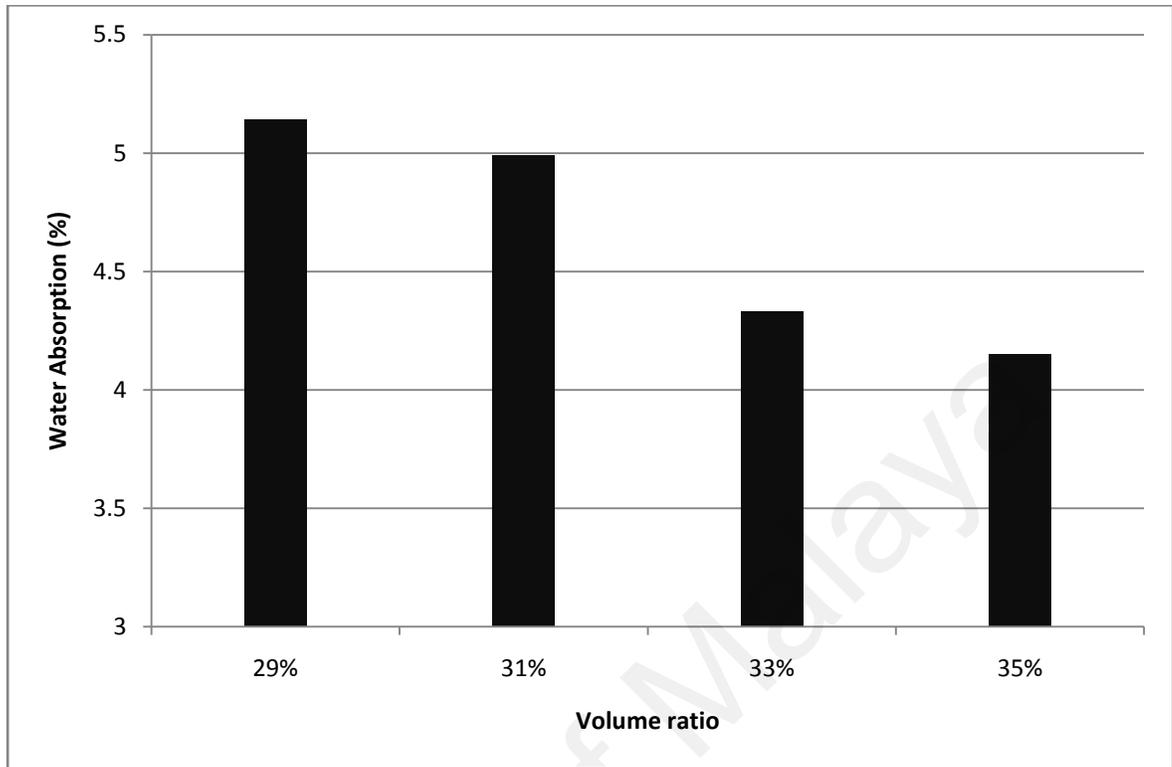
Figure 4.94: Water absorption of different aggregate contents at 28 days
