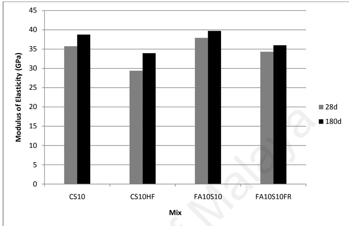
Figure 4.114: Modulus of elasticity of concretes with different shaped aggregate
