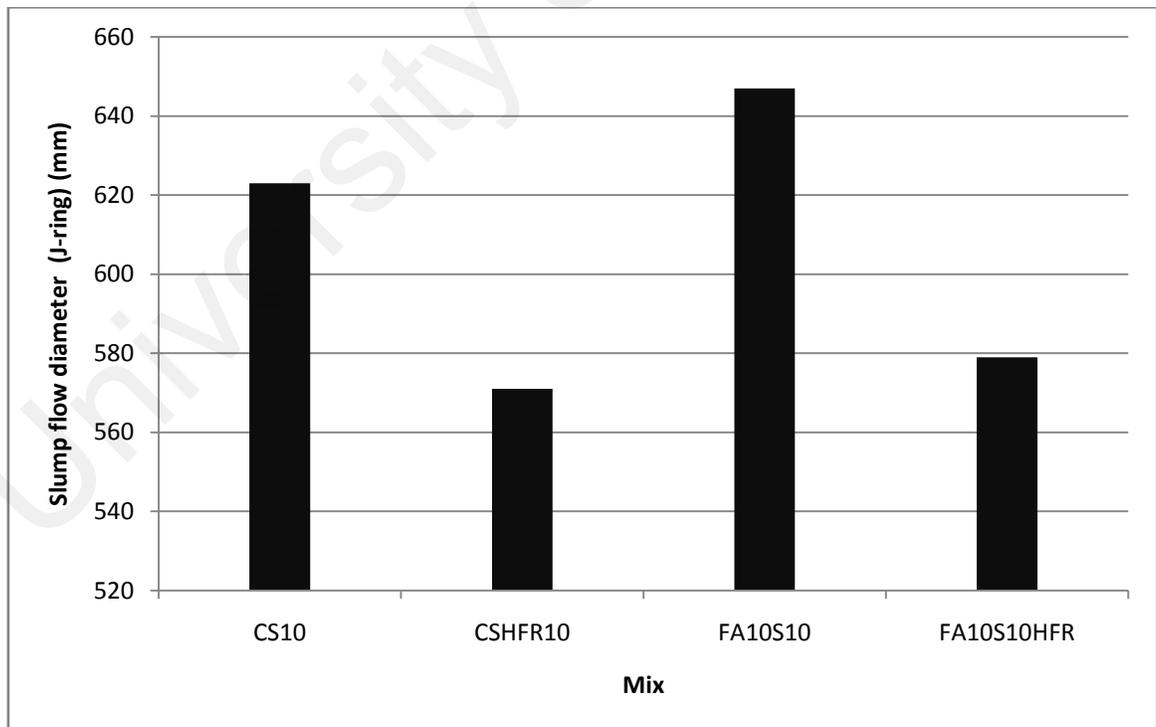
Figure 4.76: Slump flow diameter of J-ring of different shape aggregate concrete mixes
