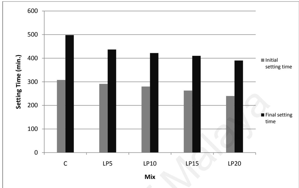
Figure 4.22: Initial and final setting time of LP mixes
