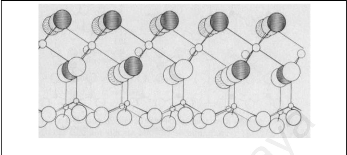
Figure 2.3: Perspective drawing of kaolinite with Si-O tetrahedrons on the bottom half and Al-O, OH octahedrons on the top half of the layer (Brinkley, 1958) cited by ( Justice, 2005)
