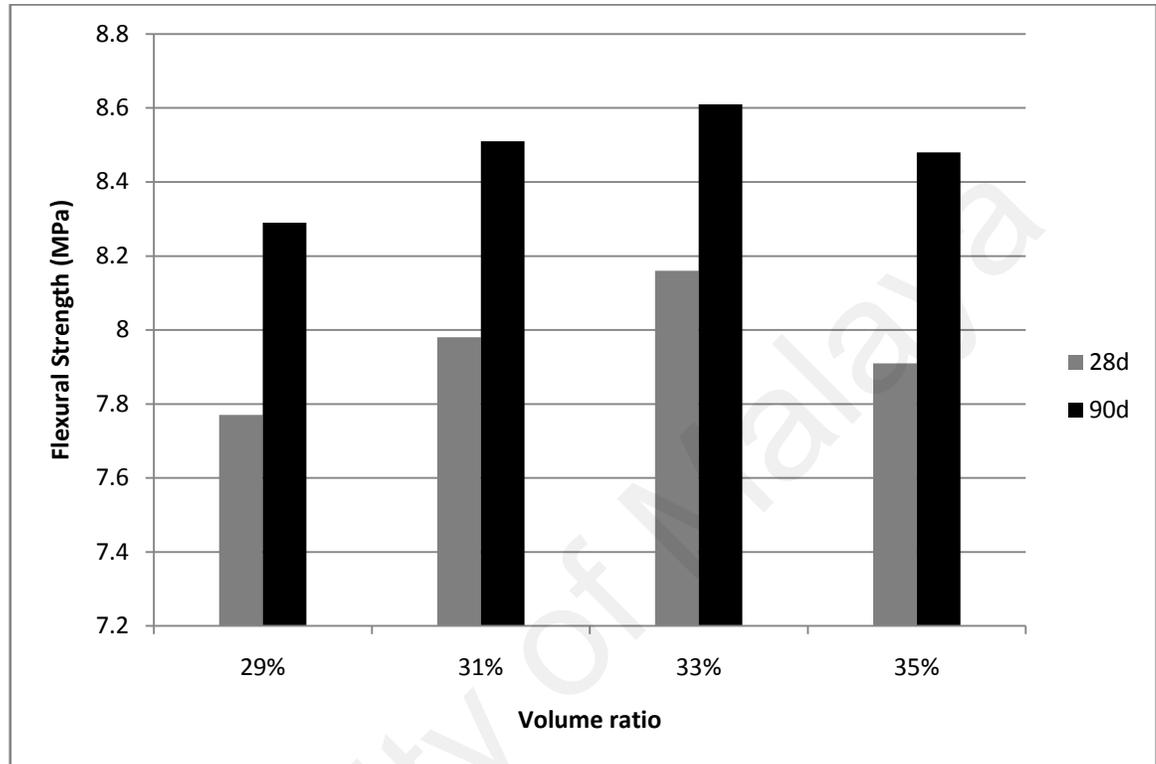
Figure 4.92: Flexural strength of different aggregate contents
