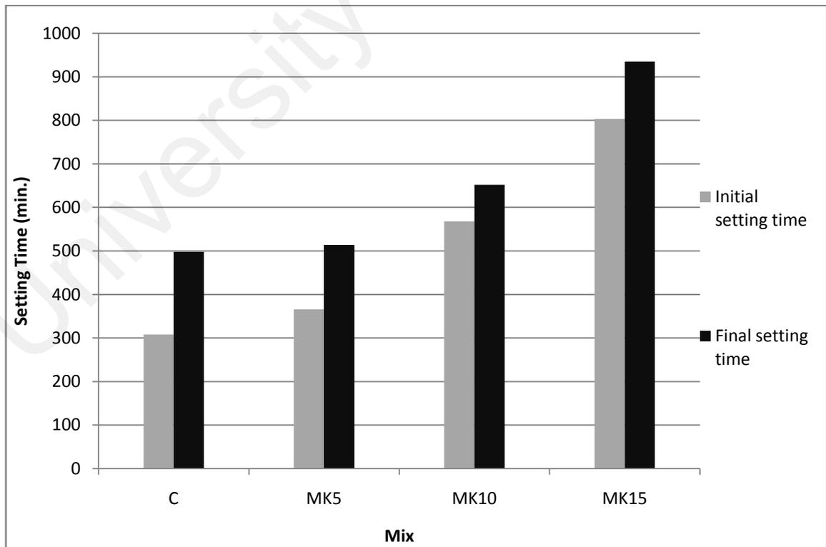
Figure 4.15: Initial and final setting time of control and metakaolin mixes
