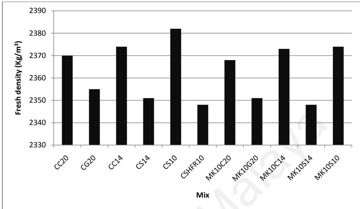
Figure 4.38: Fresh densities of metakaolin and control concrete mixes
