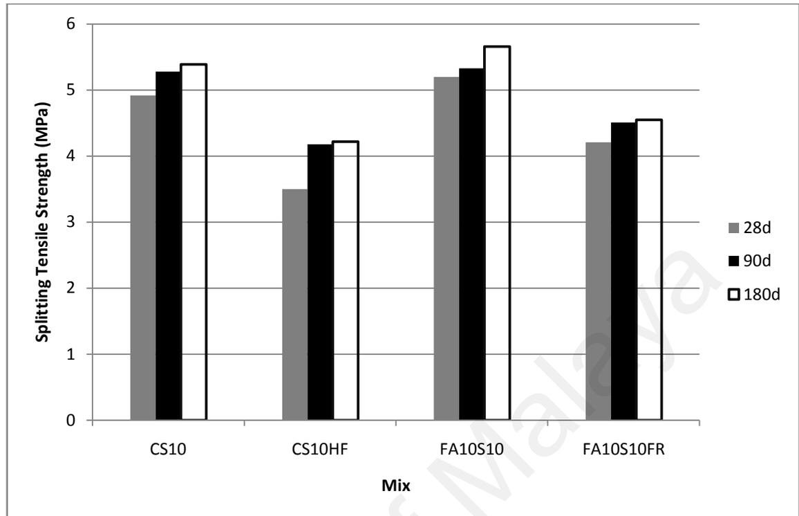
Figure 4.112: Splitting tensile strength of concretes with different shape aggregate
