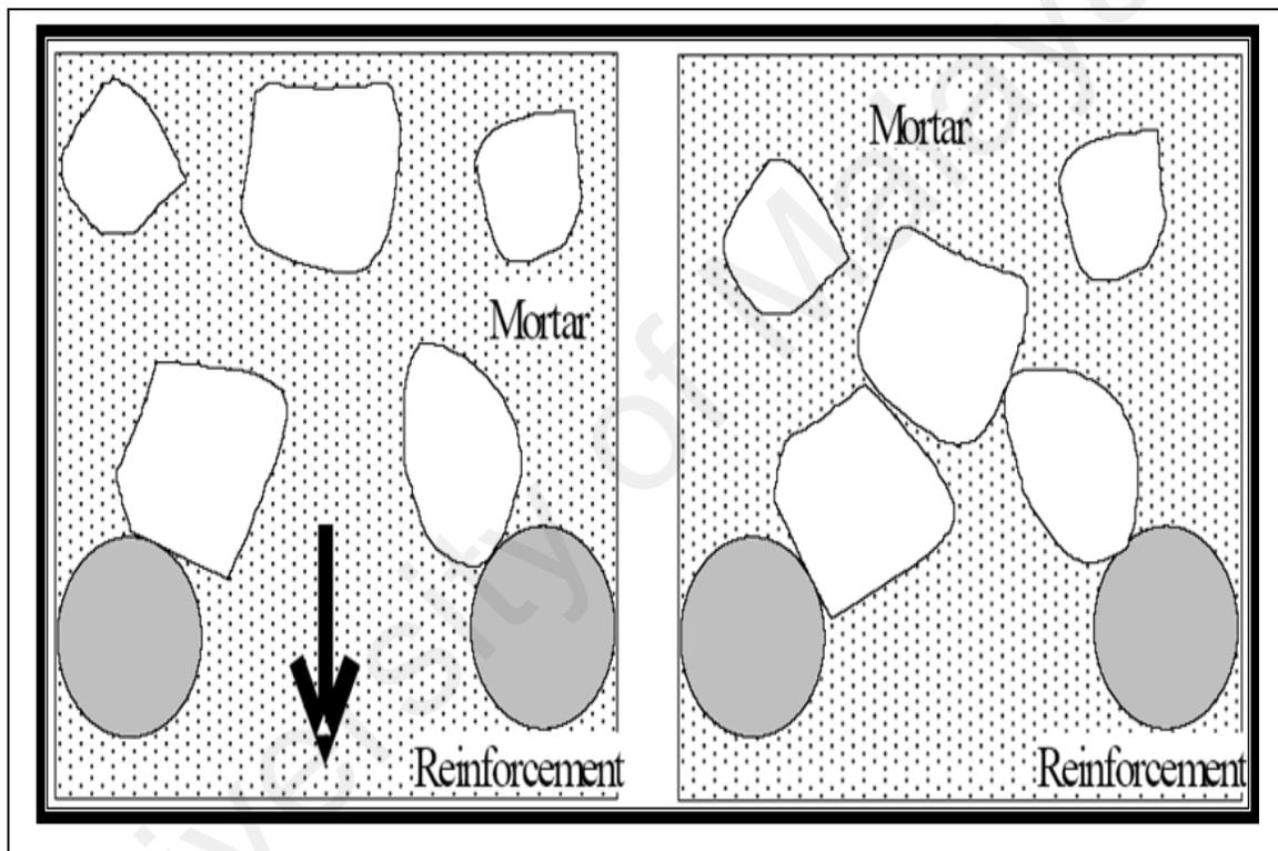
Figure 2.8: Arching phenomena during flow in congested area (EFNARC, 2002)
