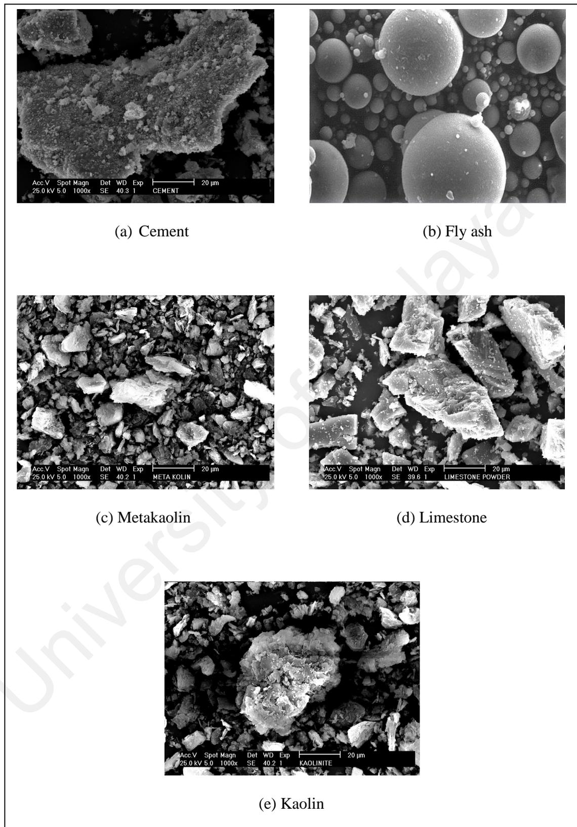
Figure 4.2: Micrographs of powders
