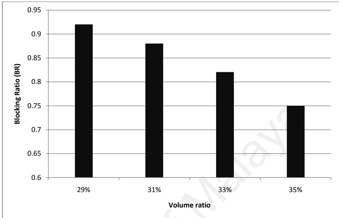
Figure 4.50: Blocking ratio of different coarse aggregate content
