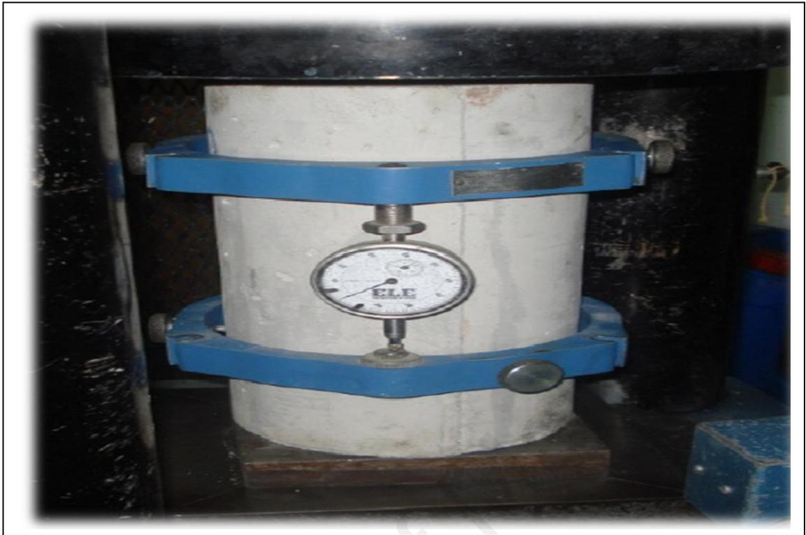
Figure 3.13: Set up of elastic modulus test
