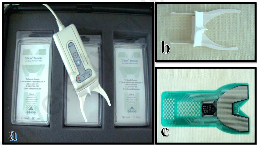
Figure 3.3: T-Scan III system, (a) handle, (b) supporting tray and (c) sensor.
