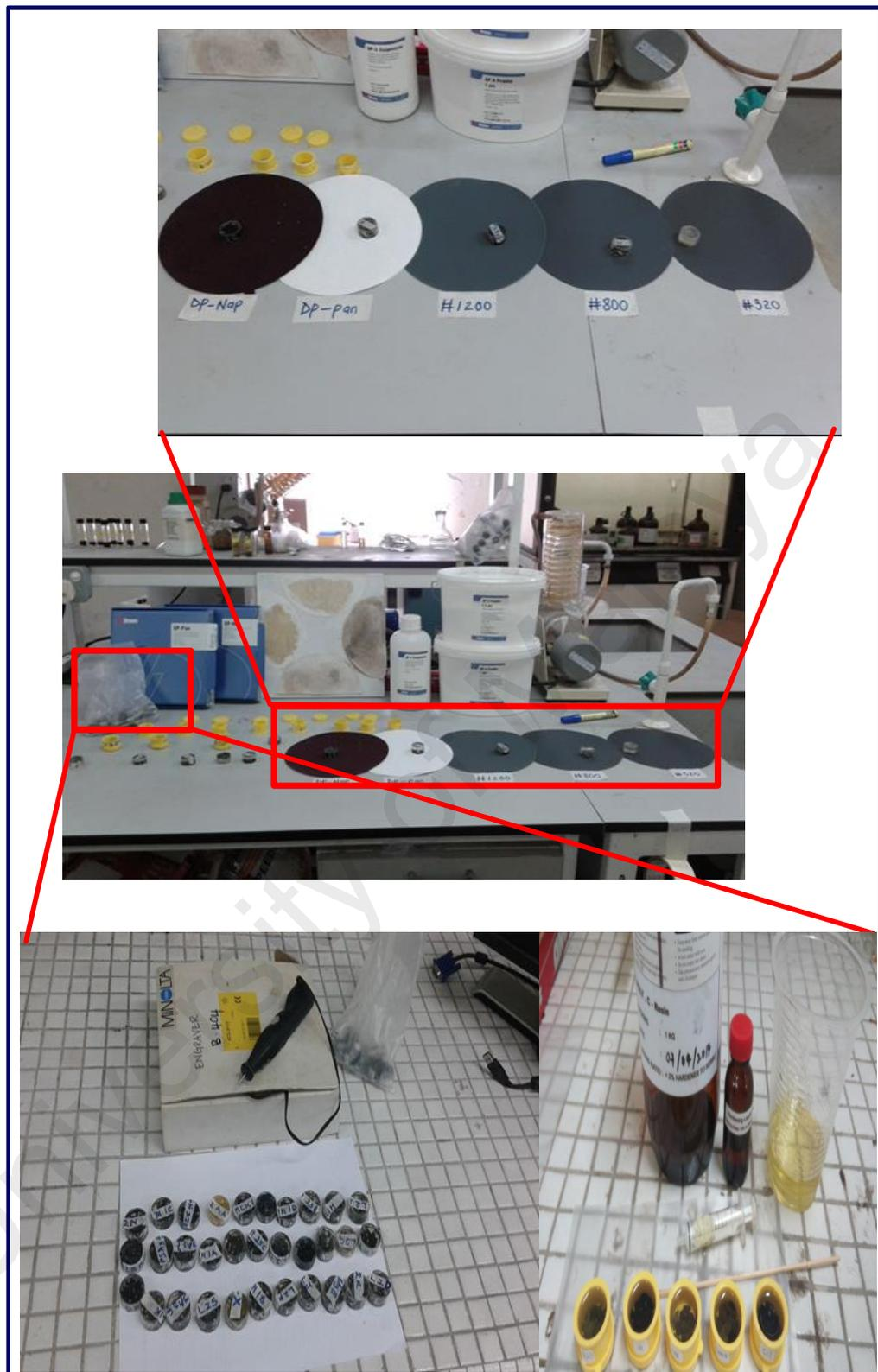
**Figure 3.11:** Polished blocks and materials used during the preparation.
