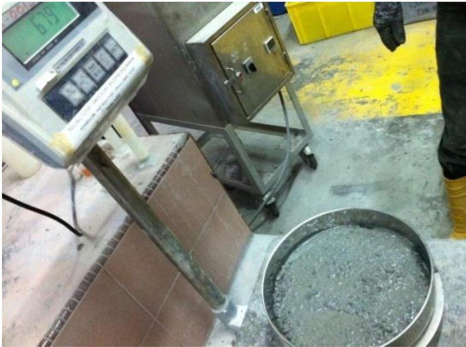
Figure 4.3.4 SCC tests - Segregation
