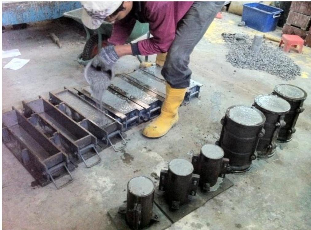
Figure 4.9 Samples for compressive strength, modulus of elasticity, tensile strength and flexural strength tests
