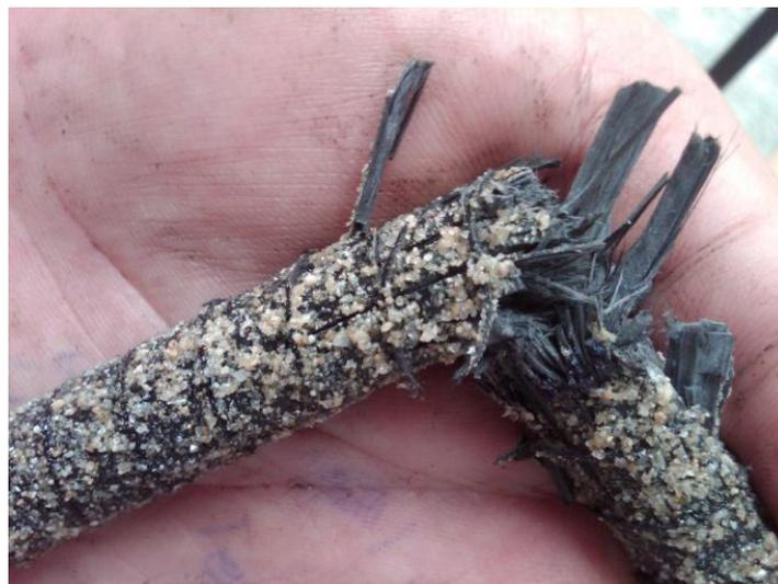
Figure 4.2 Failure of used CFRP-bars in different views
