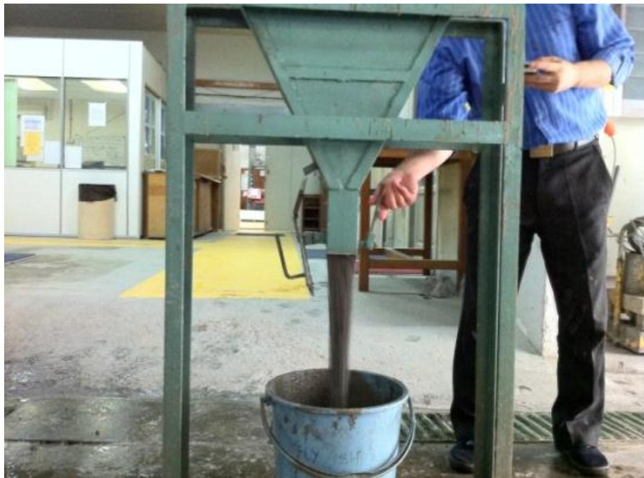
Figure 4.3.3 SCC tests - V Funnel
