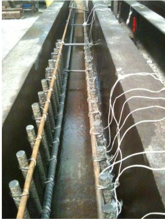
Figure 4.7.1 Group-II beams in moulds to cast -  $B_4S_{14}C_{12@10}$
