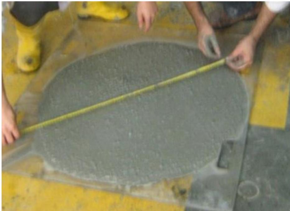
Figure 4.3.1 SCC tests - T50 & Dmax
