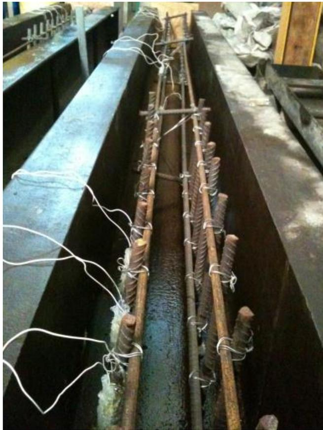
Figure 4.5.1 Group-I beams in moulds to cast -  $B_1S_{12}S_{12}@10$
