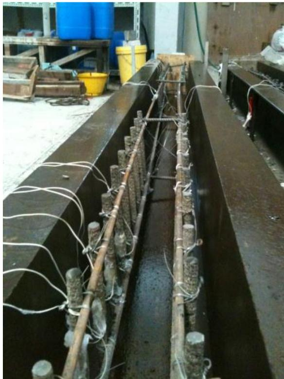
Figure 4.5.4 Group-I beams in moulds to cast  $-B_5S_{12}C_{12}@10$
