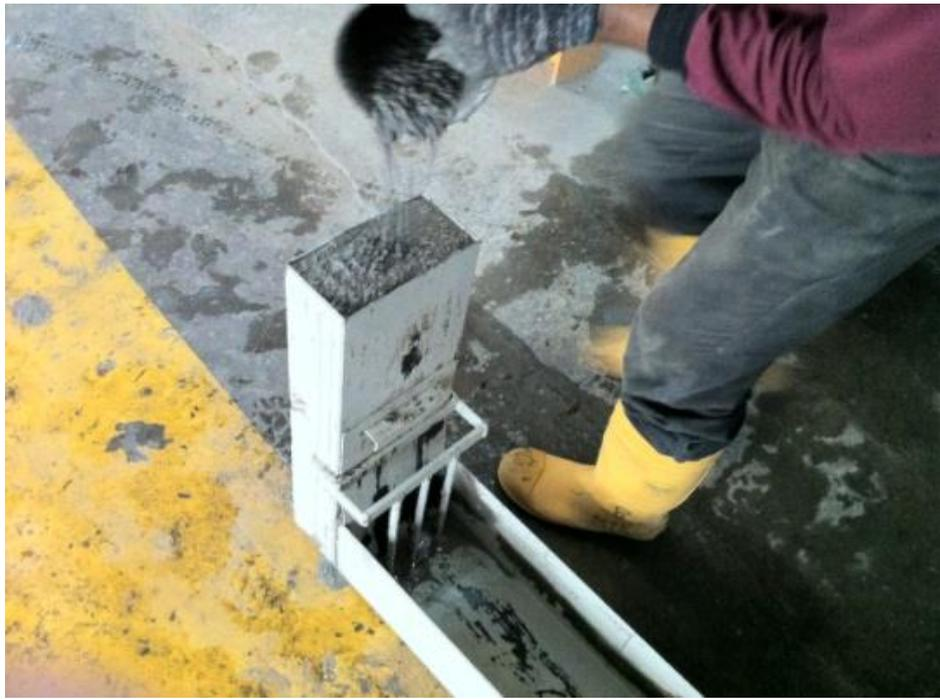
Figure 4.3.2 SCC tests - L Box
