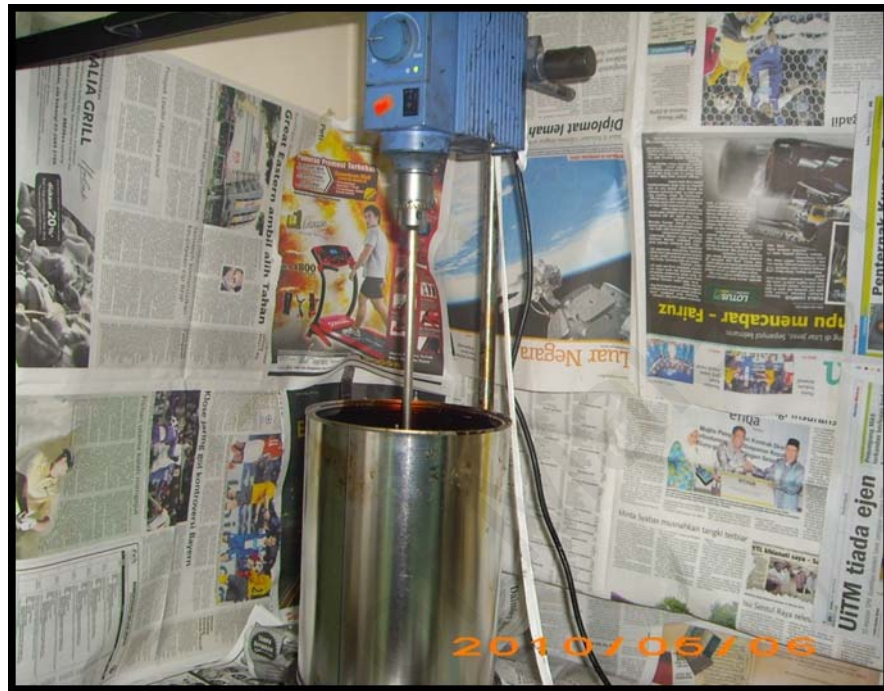
Figure 3.3: Propeller mixer used during the rubberised binder preparation
